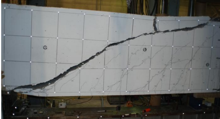
Figure 6-21: Overall Failure Crack on South Face of S1000-A4
