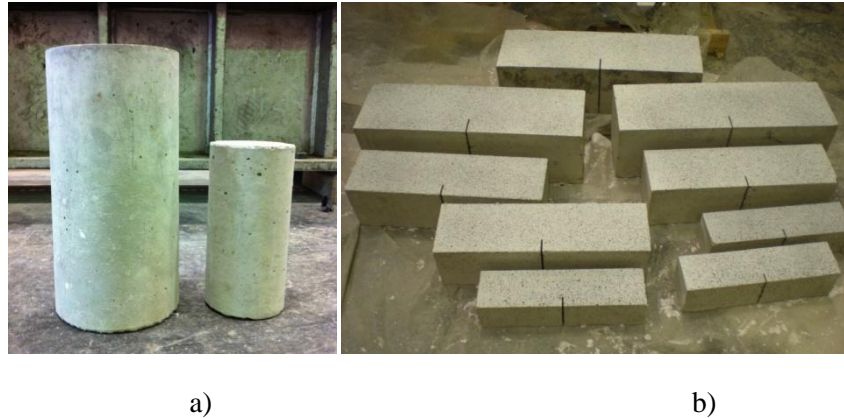
Figure 3-1: Production Mix Specimen Size Variation in a) Cylinders and b) Notched Prisms
