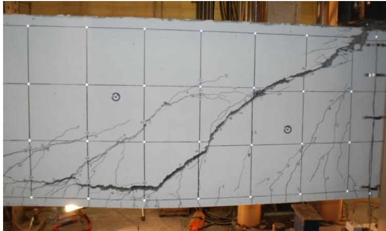
Figure 6-14: Overall Failure Crack on South Face of S1000-B2
