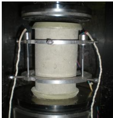
Figure 3-4: Compression Test Setup on a 100 mm Diameter Cylinder
