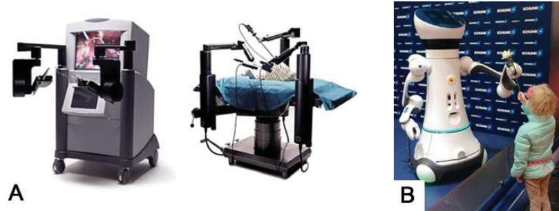
Figure 2.1: A. Zeus system used in trasatlantic surgery [1]. B. Fraunhofer Care-O-bot 4 service robot interacting with a human.
