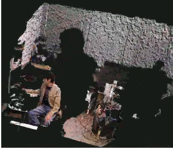
Figure 3.8: Both RGB and depth sensor are used to generate a point cloud visualization with color.
