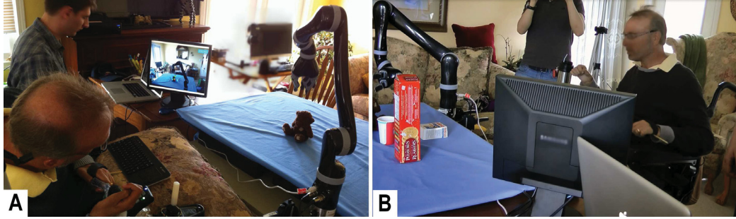
Figure 5.9: Set-up for our pilot study. For direct teleoperation, we adapted a joystick. For interacting with the visual interface, we integrated end-user’s regular PC mouse-pad. (A) Orientation task, (B) Drinking task.
