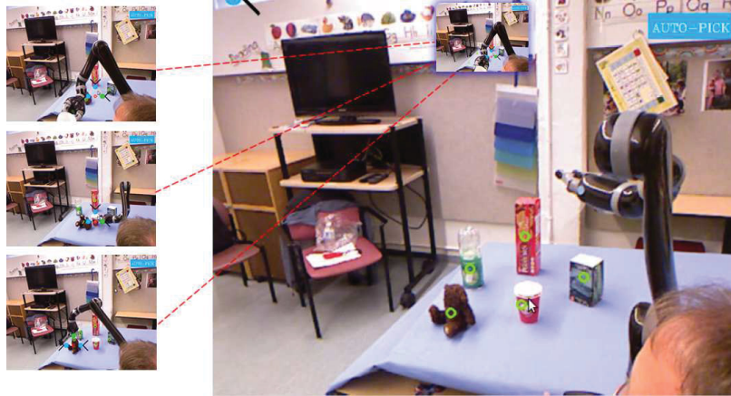
Figure 5.15: Interface preset mode. Left: three preset locations have been saved: (1) Near the user face to take a sip; (2) Picked location for the cup; (3) On top of the teddy bear. Right: The user can circle through the images of the preset list and display them as an inset on the main video window, then select the pre-set location he or she desires.
