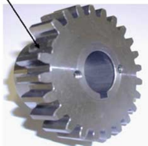
FIG. 9—The faulty gear missing a single tooth.
