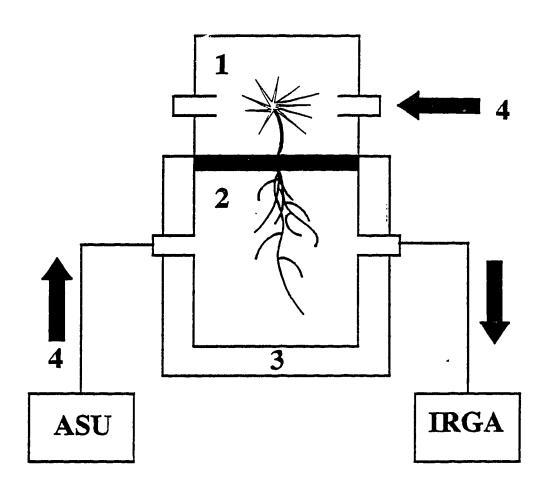
rate of 10 mL sec<sup>-1</sup>. Temperature was controlled by a water jacket around the cuvette connected to a Haake F3-C digital Refrigerated Bath and Circulator. Interior temperature of the cuvette was recorded using a thermocouple.
