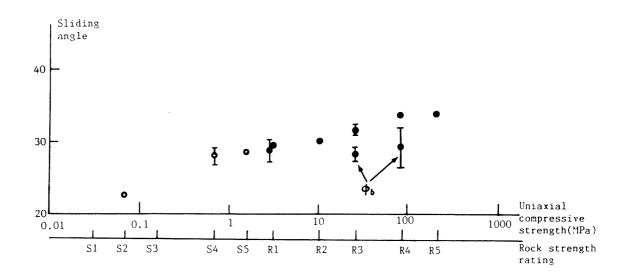
Figure 2. Relationship between strengths of rock blocks and sliding angles. S1 to S5 and R1 to R5 are strength ratings (Herget, 1977). The bars represent 95% confidence interval and the circles represent mean values of sliding angles. The open circles are shales and siltstones and the solid circles are sandstones.  $\phi_b$  is the basic friction angle.
