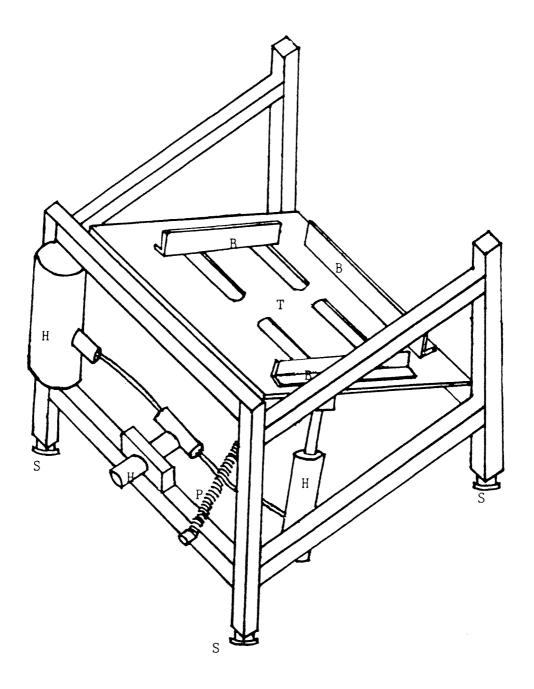
Figure 1. The portable tilting table. In the figure, T, B, H, S and P represent the tilting table, brackets, hydraulic system, adjustable screws and the spring.
