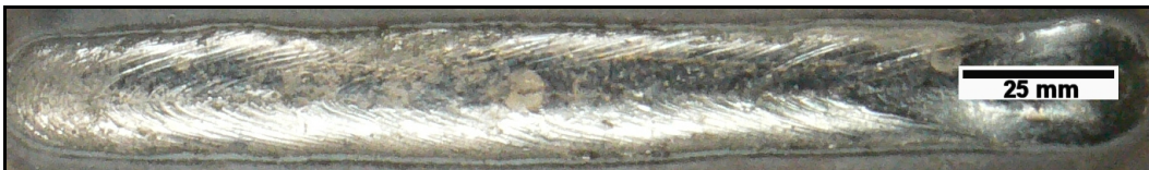
Figure 5-7: Weld Coupon 36 (Good Bead Width Consistency)
