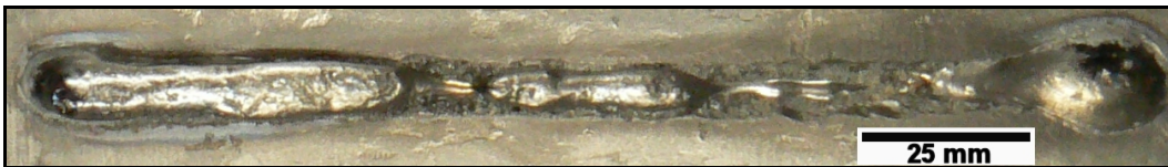
Figure 5-8: Weld Coupon 25 (Poor Bead Width Consistency)
