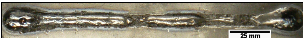
Figure 5-9: Weld Coupon 33 (Poor Bead Width Consistency)
