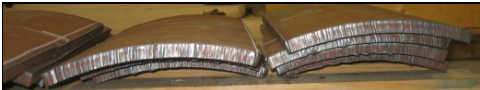
Figure 3-2: Cut Weld Coupons, Illustrating Curved 250 mm (10”) Sides
