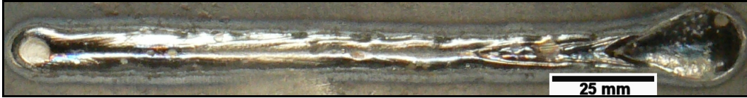
Figure 5-11: Weld Coupon 7 (Intermediate Bead Width Consistency)
