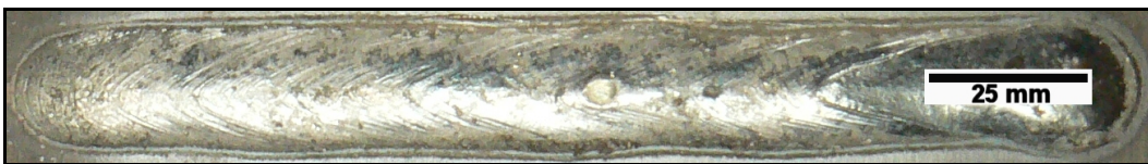
Figure 5-6: Weld Coupon 35 (Good Bead Width Consistency)
