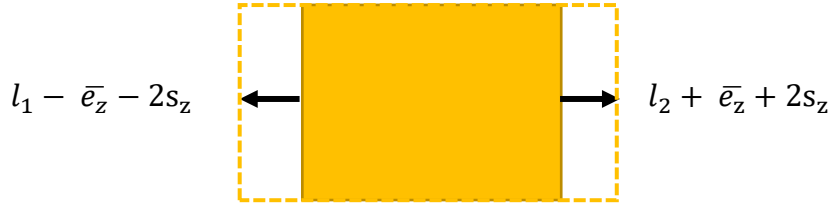
Figure 3.10: Error tolerance in z to account for the calibration error
