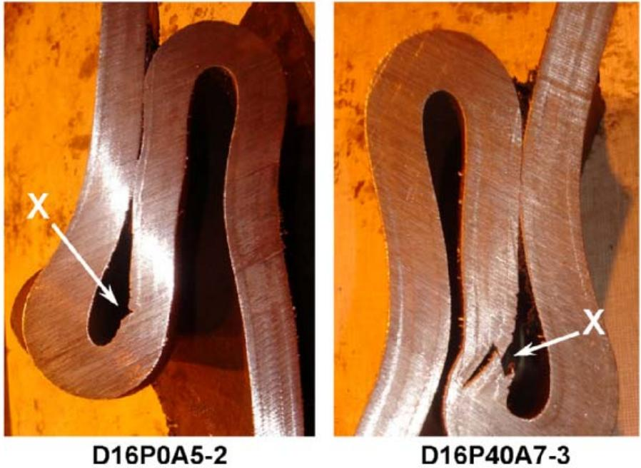
Figure 4.20 Cut segment from the compression side of Specimen 2 and 3
