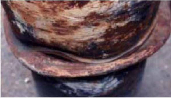
Figure 3.2 Pipe segment showing tearing fracture at wrinkle location obtained from WestCoast Energy (Das et al. 2002)
