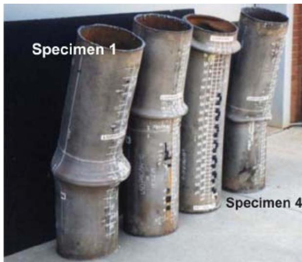
Figure 2.8 Non-axisymmetric wrinkles under bending deformation (Das et al. 2008)
