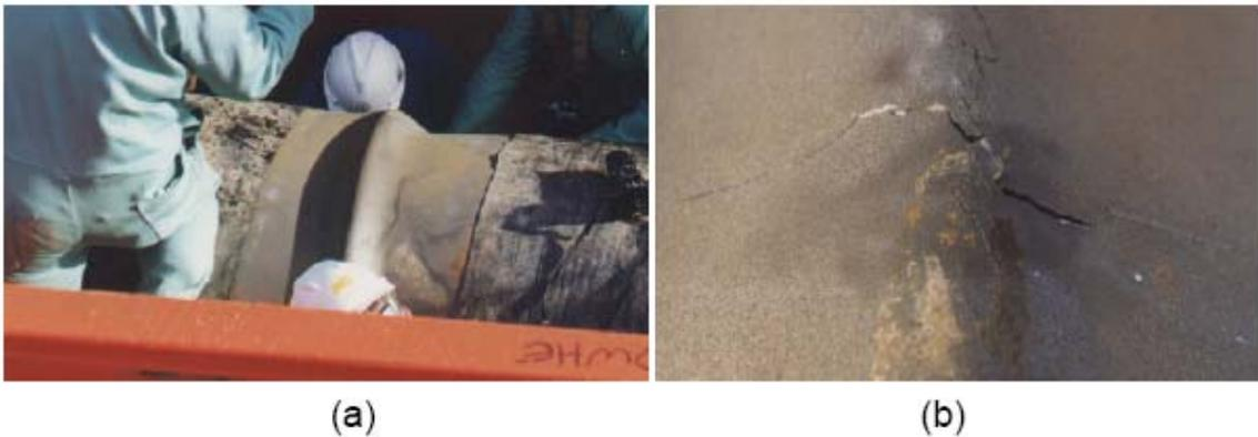
Figure 2.4 (a) Wrinkle (buckle) in a 40 inch diameter steel pipe with (b) close-up view of wrinkled pipe showing through-the-wall cracks (NTSB 1999)
