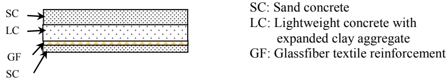
Figure 5.1- Cross-section configuration of prototype panel
