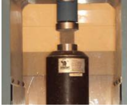
(a) Cube test setup
