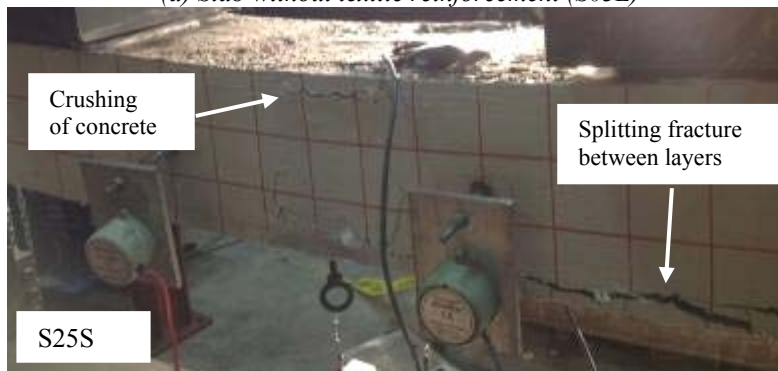
(b) Slab with textile reinforcement (S25S)
