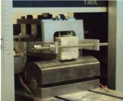
(c) Prism test setup
