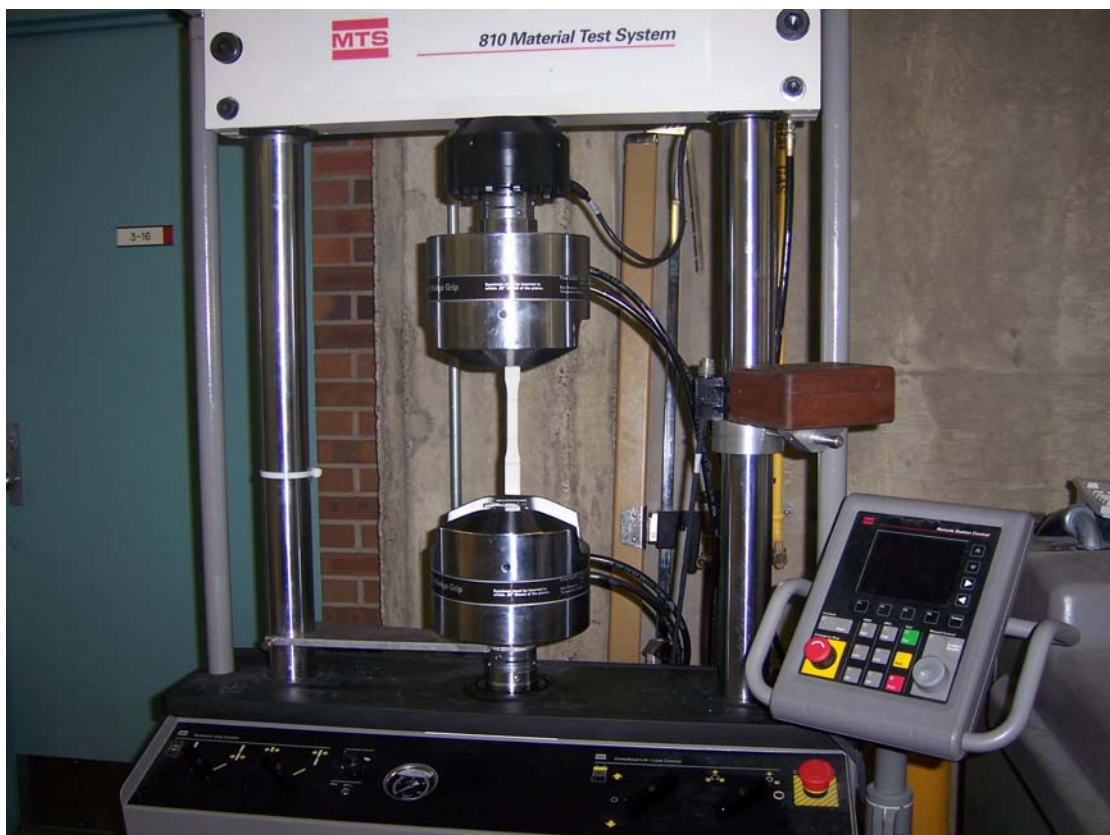
Fig. 3.3 MTS material testing system and tensile test setup
