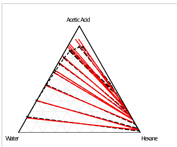
Figure B.3 Huron—Vidal Peng—Robinson calculation of LLE for water—acetic acid—hexane using optimized parameters; default parameters failed to predict LLE. Calculated values are solid lines, experimental values are dashed lines. (1)
