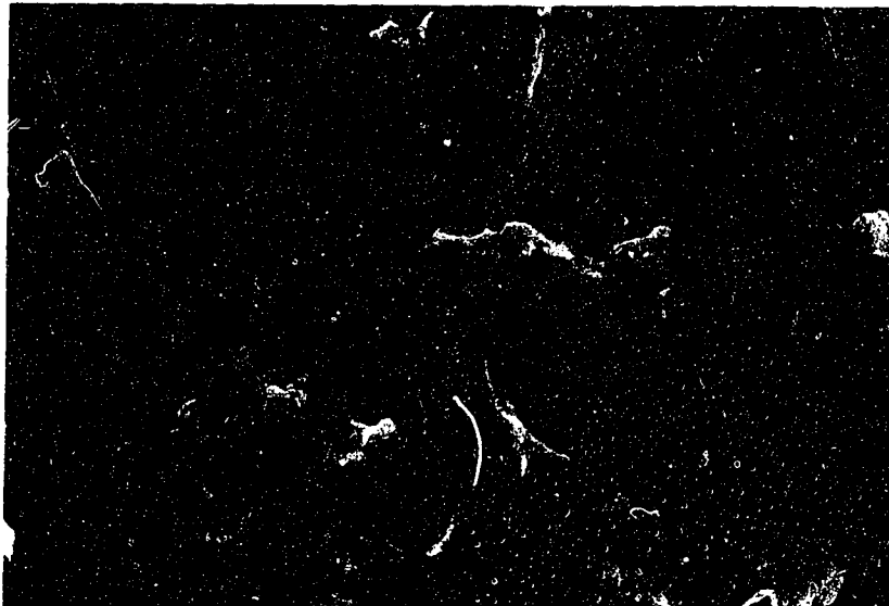
Figure 4.29: Sample SW1 - 40% cold worked, 147 ppm hydrogen, final test done on sample, testing done at 265°C. SEM photograph taken looking down on the fracture surface (radial/axial plane). Few, if any lengthwise cracks visible. Cracking direction is from top to bottom. 6,000X.
