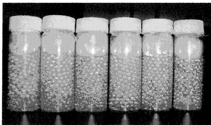
**Figure 4.11: PHCs collected during SC CO<sub>2</sub> extraction**
