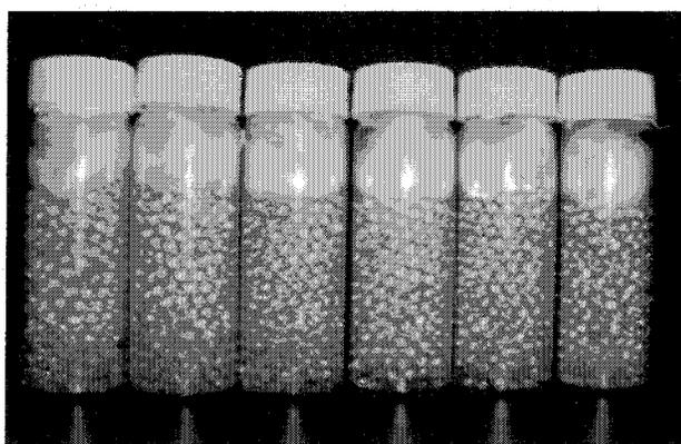
**Figure 3.6: Hydrocarbons collected every 5-minutes during dynamic extraction**
