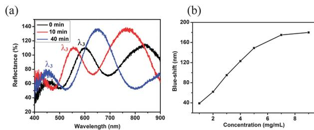
**Fig. 2** (a) Reflectance spectra of etalon after exposure to triolein ( $9 \text{ mg mL}^{-1}$ ) at 30 °C after the indicated times; (b)  $\lambda_3$  blue-shift as function of triglyceride concentration.
