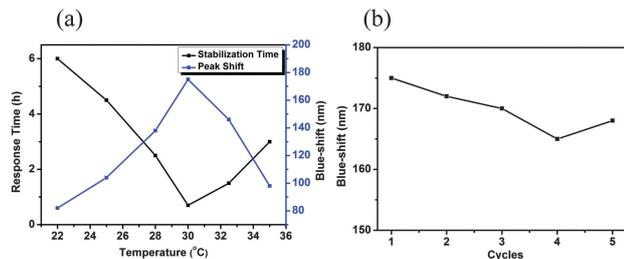
Fig. 3 (a) Response time and  $\lambda_3$  blue-shift as function of temperature; (b)  $\lambda_3$  blue-shift as function of the number of times used.
