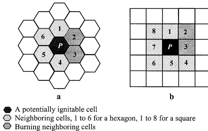
Figure 3.2. Depiction of the principle of fire spread.
