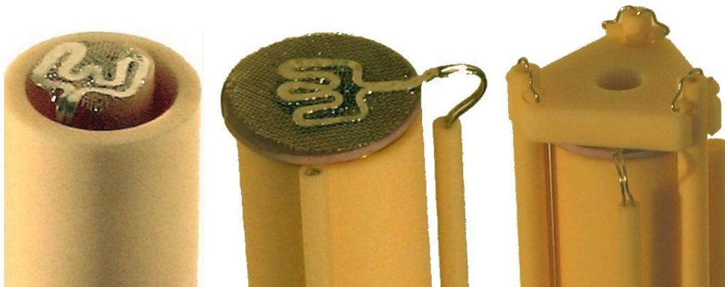
Figure 3.1 Schematic of conductivity test by the two-points method. Left: the bottom electrode pushed up by the inner gas supply tube. Middle: sample, thermocouple and top electrode. Right: spring load assembly pulling the setup tightly together.
