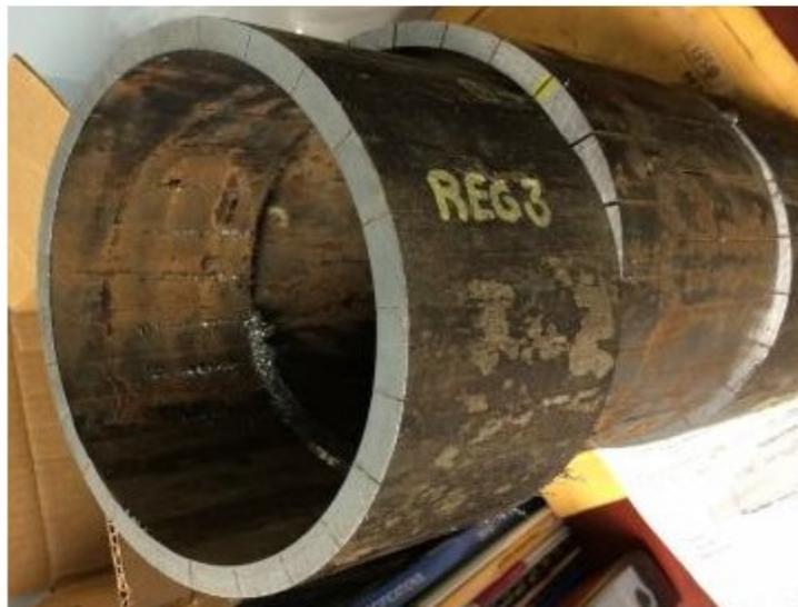
Figure 1-3. A failed section of slotted liner with considerable amount of corrosion stains [5].
