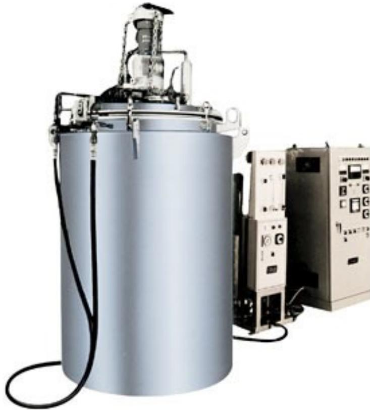
Figure 2-9. The industrial-scale “pot-type” gas nitriding furnace [38].
