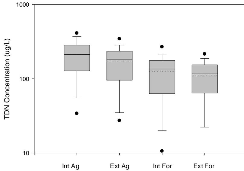
Figure 3-4 Proportion of total nitrogen in the dissolved form in the agricultural (extensive and intensive) and forestry (extensive and intensive) catchments.
