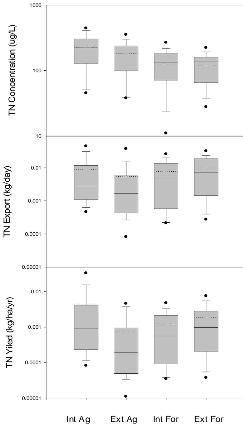
Figure 3-3 Total dissolved nitrogen concentration ( $\mu\text{g/L}$ ) in the agricultural (extensive and intensive) and forested (extensive and intensive) catchments.
