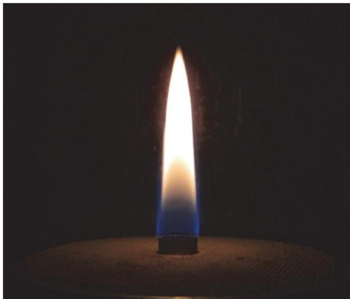
Figure 2.4. Laminar co-flow methane diffusion flame used in this study
