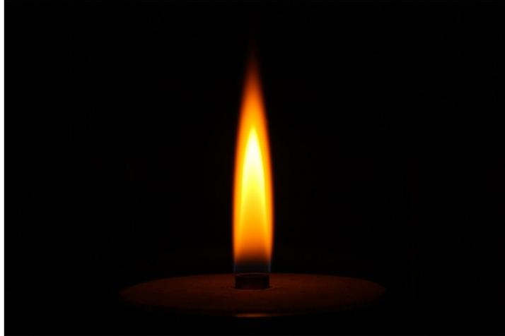
Figure 2.10. Laminar co-flow methane diffusion flame with NaCl additive.
