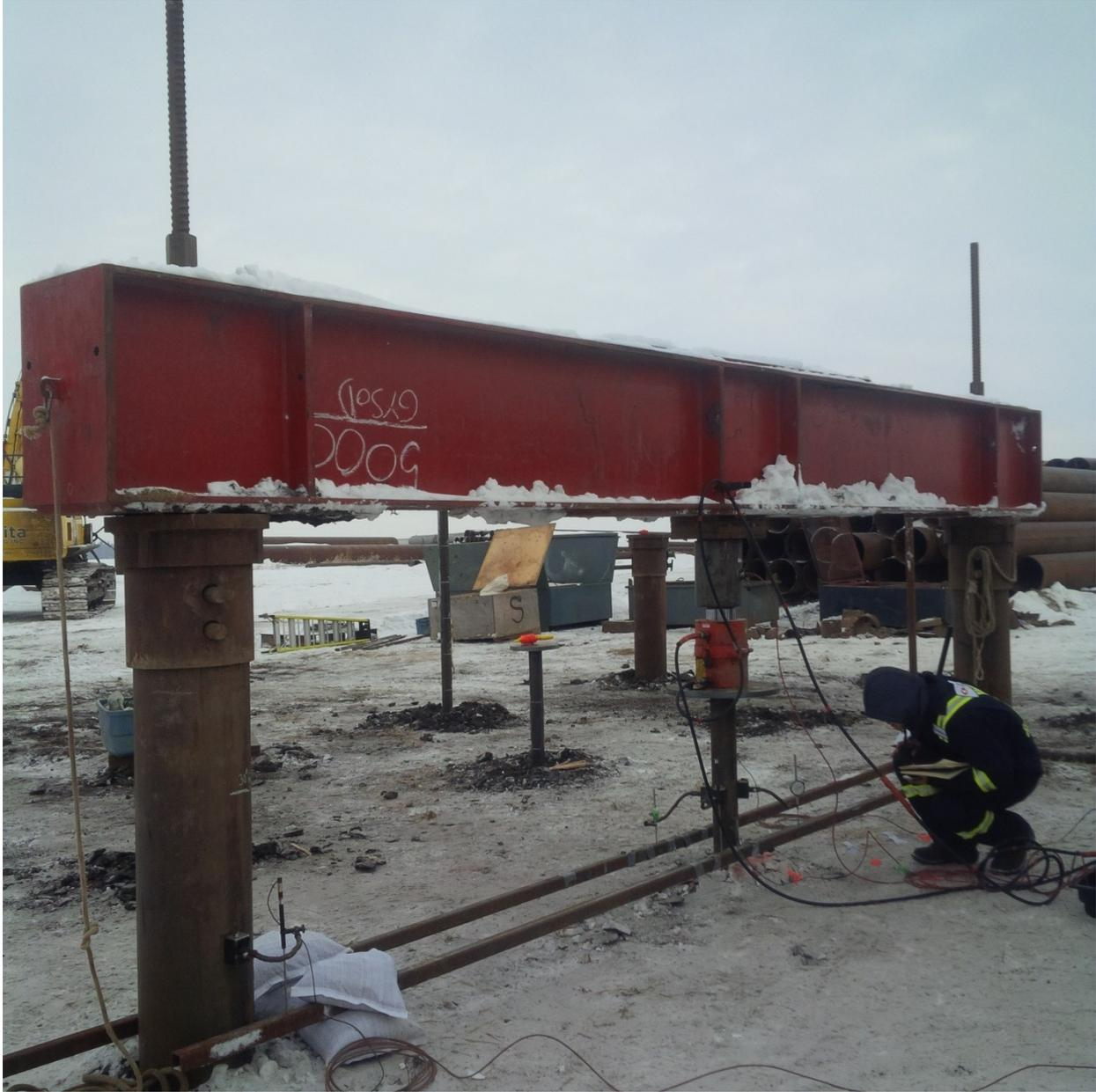
Figure 3-9: Setup of axial compression tests
