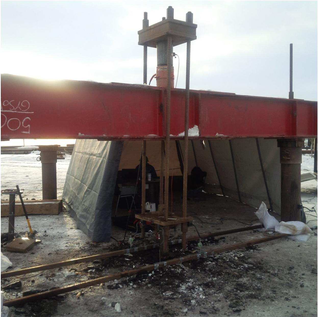
Figure 3-10: Setup of axial tension tests
