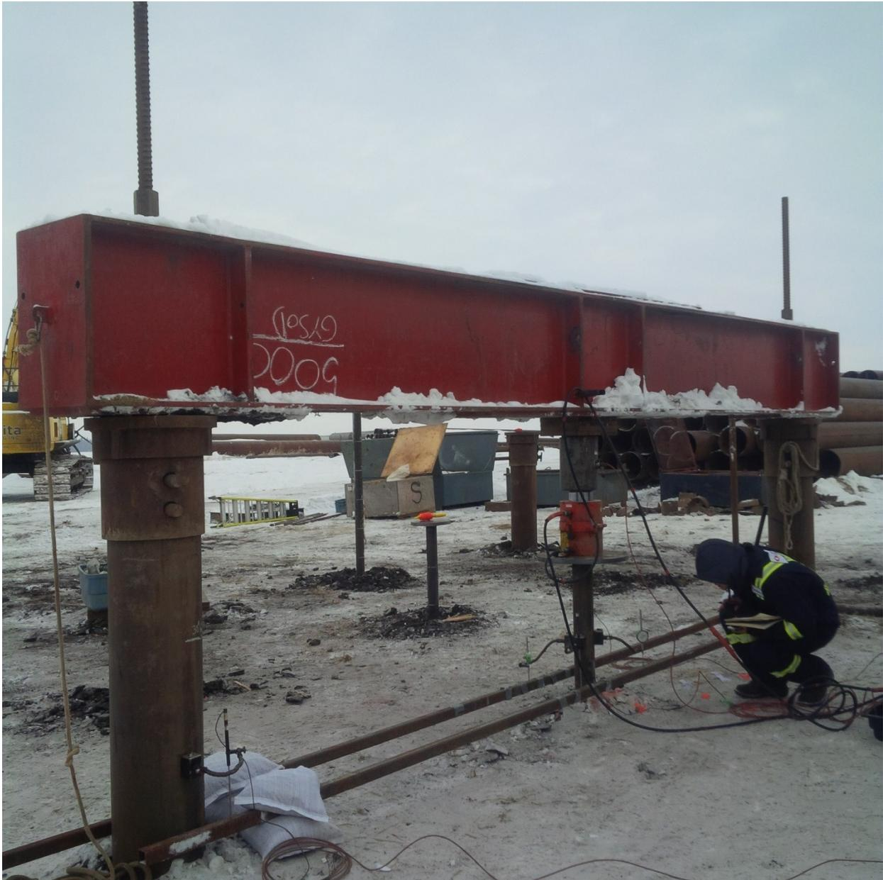
Figure 3-9: Setup of axial compression tests
