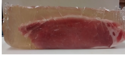
Figure 3.6: The ex-vivo tissue sample consisting of porcine loin muscle tissue embedded in gelatin.
