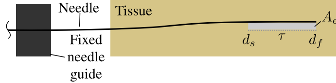
Figure 7.1: The considered control objective commonly occurring during prostate brachytherapy, which is to minimize the area A_e under the line segment \tau .
