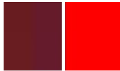
Figure 3.2: The intensity of a red pixel in the right image (projected pattern) is (255, 0, 0) , while in the left image (captured image) is (104, 23, 17) . These two pixels are representing two corresponding pixels, one on the projected image by the projector and the other on the captured image by the camera. These two corresponding pixels are supposed to have the same intensities but it does not happen in practice.
