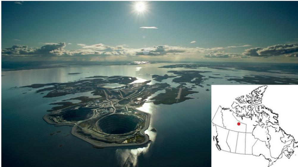
**Figure 3.1:** DDMI mine site is located 320 km northeast of Yellowknife, NWT in the Barrenlands region. The two open pits located in the image foreground were constructed over the Lac de Gras lake bed through the installation of dyke systems to allow for de-watering. The mine footprint caused extensive fish habitat loss, triggering habitat compensation projects to help offset environmental impacts. Photo courtesy Diavik Diamond Mines, Inc.
