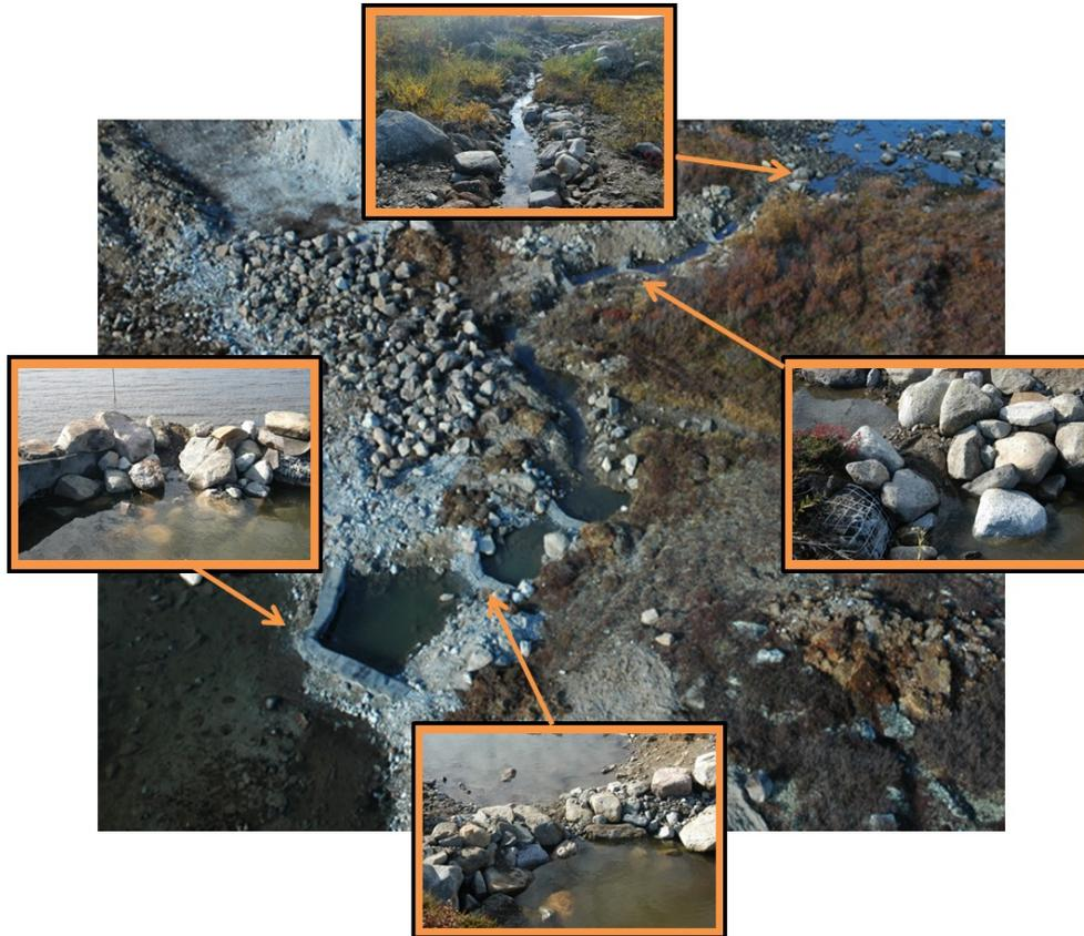
**Figure 2.4:** Aerial photo of M1S with original gabion structures. Overlaid images depict the location and details of various retrofitted structures including weir one (left), weir two (bottom), weir five (right), and the channelized M1S-LDG connection (top). Aerial photo courtesy of Praetorian Construction Management.
