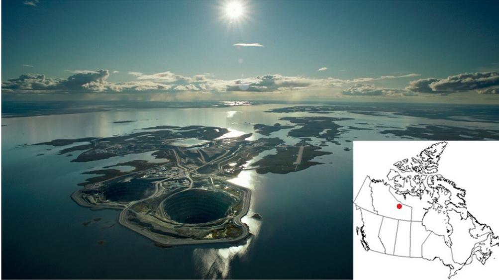
**Figure 2.1:** DDMI mine site is located 320 km northeast of Yellowknife, NWT in the Barrenlands region. The two open pits located in the image foreground were constructed over the Lac de Gras lake bed through the installation of dyke systems to allow for de-watering. The mine footprint caused extensive fish habitat loss, triggering habitat compensation projects to help offset environmental impacts. Photo courtesy Diavik Diamond Mines, Inc.
