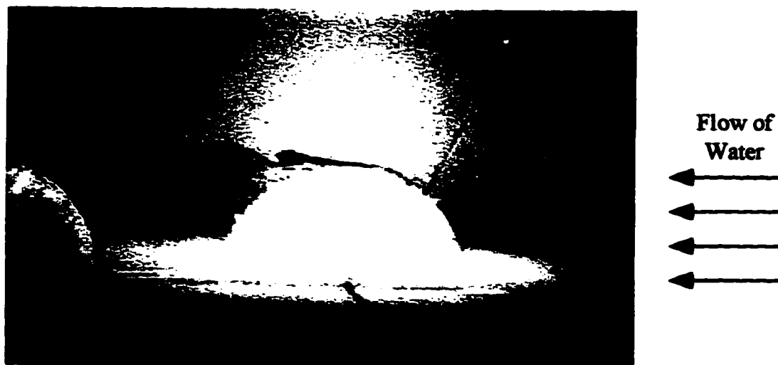
Figure 4.23 Arch vortex shedding from LE when S/S' \geq 1.7/1.8
