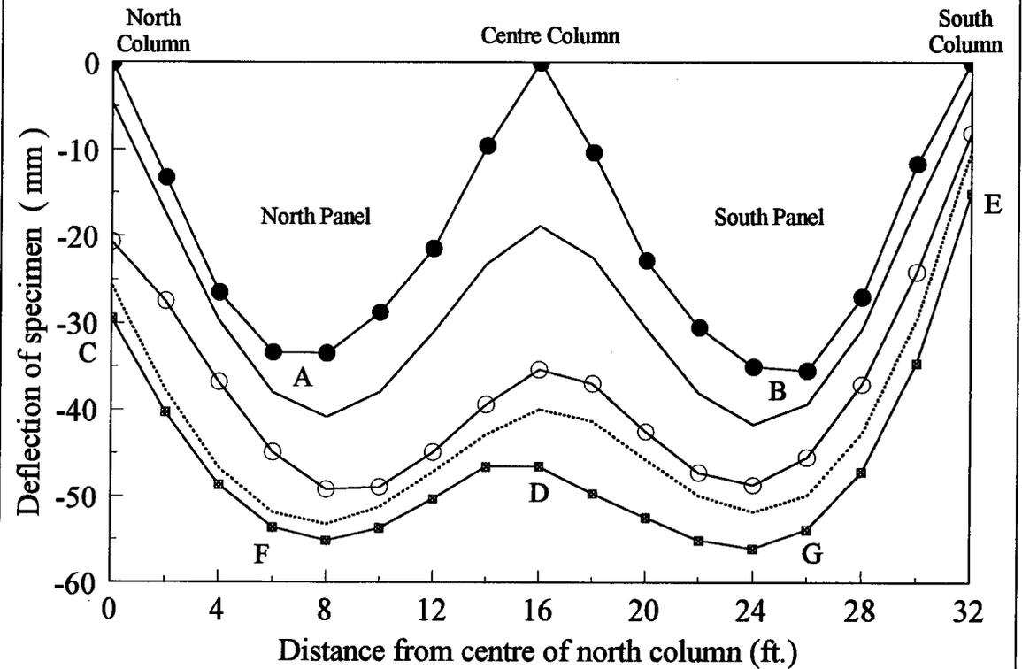
(b) Right before punching of interior connection,  $q = 17.1$  kPa
