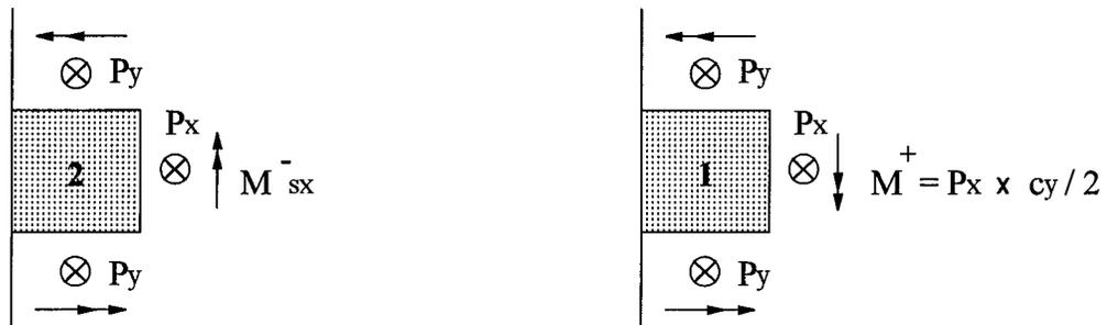
$P_y = \text{Shear capacity of spandrel strip}$
