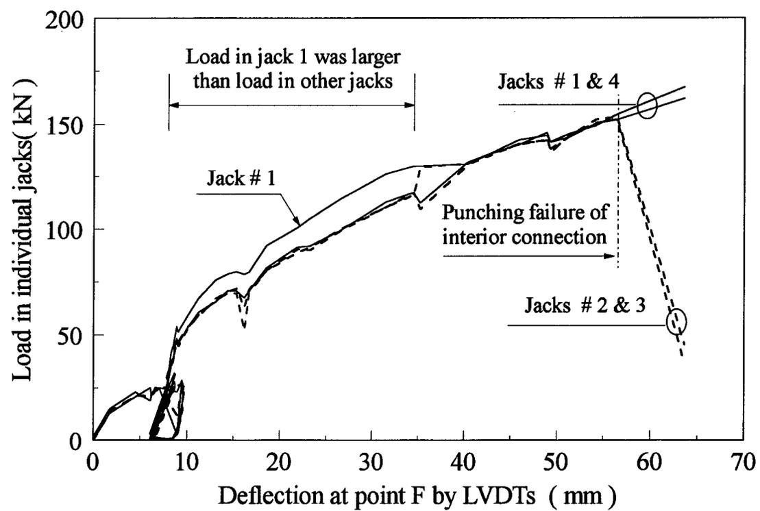
Figure 4.5 Load in jacks versus deflection of specimen
