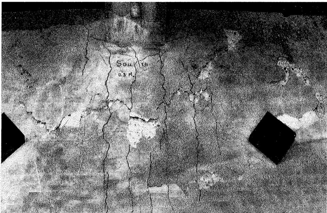
Figure 4.40 Punching of south connection
