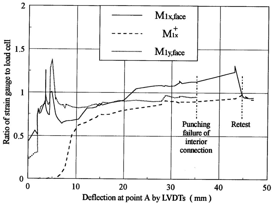
Figure 4.20 Comparison of the external measurements with the internal measurements in the north connection
