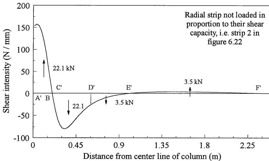
Figure 6.32 Idealized torsional shear intensity diagram along side faces of interior radial strips, case b
