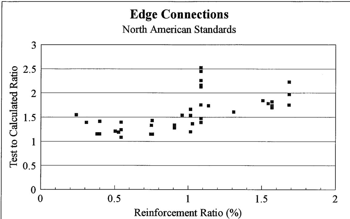
Figure 8.11 Test to calculated ratios of the edge connections reported in the literature versus the reinforcement ratio of the top bars in the interior radial strip
