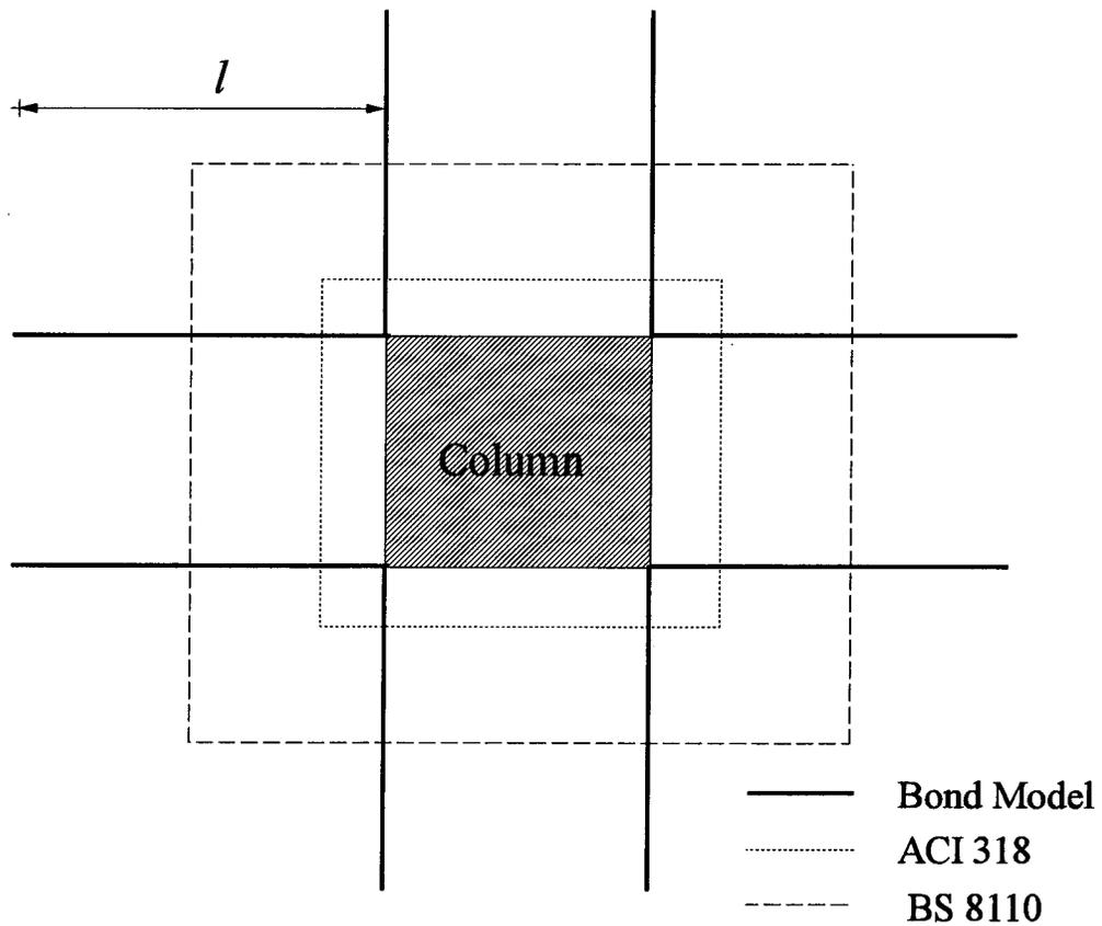
Figure 2.10 Bond Model Critical Section
