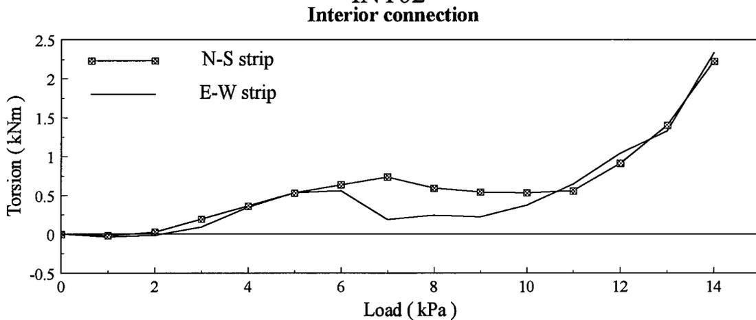
Figure 6.10 Torsional moment along each side face of radial strips, slab INT02
