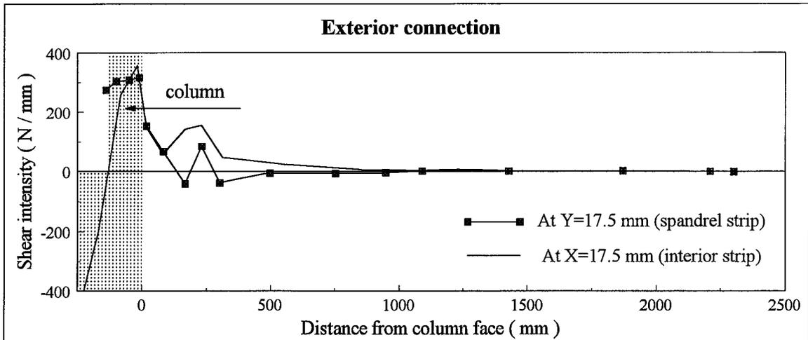
Figure 6.14 Shear intensity at a load of 10 kPa, slab EXT01
