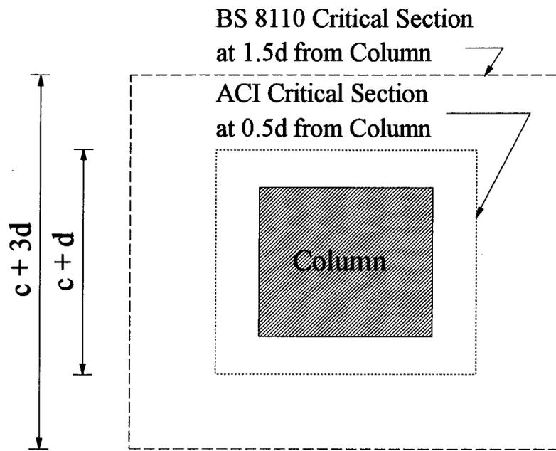
Figure 2.9 Code-defined Critical Sections
