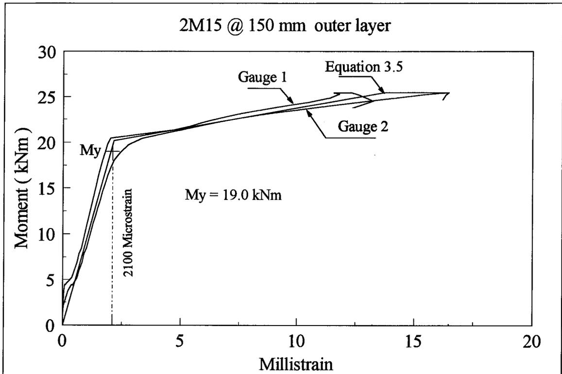
Figure 3.25 Moment-Strain Relationship for Beam 1
