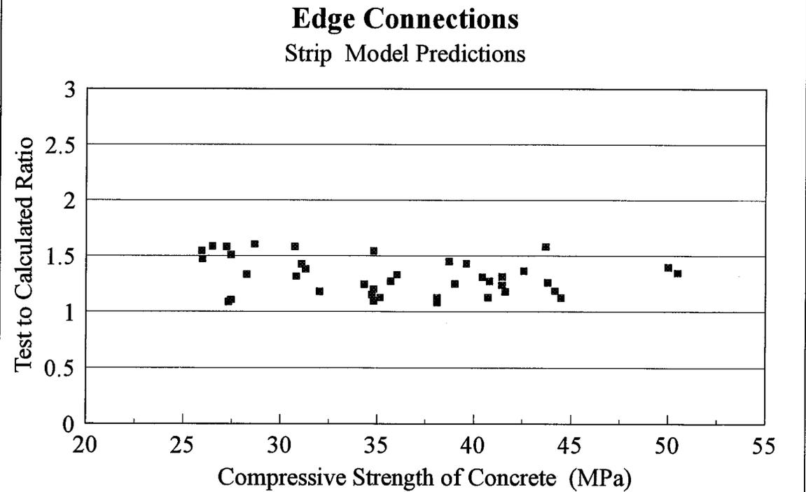
Figure 8.3 Test to calculated ratios of edge connections reported in the literature versus the compressive strength of the concrete,  $f_c$
