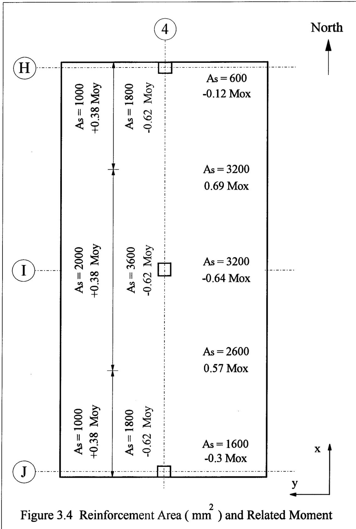
Figure 3.4 Reinforcement Area ( $\text{mm}^2$ ) and Related Moment
