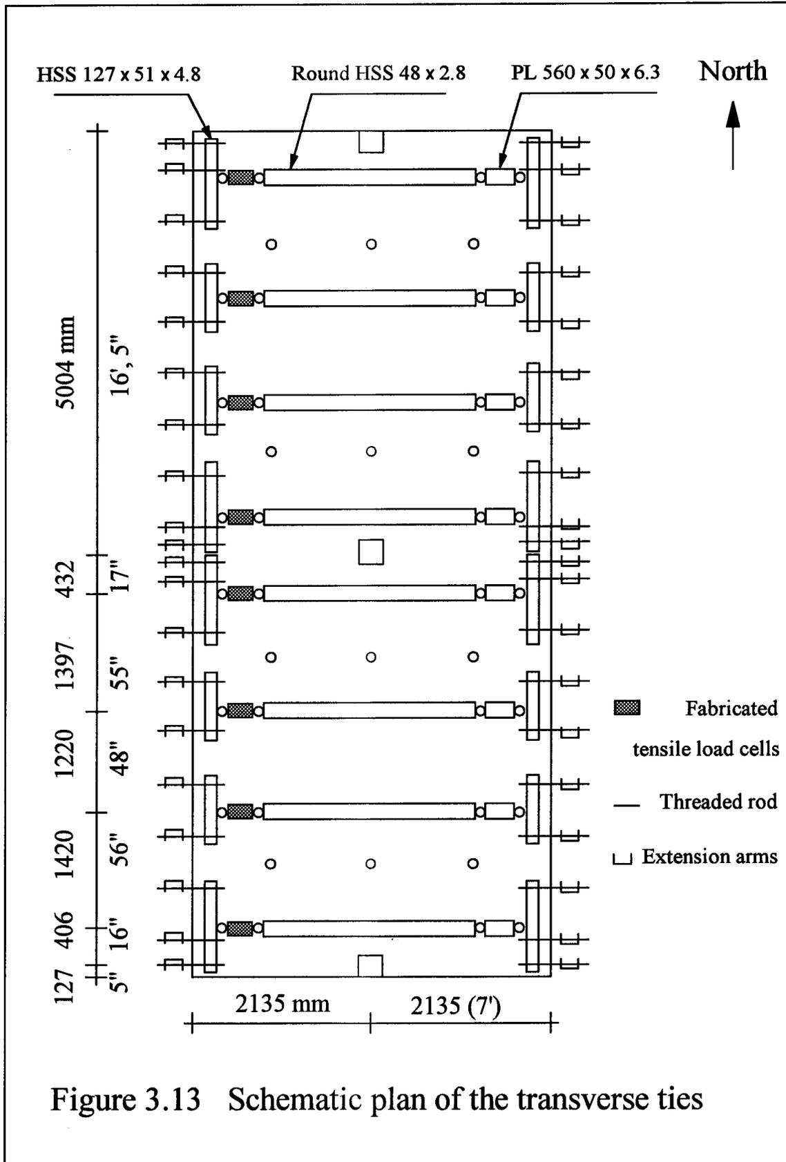
Figure 3.13 Schematic plan of the transverse ties
