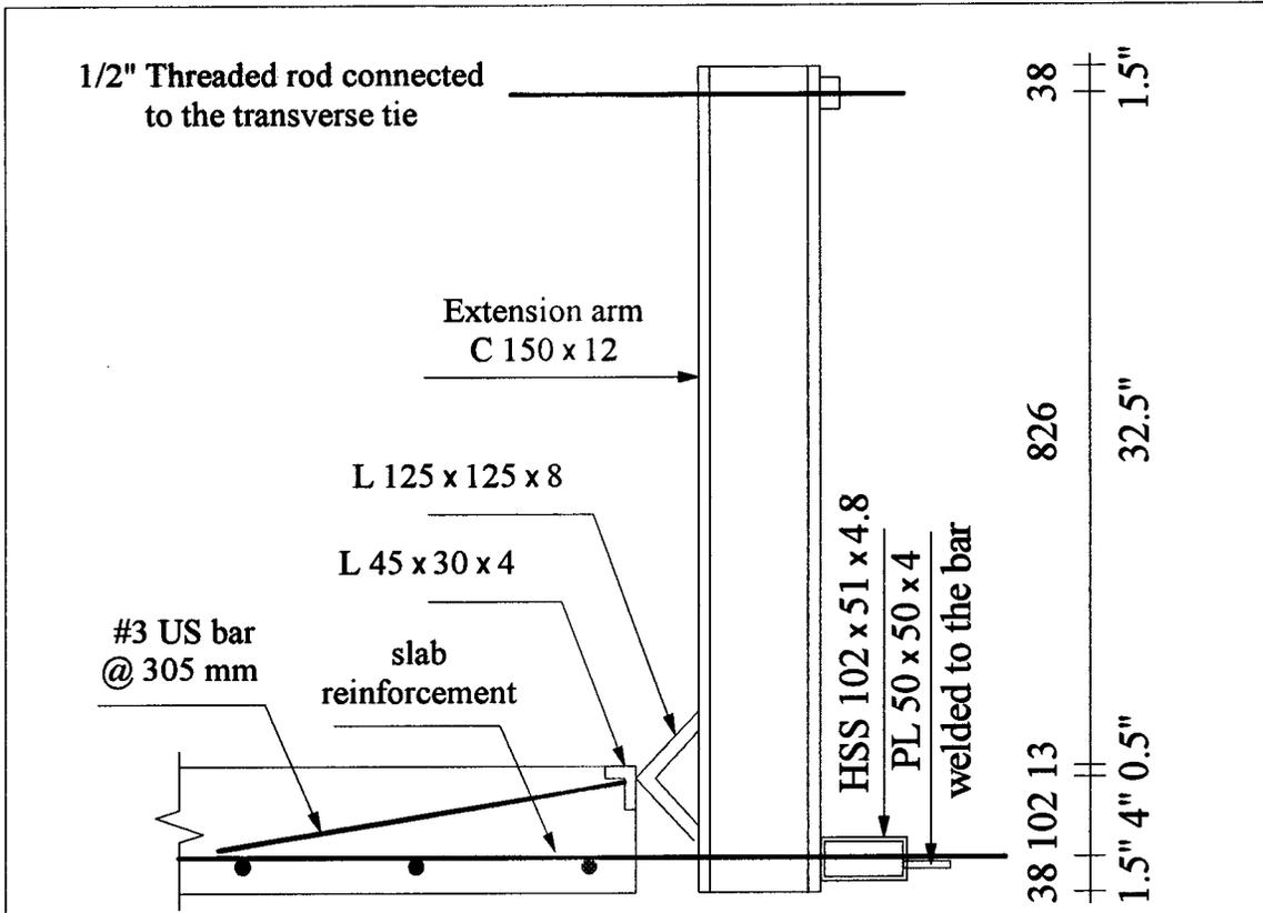
Figure 3.14 Restraint Details for continuous edge
