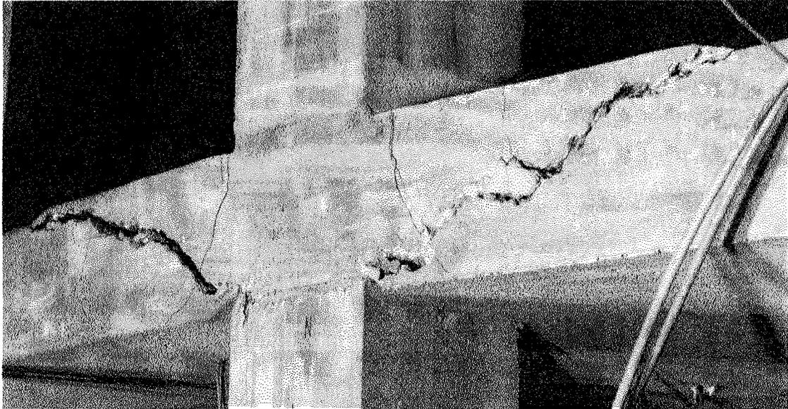
Figure 4.41 Side view of punching of north connection
