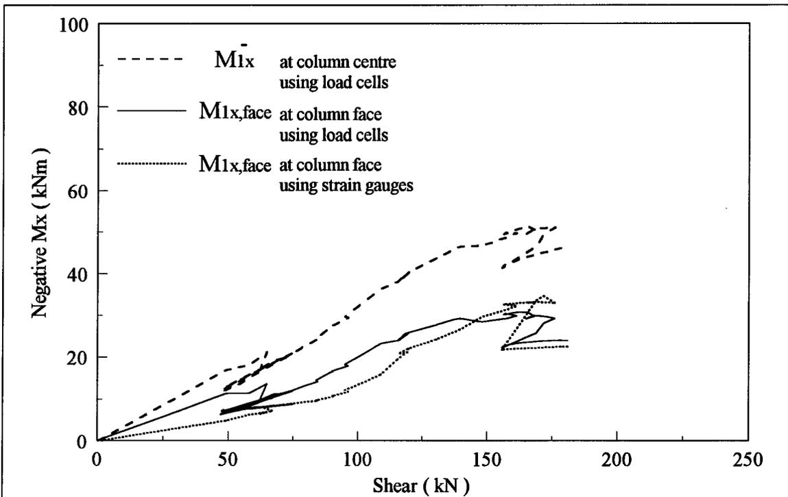
Figure 4.8 Moment -shear diagrams of the north connection
