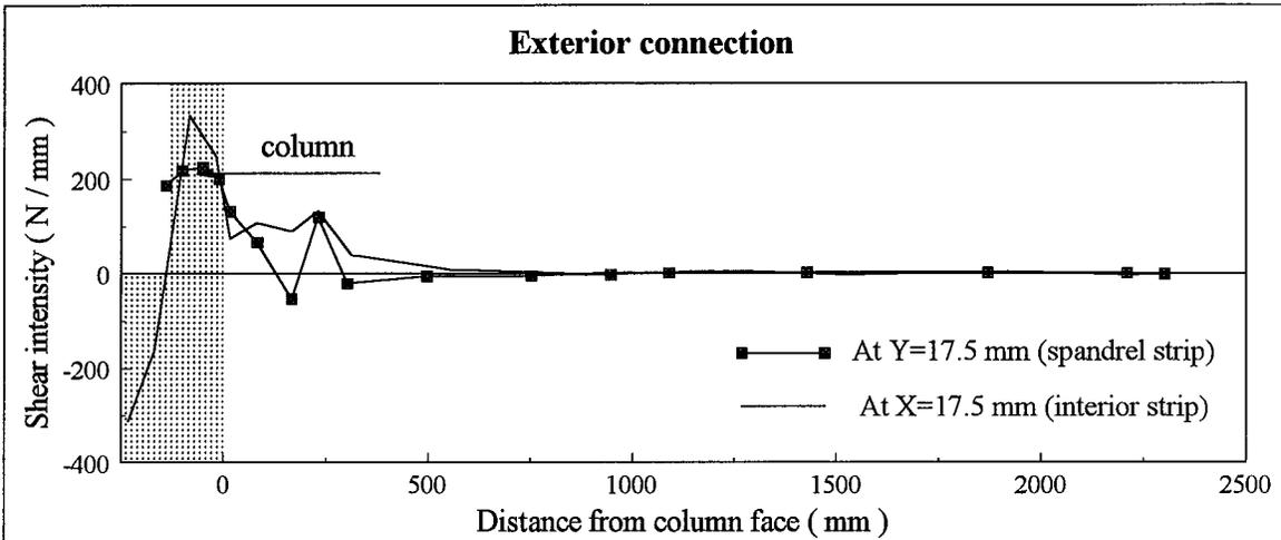
Figure 6.17 Shear intensity at a load of 9 kPa, slab EXT02
