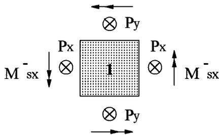
$P_y$  = Shear capacity of radial strip  $y$
