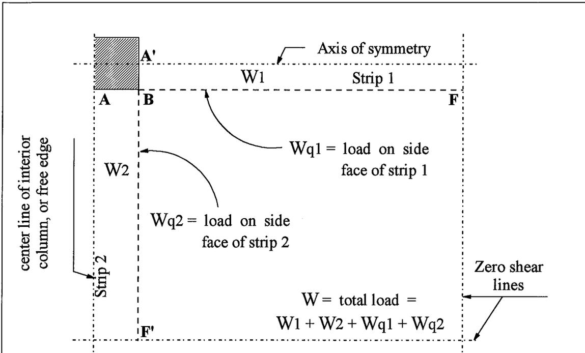
Figure 6.22 Key plan for figures 6.21 through 6.35
