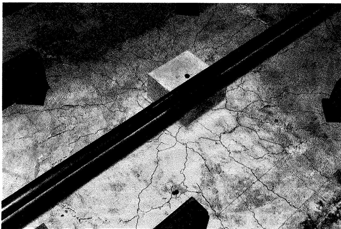
Figure 4.36 Punching of interior connection
