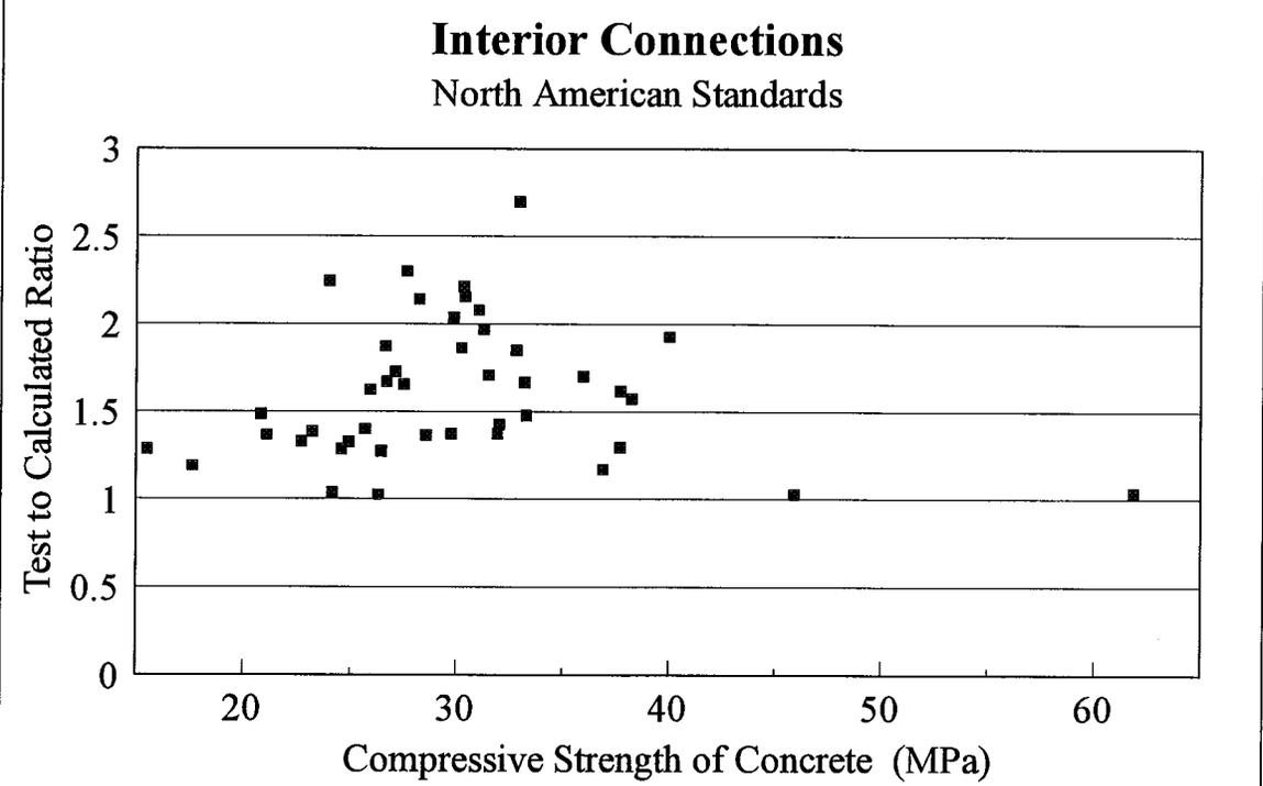
Figure 8.15 Test to calculated ratios of eccentrically loaded interior connections reported in the literature versus the compressive strength of the concrete,  $f_c$
