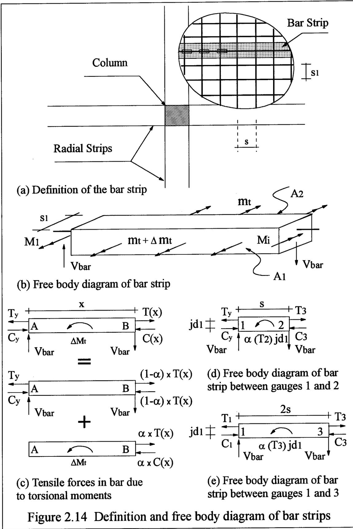
Figure 2.14 Definition and free body diagram of bar strips
