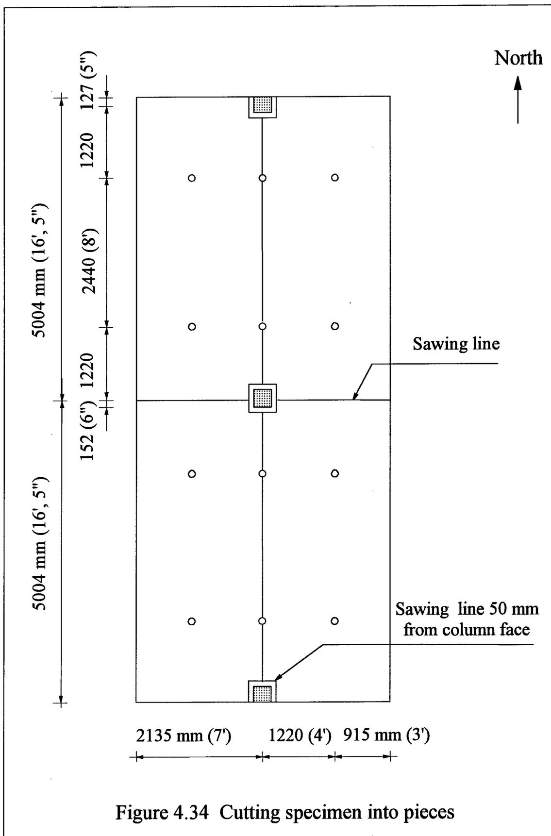
Figure 4.34 Cutting specimen into pieces
