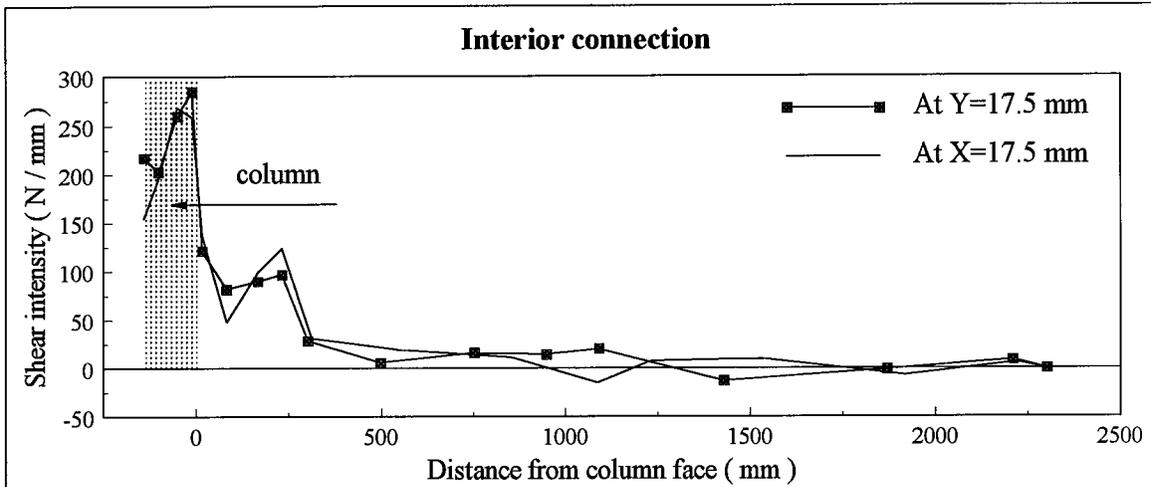
Figure 6.5 Shear intensity at a load of 15 kPa, slab INT01
