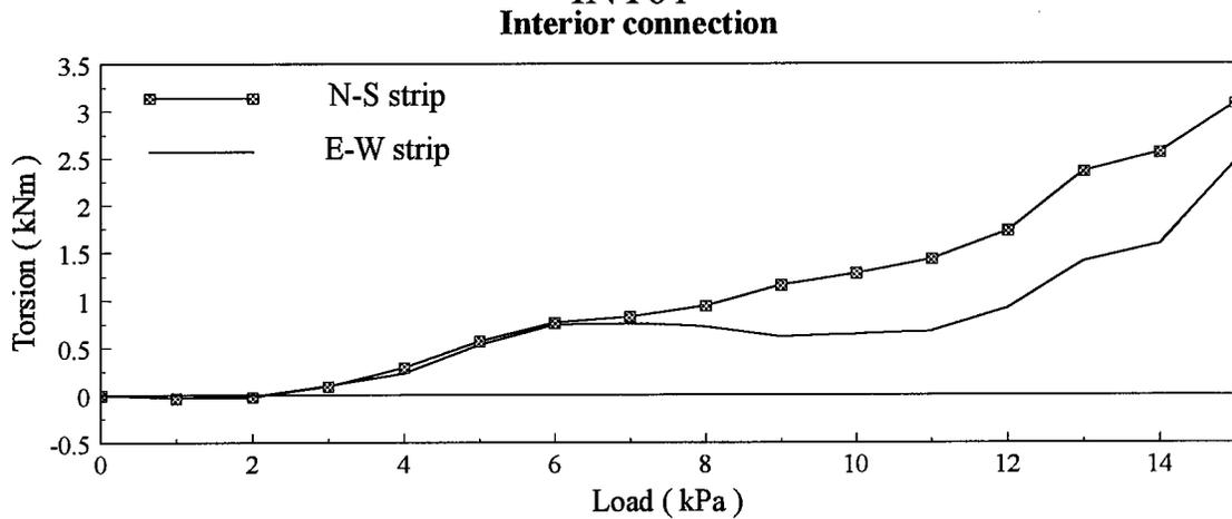
Figure 6.7 Torsional moment along each side face of radial strips, slab INT01
