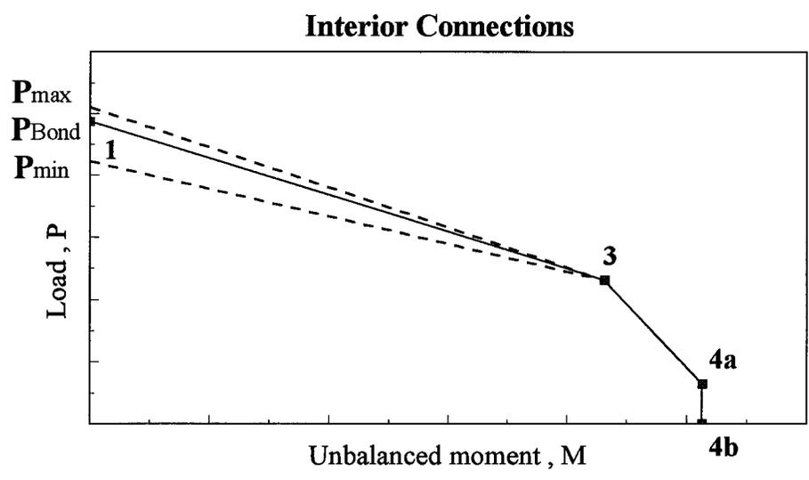
Figure 7.8 Moment-Shear Diagram for the Capacity of Interior Connections - Non-Proportional Behavior
