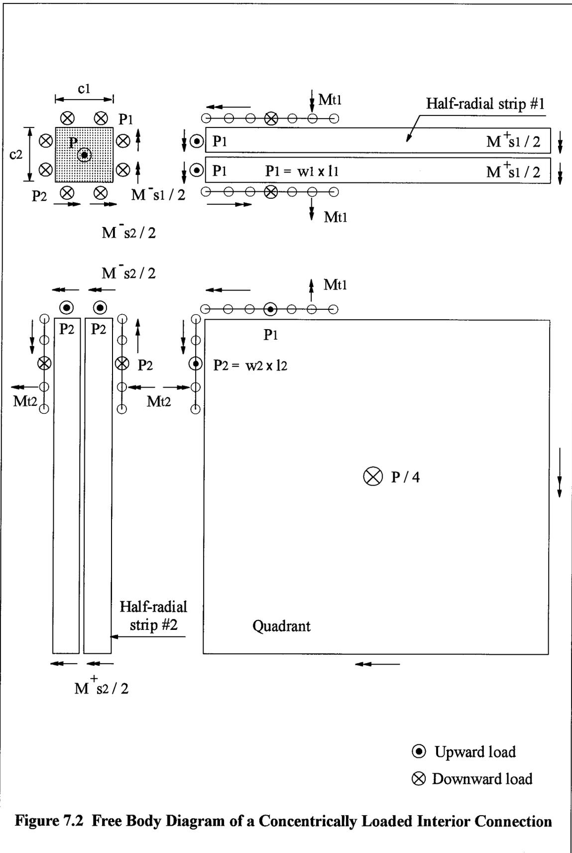
**Figure 7.2 Free Body Diagram of a Concentrically Loaded Interior Connection**
