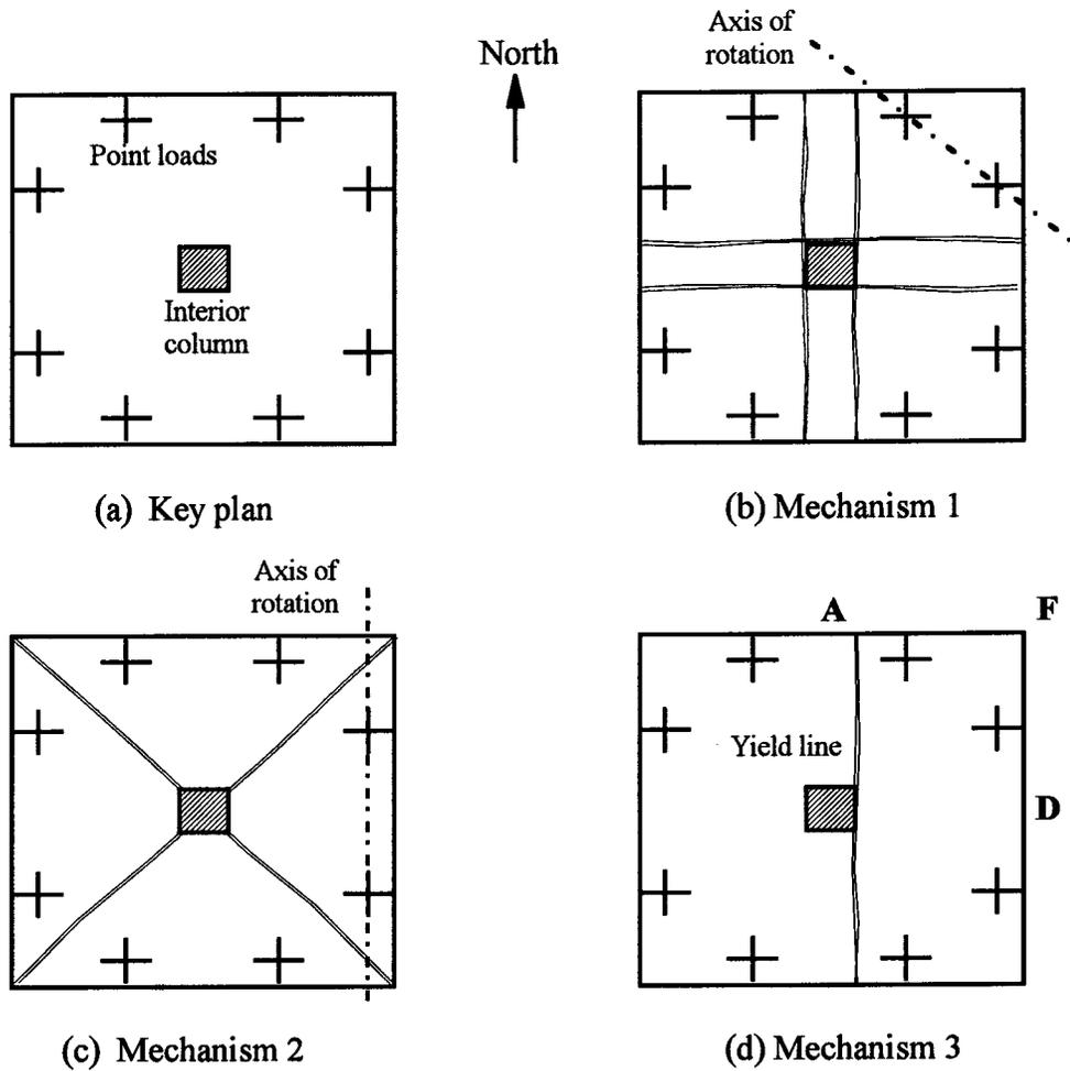
Figure 5.17 An example of possible mechanisms of failure
