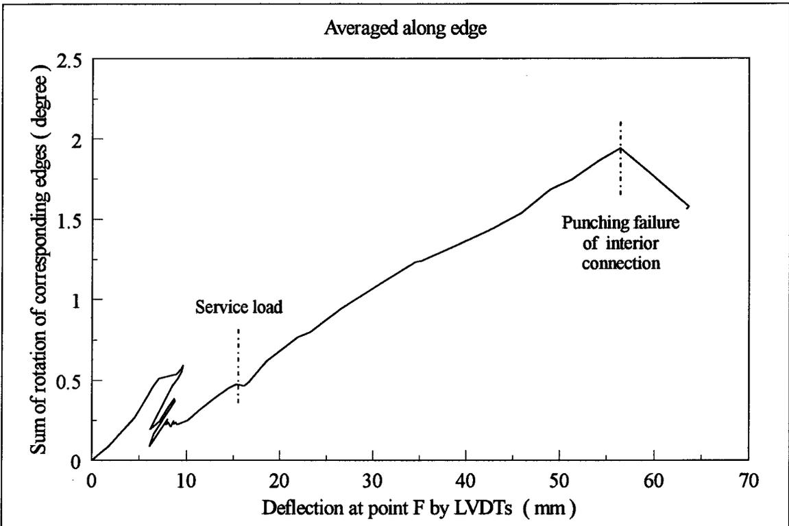
**Figure 4.24 Sum of rotation of corresponding continuous edges**
