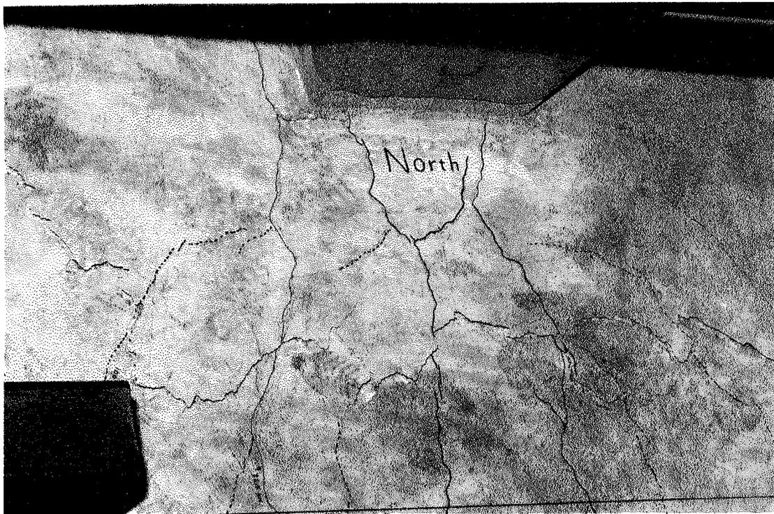
Figure 4.38 Punching of north connection
