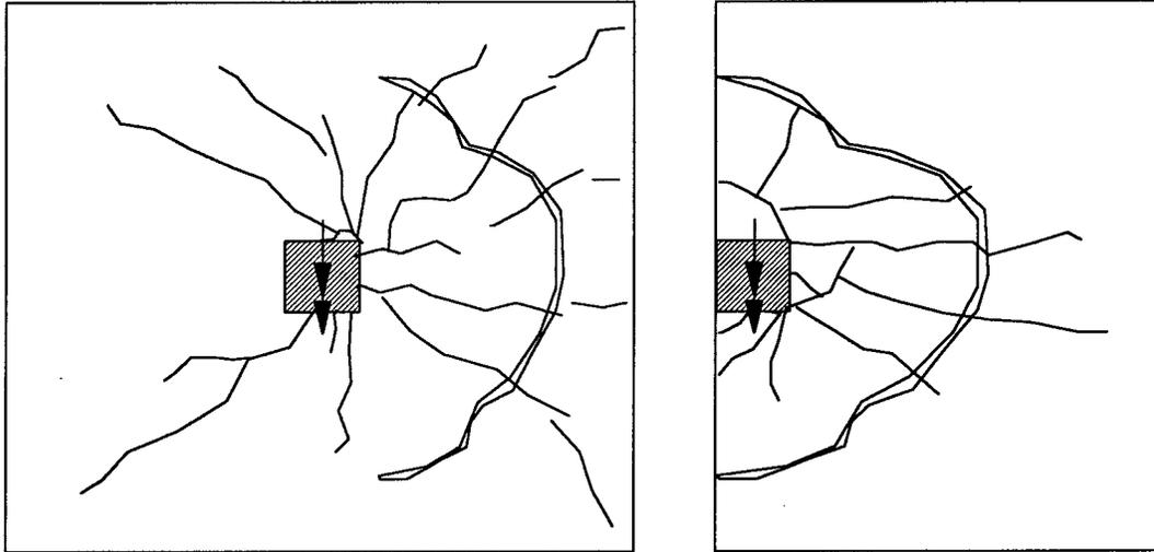
Figure 2.3 Typical punching failure of plate-column connections with unbalanced moments
