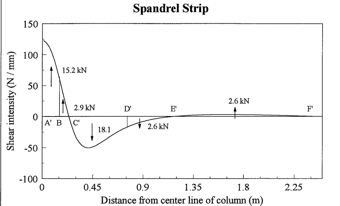
Figure 6.36 Idealized torsional shear intensity diagram along side faces of spandrel strips
