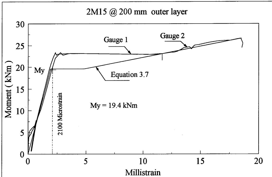
Figure 3.27 Moment-Strain Relationship for Beam 3
