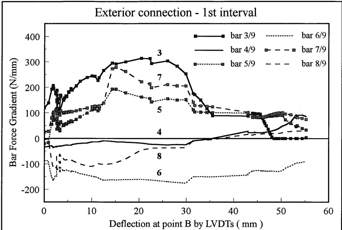
**Figure B7 - Force gradient in bars running E-W, south connection, 1st interval**
