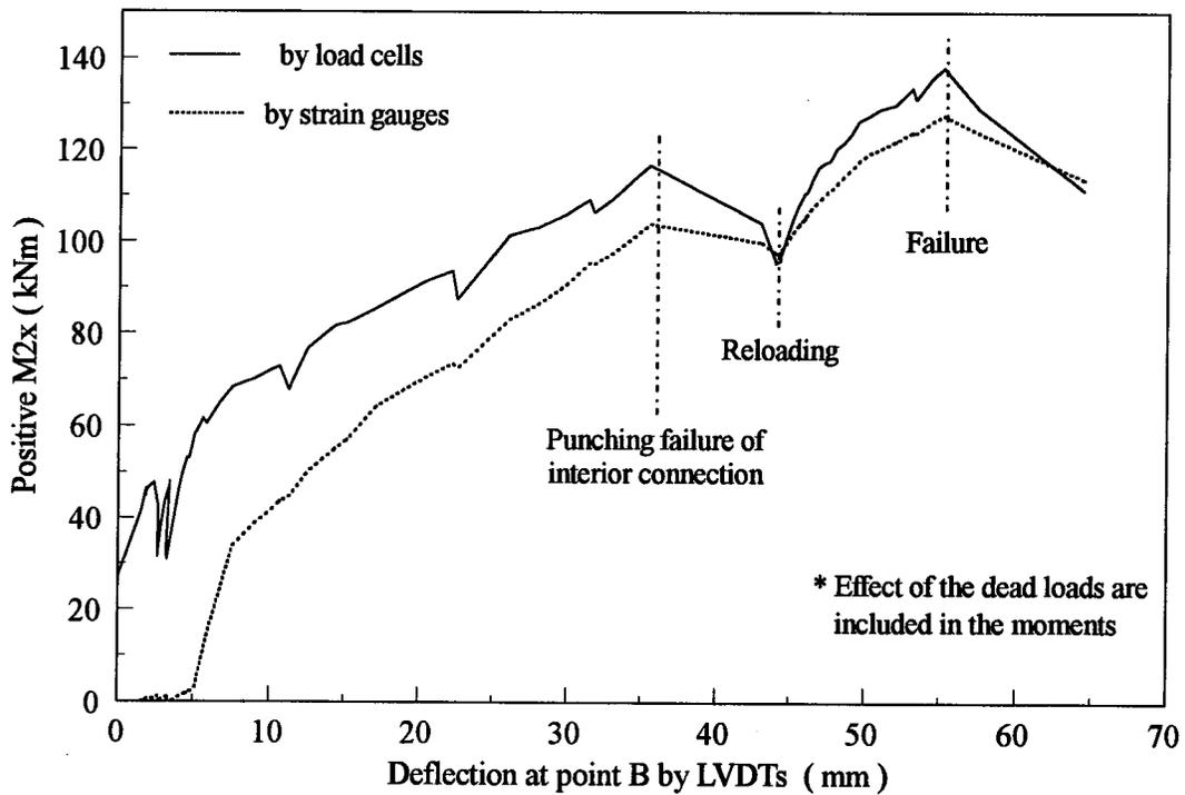
Figure 4.15 Positive moment in x direction, south panel
