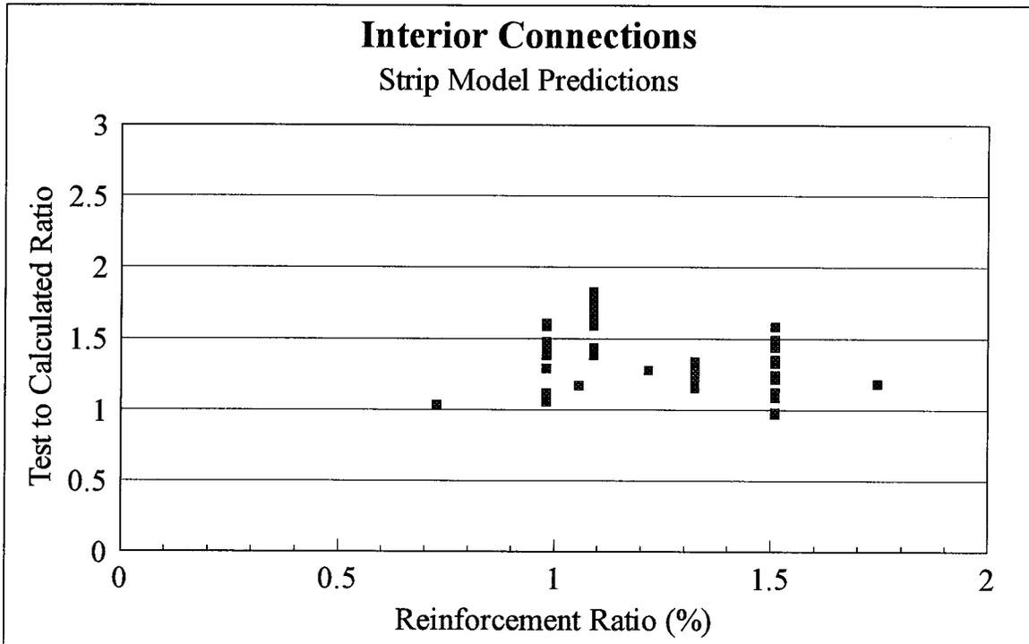
Figure 8.5 Test to calculated ratios of eccentrically loaded interior connections reported in the literature versus the reinforcement ratio
