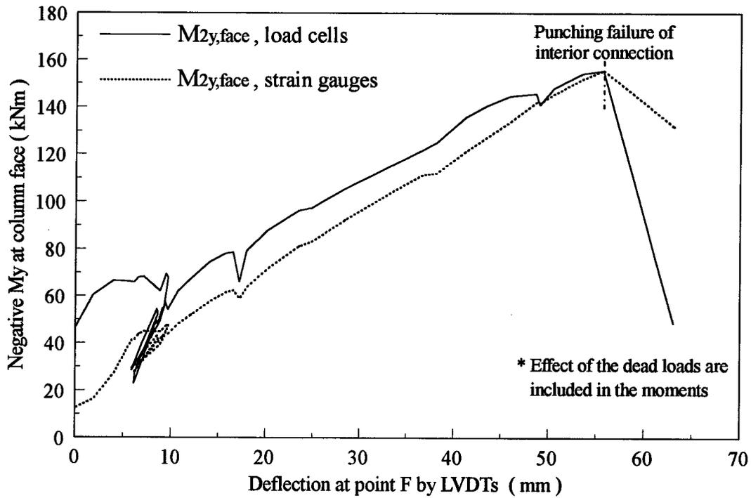
Figure 4.18 Negative moment in the y direction at the face of the interior column versus the deflection of the specimen
