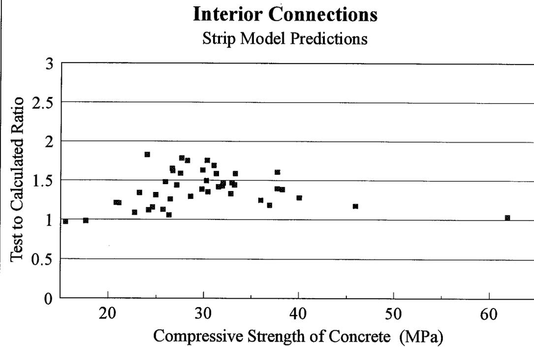
Figure 8.6 Test to calculated ratios of eccentrically loaded interior connections reported in the literature versus the compressive strength of the concrete,  $f_c$
