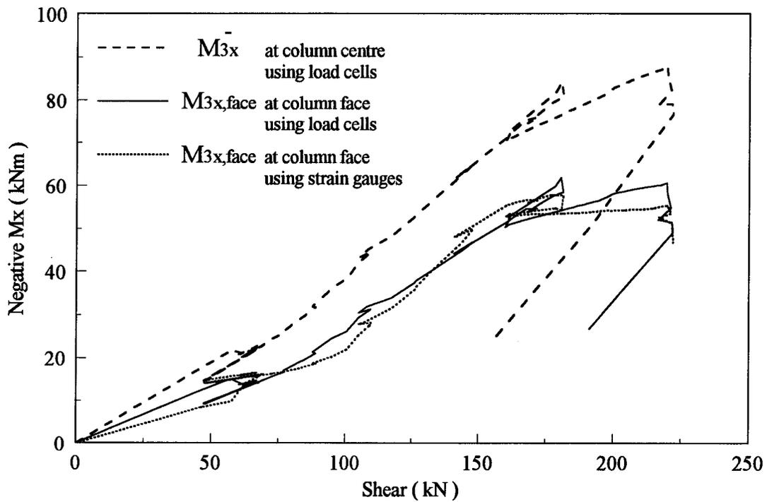
Figure 4.9 Moment -shear diagrams of the south connection
