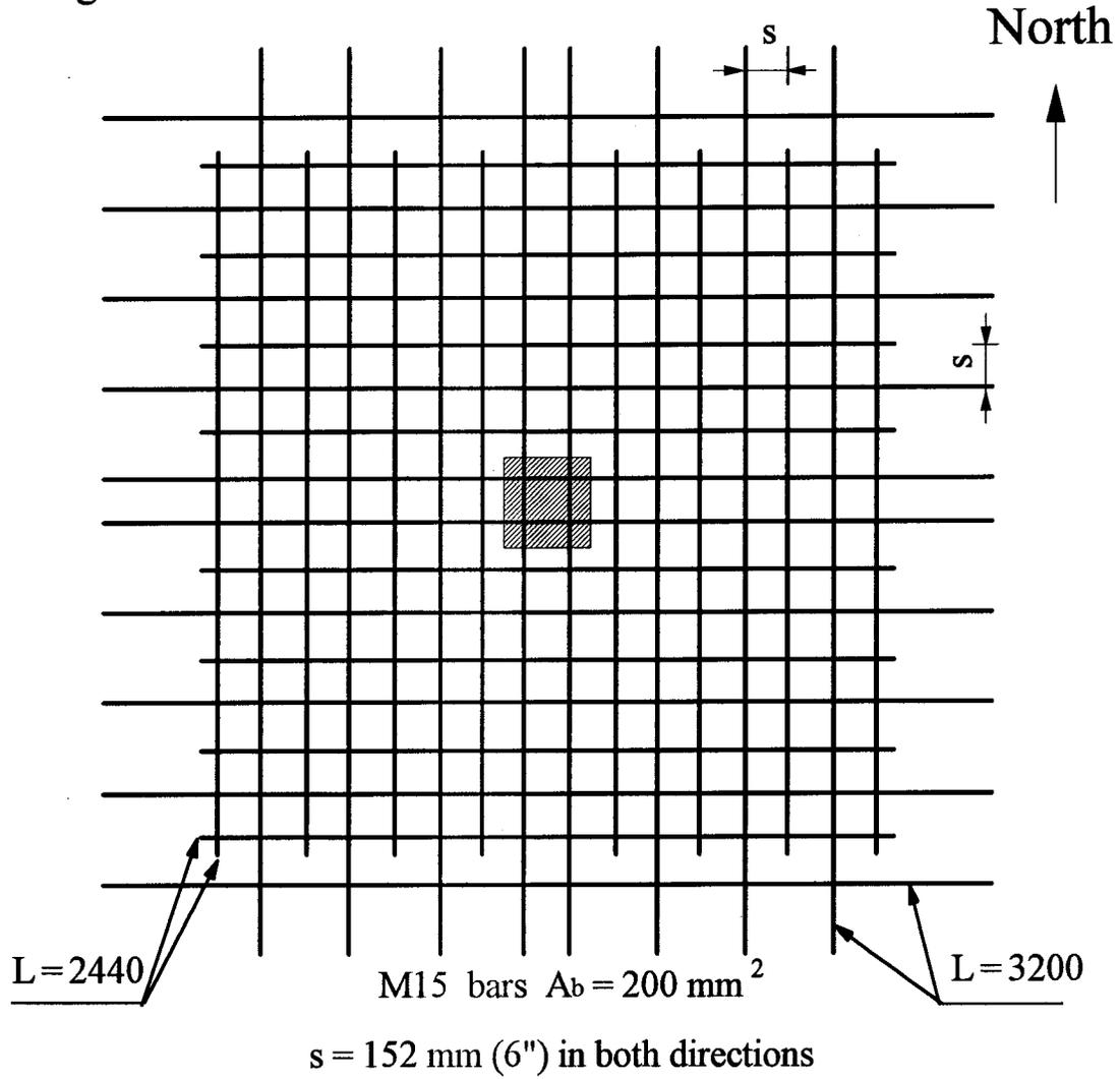
Figure 3.6 Top reinforcement around interior column
