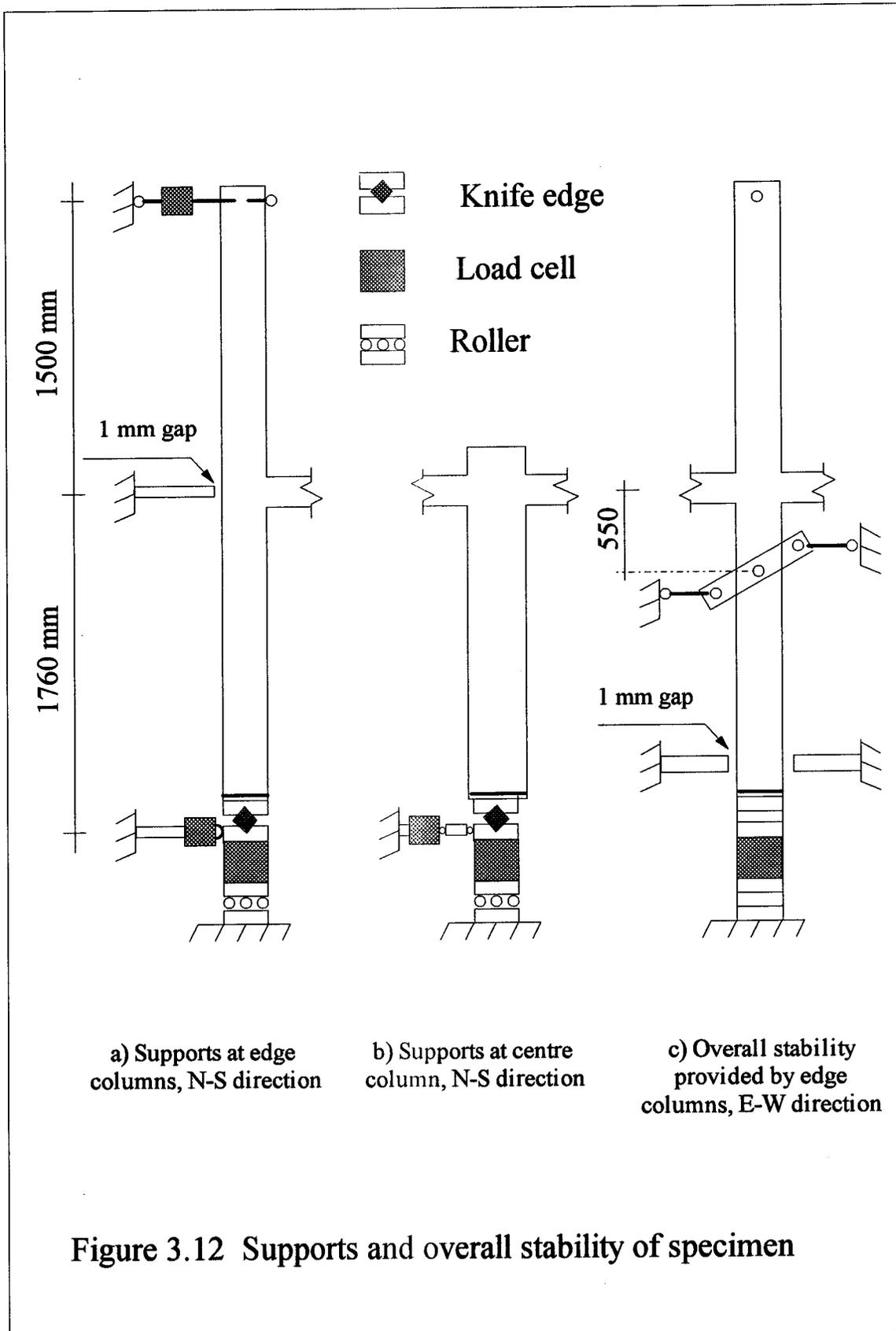
**Figure 3.12 Supports and overall stability of specimen**
