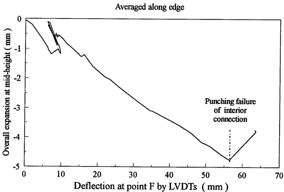
Figure 4.23 Overall expansion at mid-height of the continuous edge
