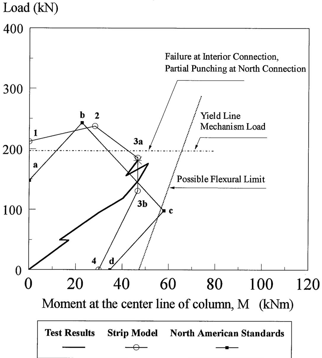
Figure 8.16 Comparison of North American standards, Strip Model, and the test results of the north edge connection in the current study
