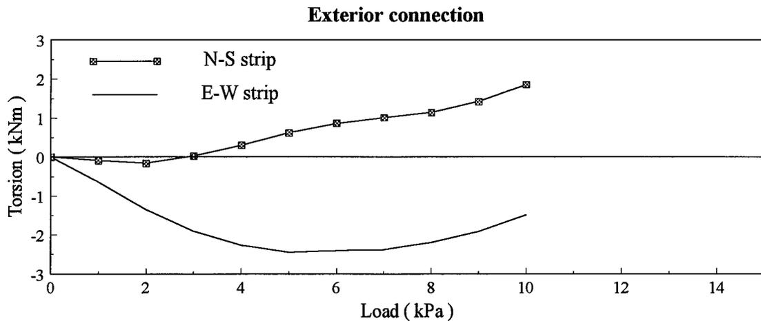
Figure 6.16 Torsional moment along each side face of radial strips, slab EXT01
