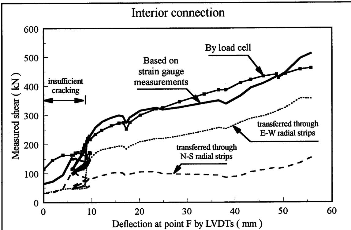
**Figure 5.9 Measured shear at interior connection by load cell and strain gauges**
