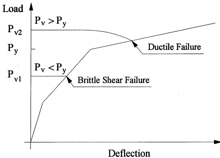
Figure 2.4 Brittle and Ductile Punching Failures
