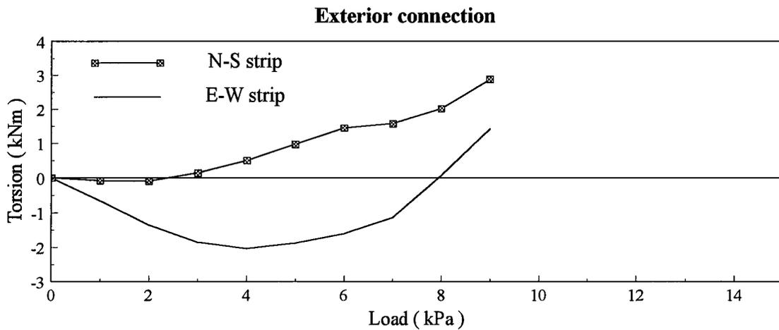
Figure 6.19 Torsional moment along each side face of radial strips, slab EXT02
