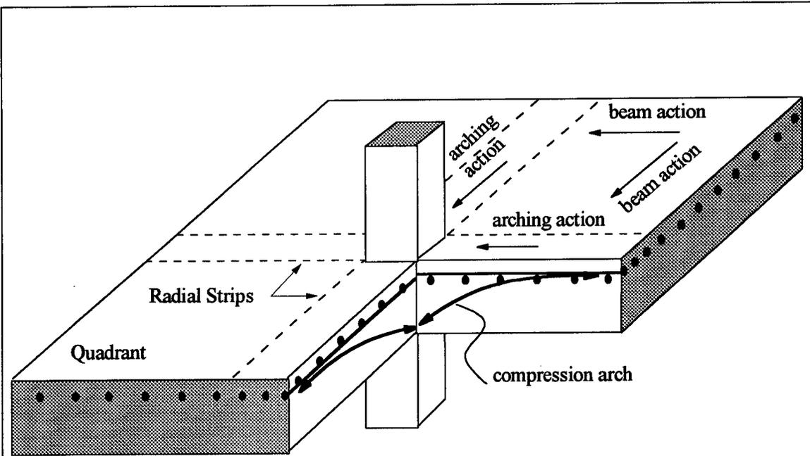
Figure 2.6 Shear transfer in flat plate-column connections
