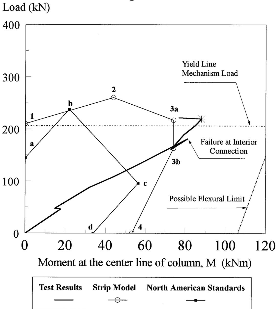
Figure 8.17 Comparison of North American standards, Strip Model, and the test results of the south edge connection in the current study
