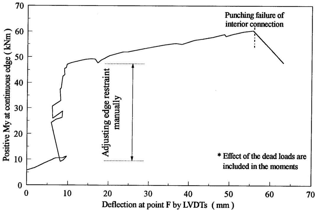
Figure 4.19 Positive moment in the y direction at the continuous edges versus the deflection of the specimen
