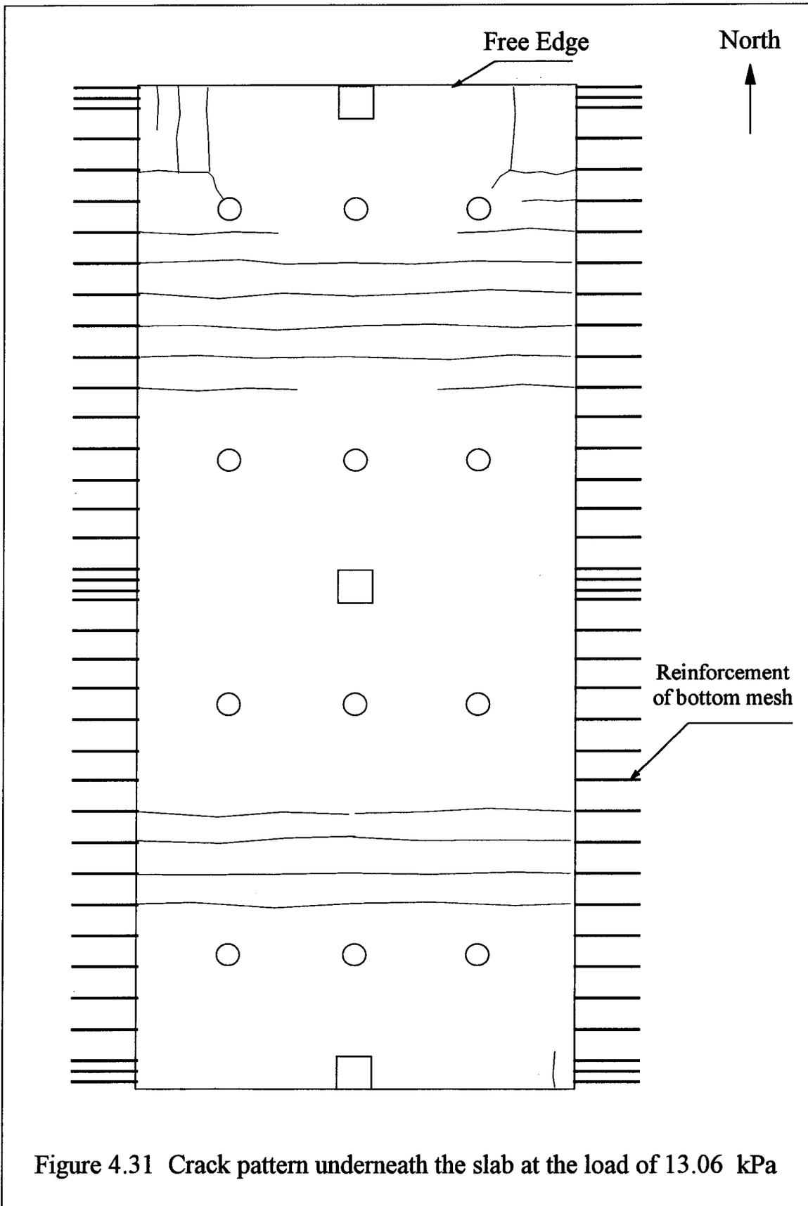
Figure 4.31 Crack pattern underneath the slab at the load of 13.06 kPa
