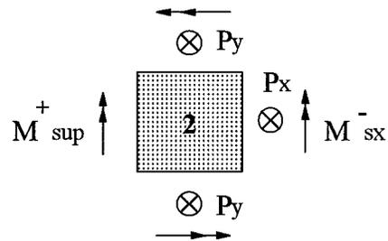
$P_y$  = Shear capacity of radial strip  $y$
