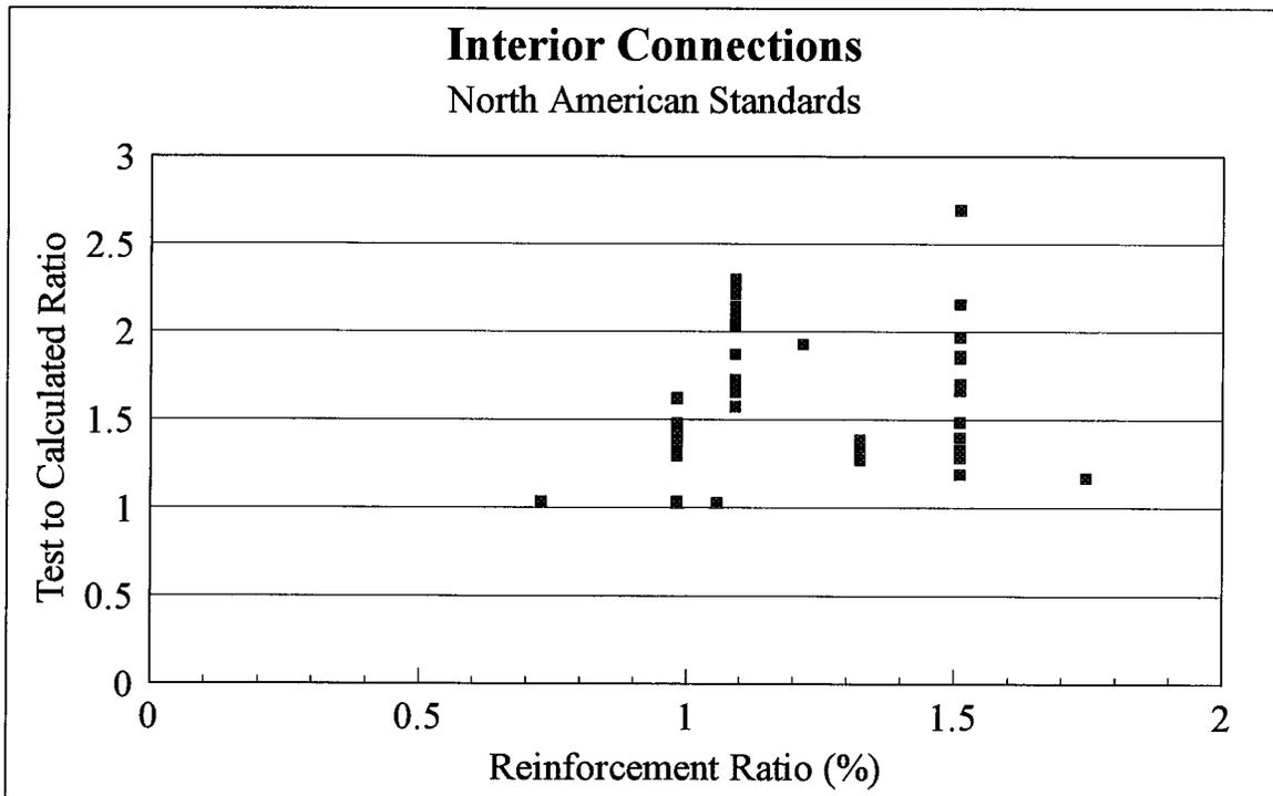
Figure 8.14 Test to calculated ratios of eccentrically loaded interior connections reported in the literature versus the reinforcement ratio
