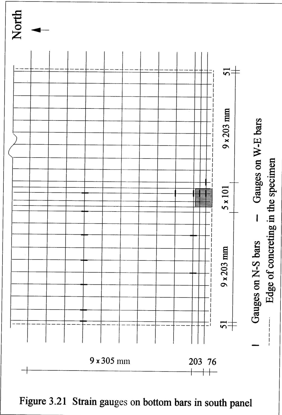
Figure 3.21 Strain gauges on bottom bars in south panel
