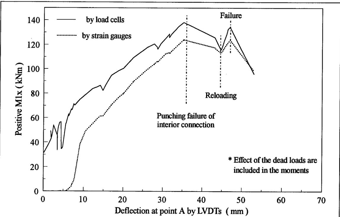
Figure 4.14 Positive moment in x direction, north panel
