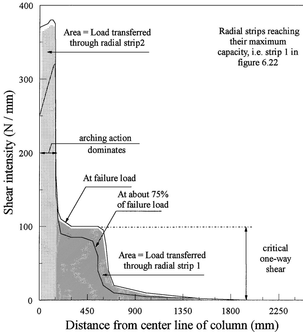
Figure 6.27 Typical shear intensity diagram along side faces of interior radial strips, case a
