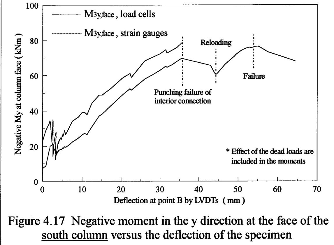
Figure 4.17 Negative moment in the y direction at the face of the south column versus the deflection of the specimen
