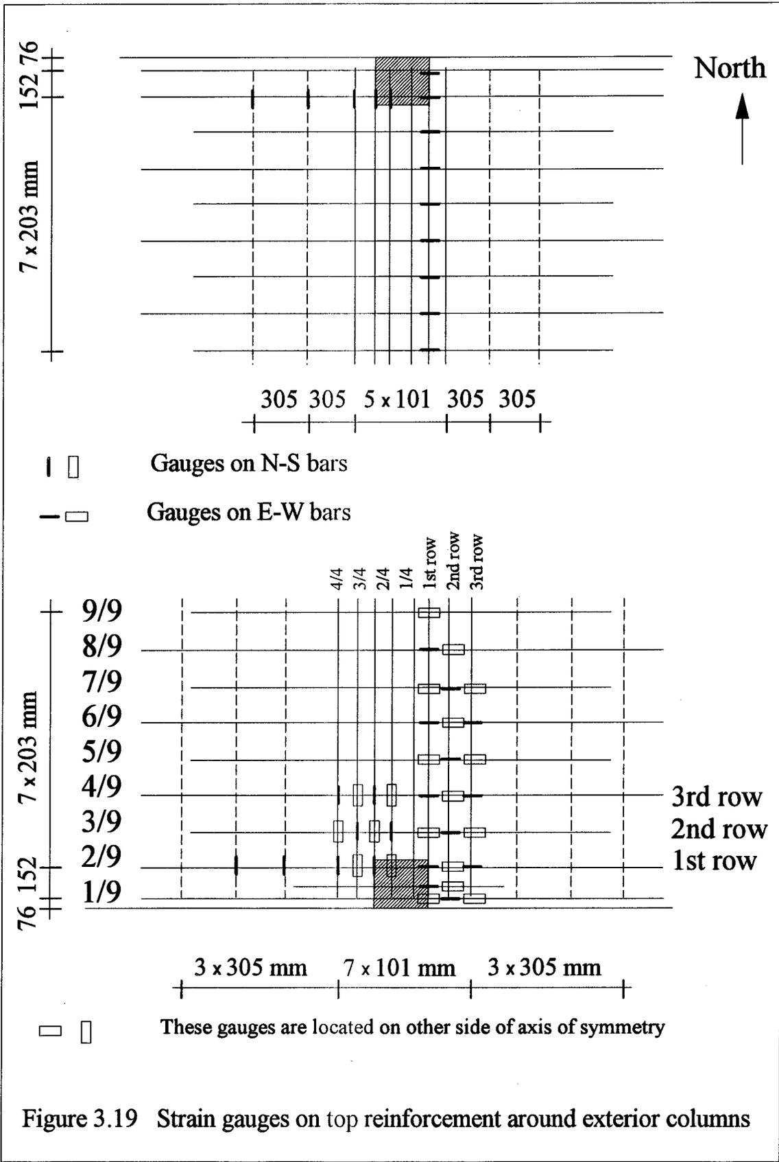
Figure 3.19 Strain gauges on top reinforcement around exterior columns
