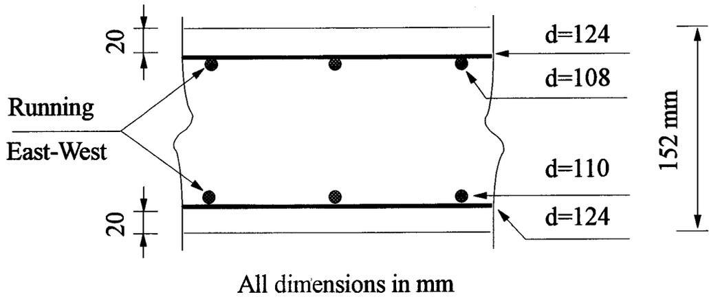
Figure 3.5 Cross section of slab
