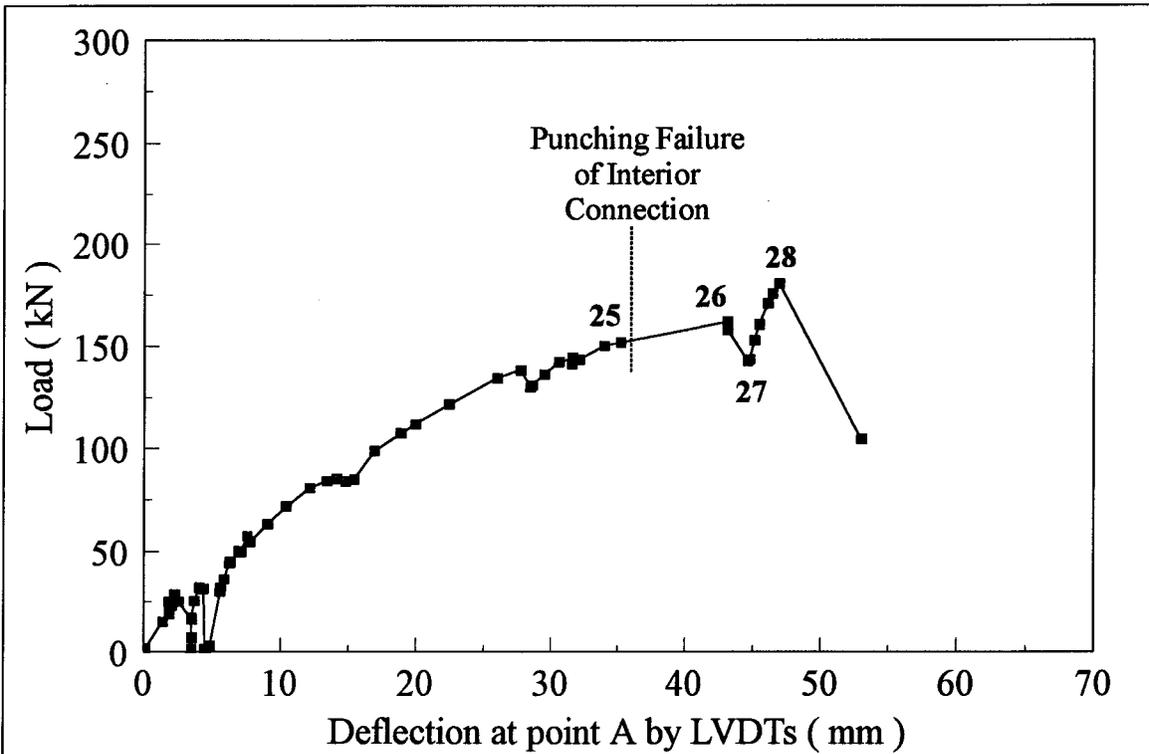
Figure 4.2 Load in jack #1 versus the deflection of the specimen
