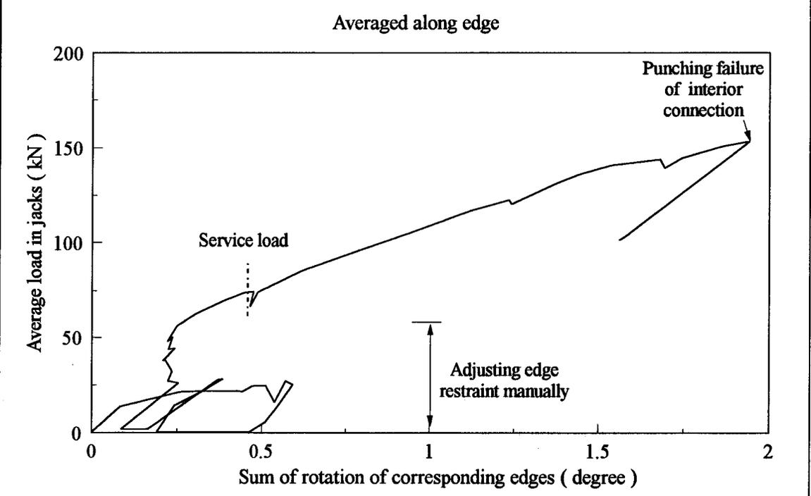
**Figure 4.25 Average load in jacks versus the rotation of the continuous edge**
