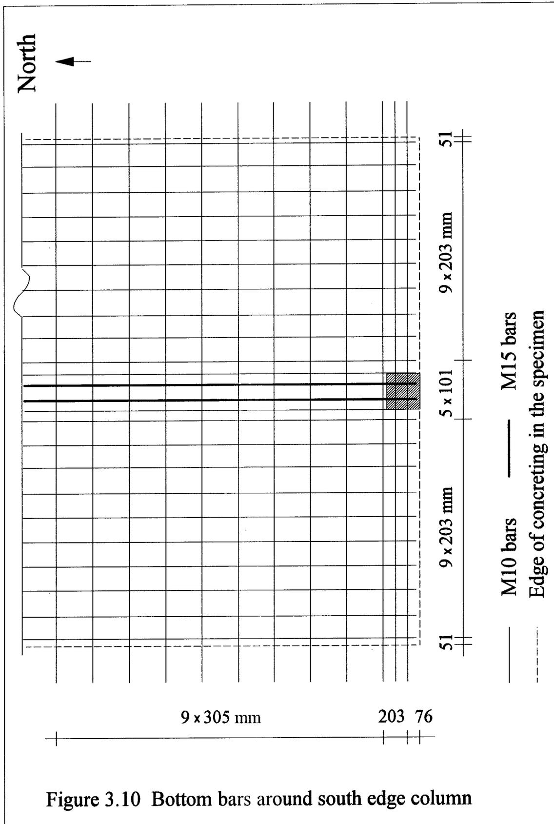
Figure 3.10 Bottom bars around south edge column
