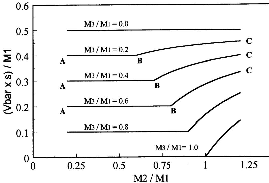
Figure 5.6 Suggested equations (5.4 and 5.5) for  $V_{\text{bar}}$
