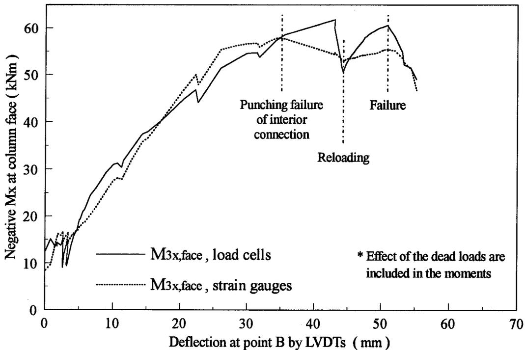
Figure 4.13 Negative moment in the x direction at the face of the south column versus the deflection of the specimen
