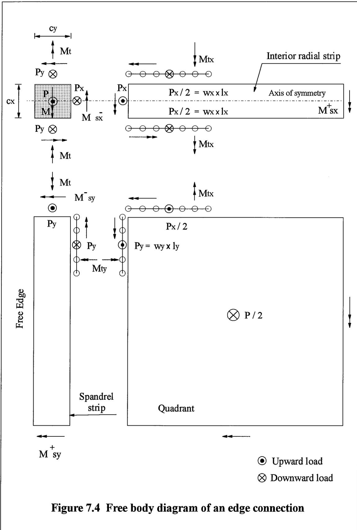
**Figure 7.4 Free body diagram of an edge connection**
