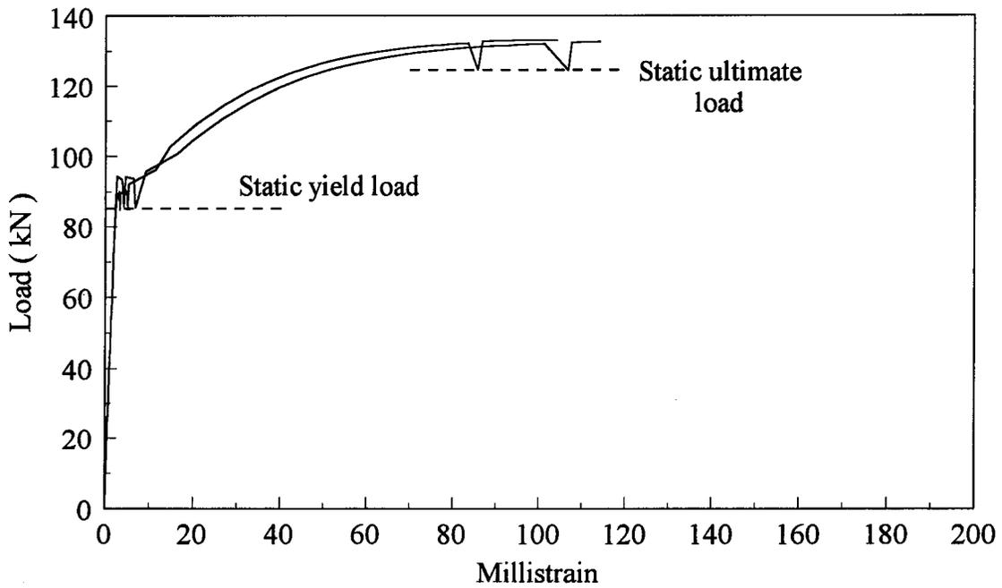
(b) 15M deformed bars with nominal area of 200 mm<sup>2</sup>
