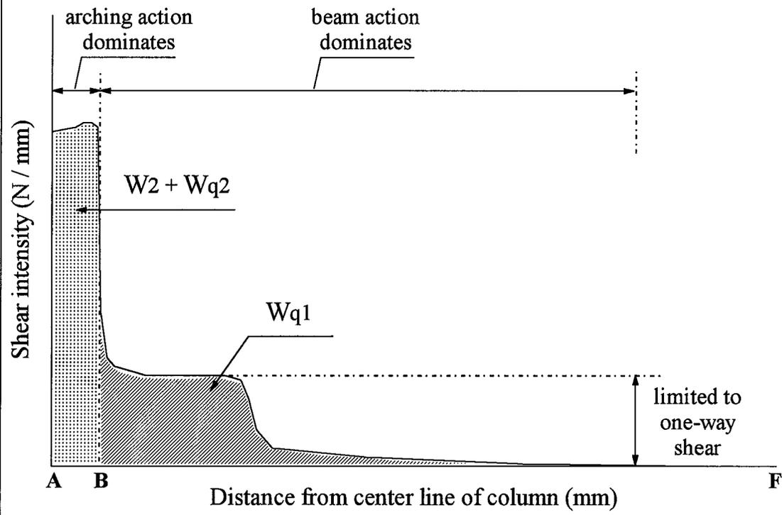
Figure 6.23 Typical shear intensity diagram along section ABF
