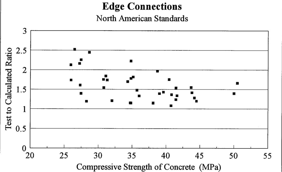
Figure 8.12 Test to calculated ratios of the edge connections reported in the literature versus the compressive strength of the concrete,  $f_c$
