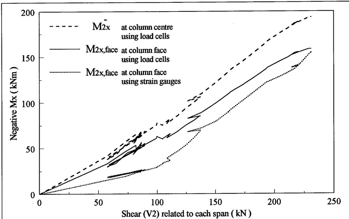
Figure 4.10 Moment-shear diagrams of the interior connection
