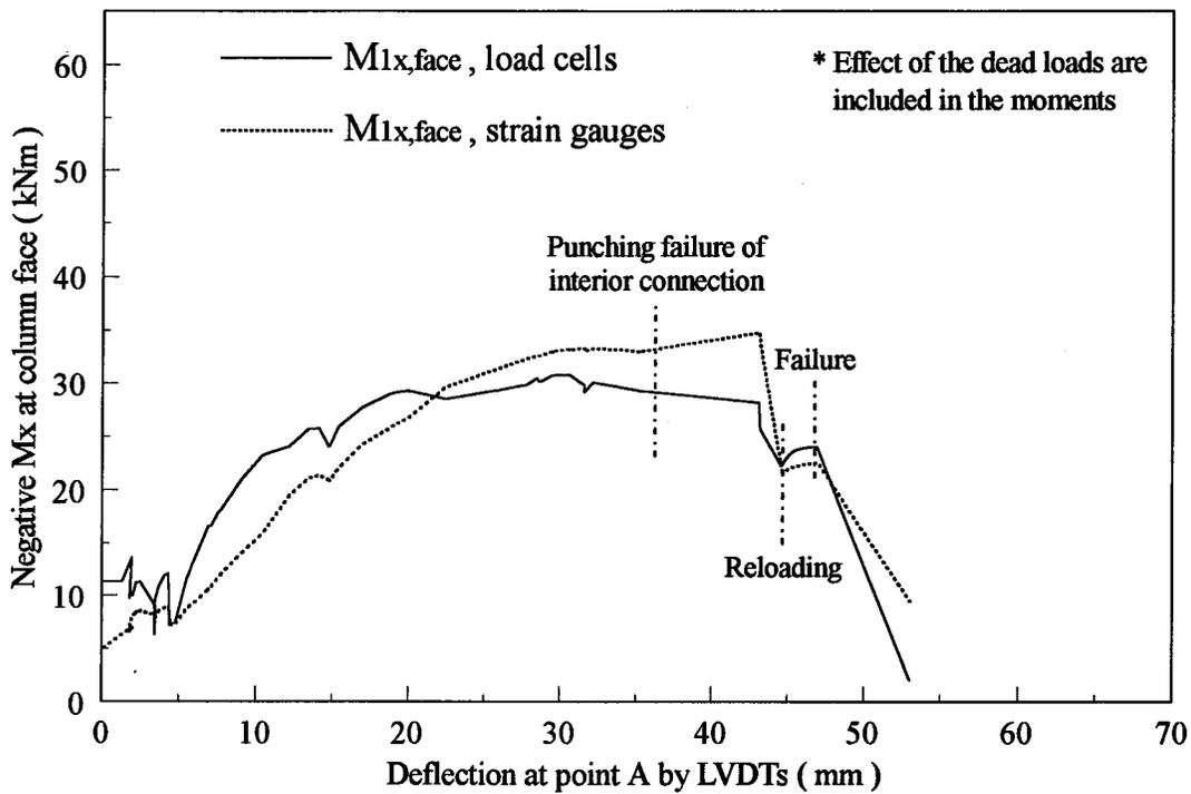
Figure 4.12 Negative moment in the x direction at the face of the north column versus the deflection of the specimen
