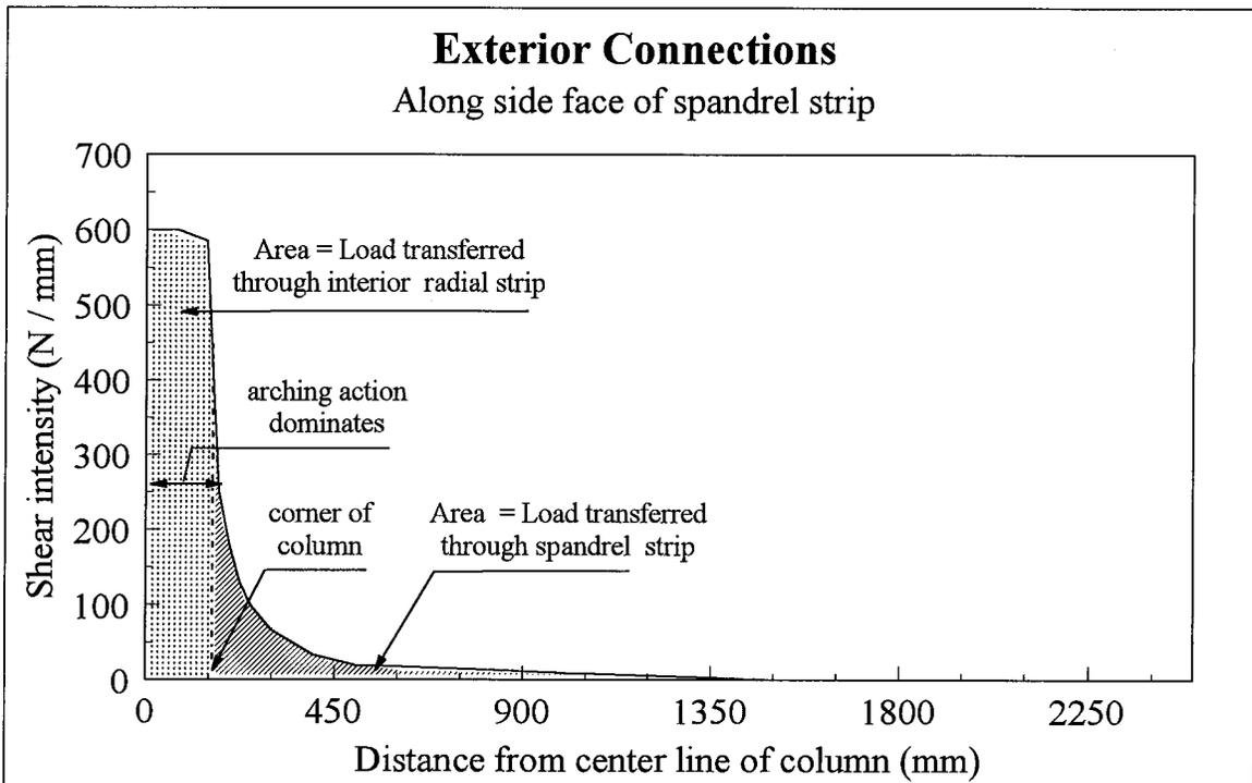
Figure 6.33 Typical shear intensity diagram along side face of a spandrel strip
