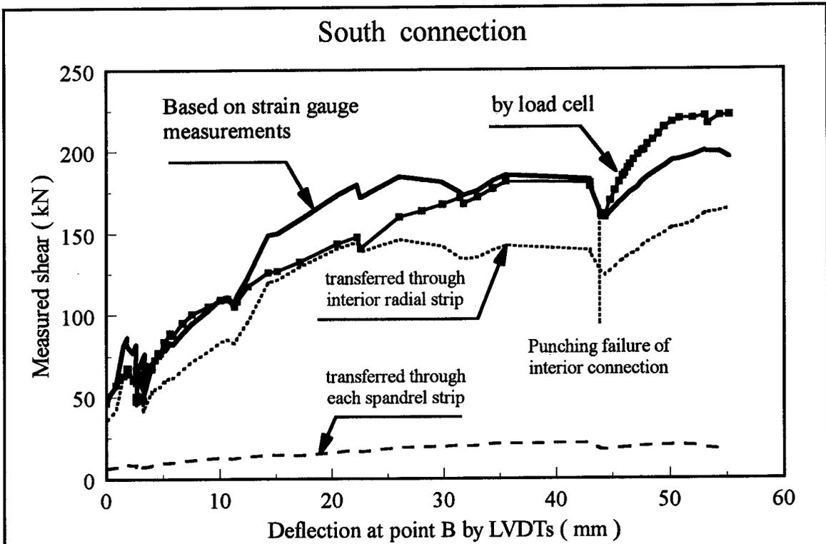
**Figure 5.13 Measured shear at south connection by load cell and strain gauges**
