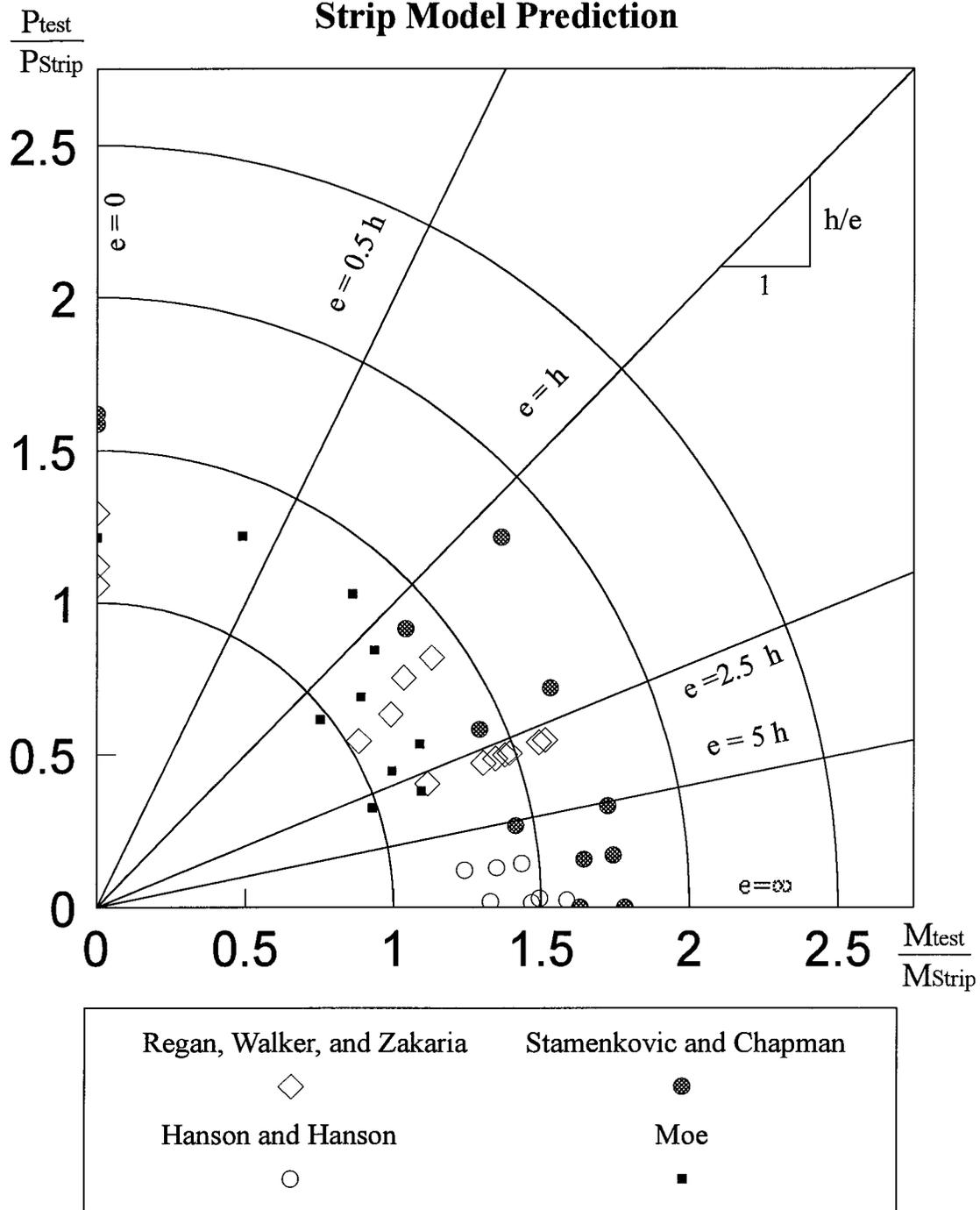
Figure 8.4 Test to calculated ratio for the interior connections reported in the literature - Strip Model
