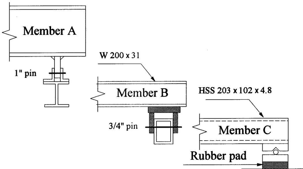
Figure 3.15 Connections of load distributing beams
