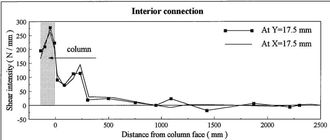
Figure 6.8 Shear intensity at a load of 14 kPa, slab INT02
