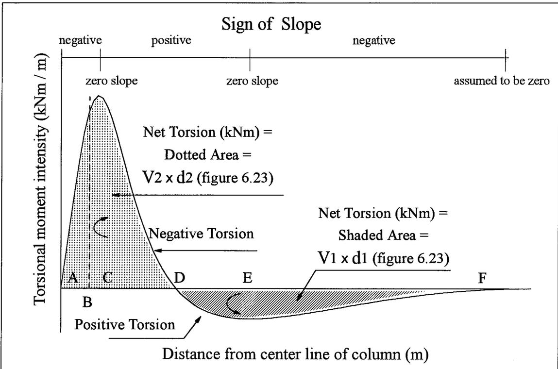
**Figure 6.24 Typical torsional moment intensity diagram along side faces of strip 1**
