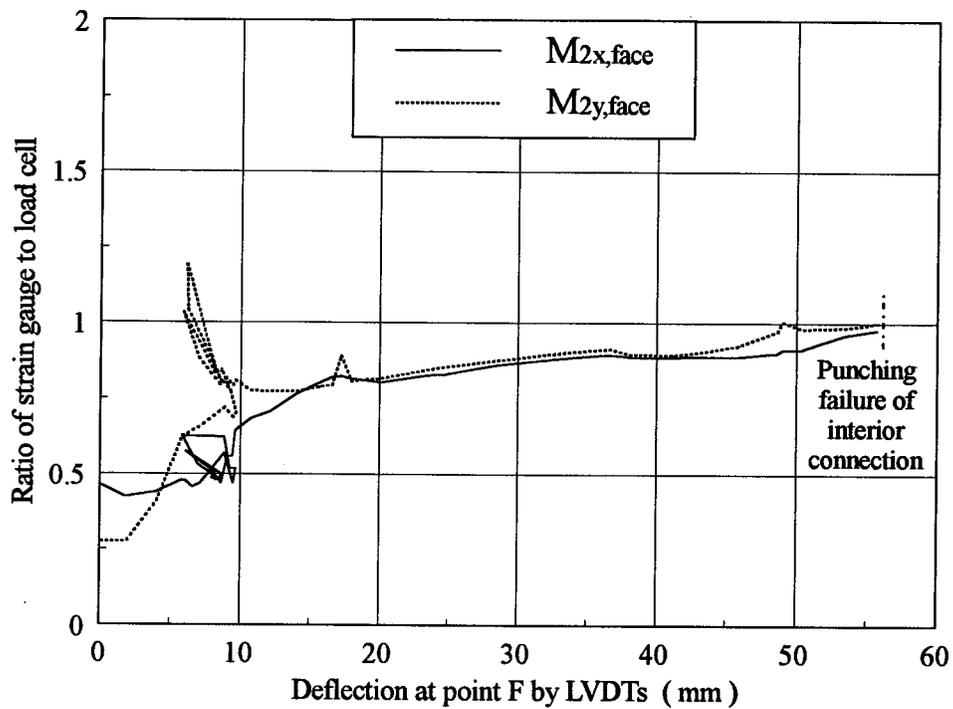
Figure 4.22 Comparison of the external measurements with the internal measurements in the interior connection
