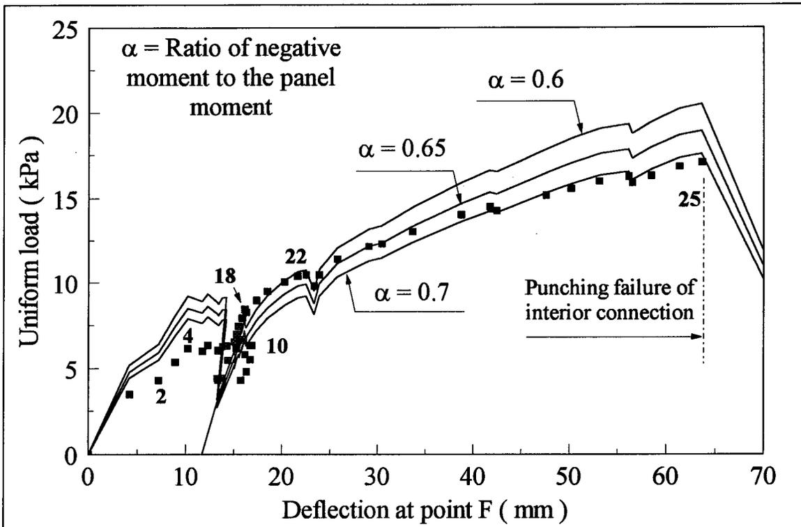
Figure 4.4 Load-Deflection Diagram - Ideal Edge Restraint
