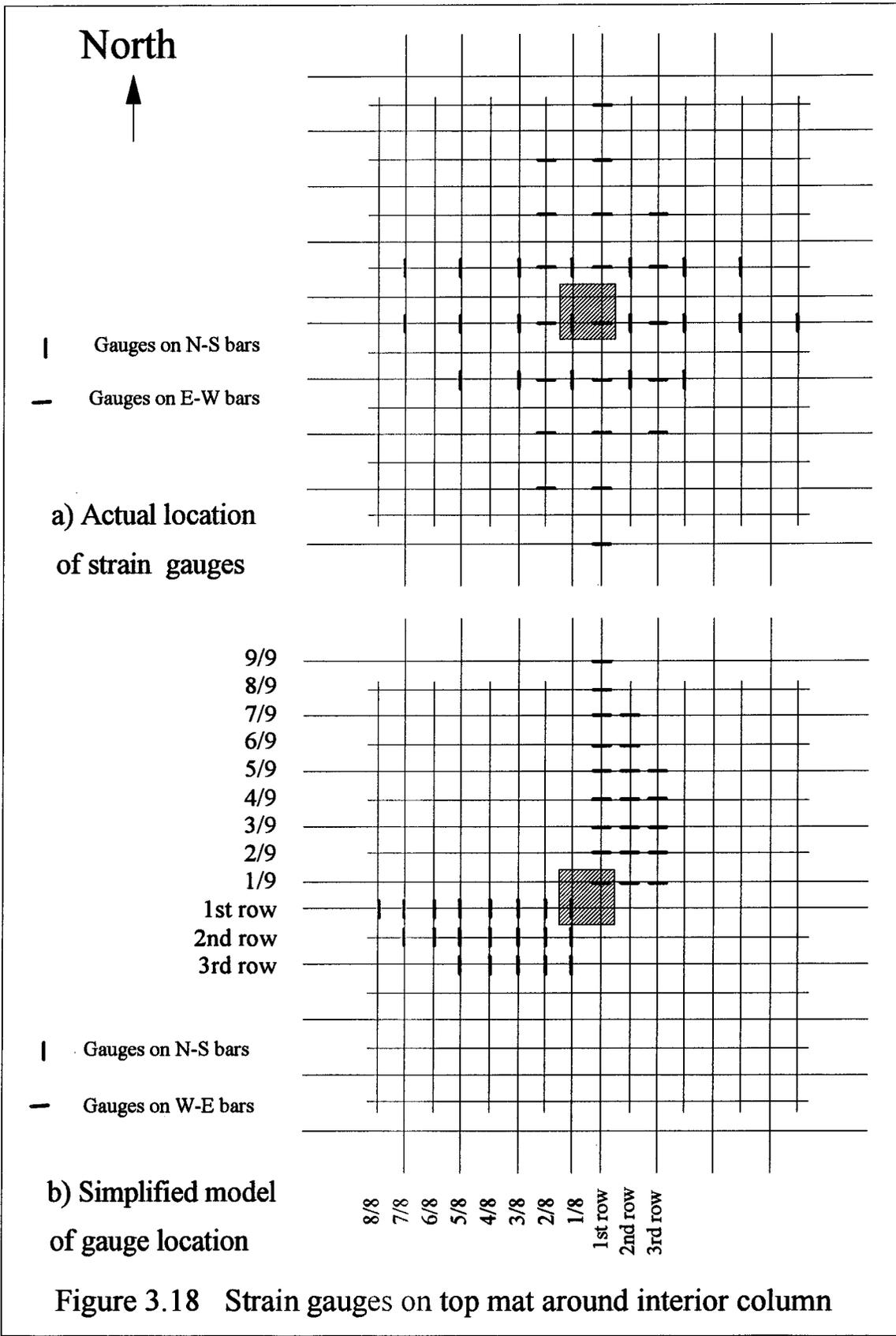
Figure 3.18 Strain gauges on top mat around interior column
