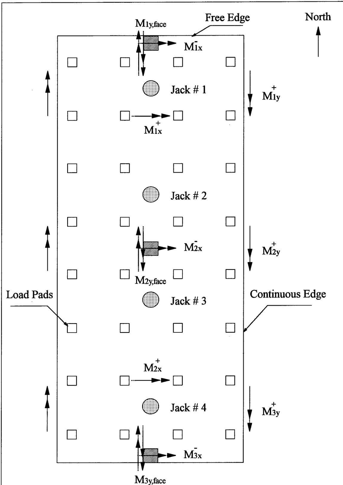
Figure 4.6 Definition and position of loads and moments
