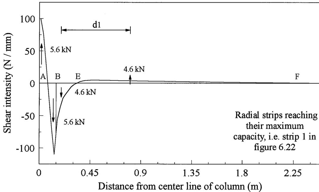
Figure 6.29 Idealized torsional shear intensity diagram along side faces of interior radial strips, case a
