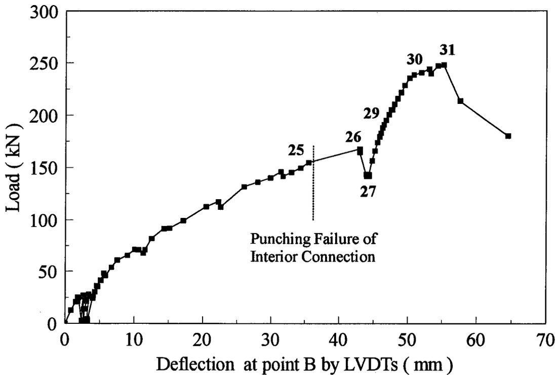
Figure 4.3 Load in jack #4 versus the deflection of the specimen
