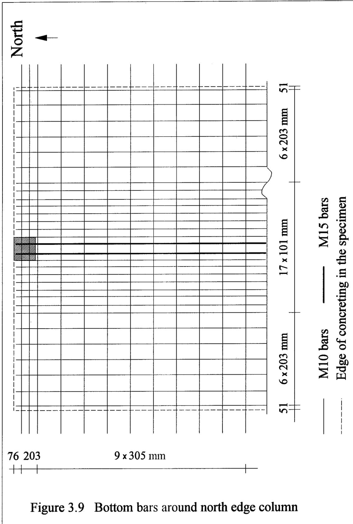
Figure 3.9 Bottom bars around north edge column
