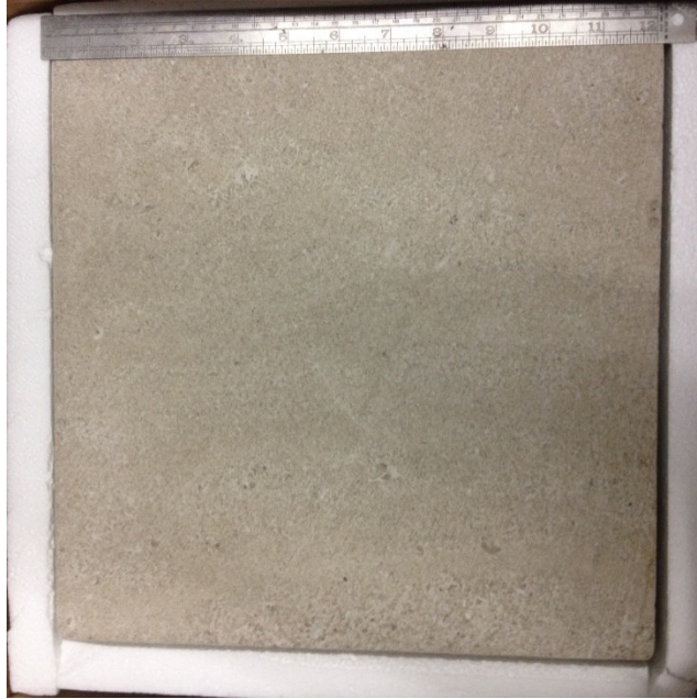
Figure 4.1 Top view of one raw block of Indiana Limestone used for rock strength experiments. A ruler is shown for scale.
