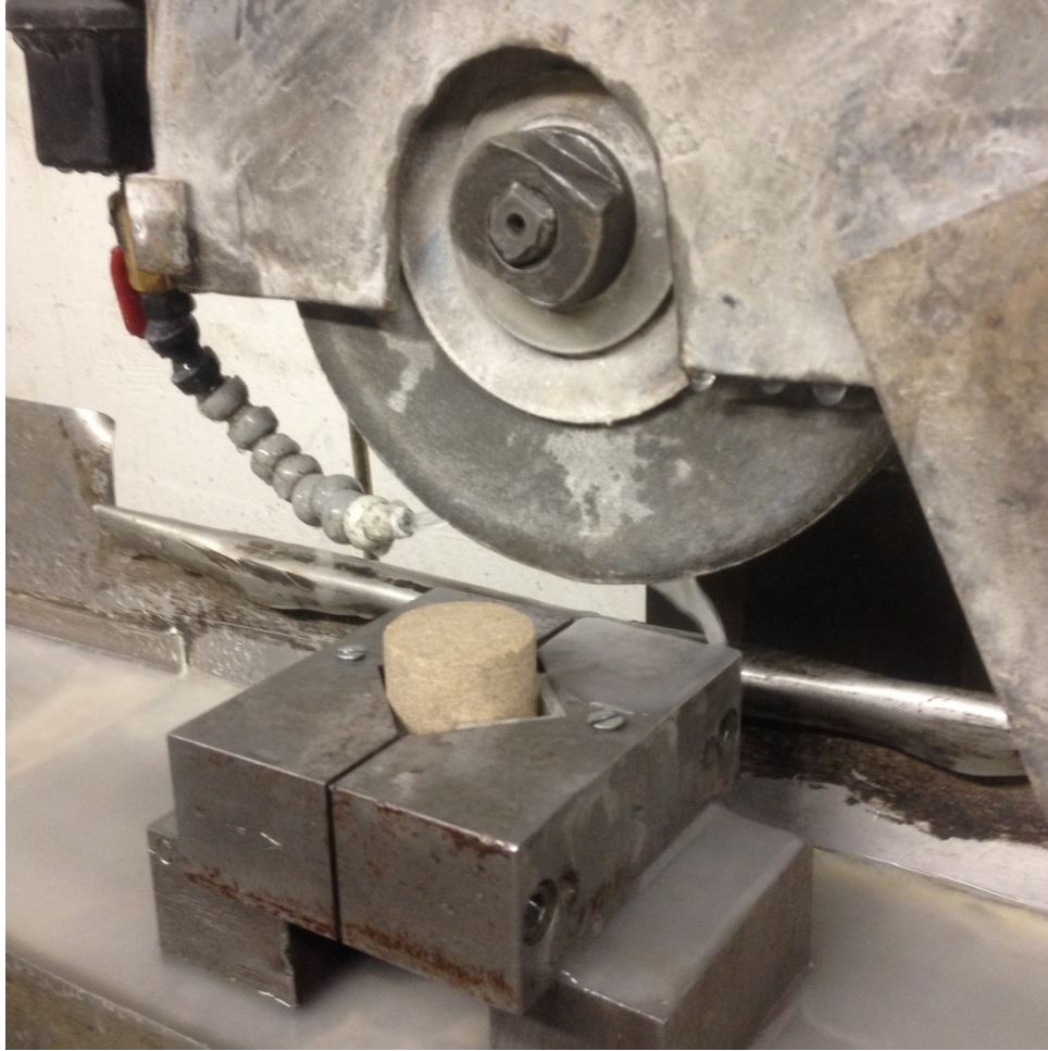
Figure 4.4 Photo of the surface grinder used to machine the ends of the cored specimens. Specially machined V-blocks are used to hold the sample in place on the flat, magnetic surface. The surface grinder operates manually and like the coring process, a pump provides water to the surface of the grinding wheel acting to cool and wash away cuttings.
