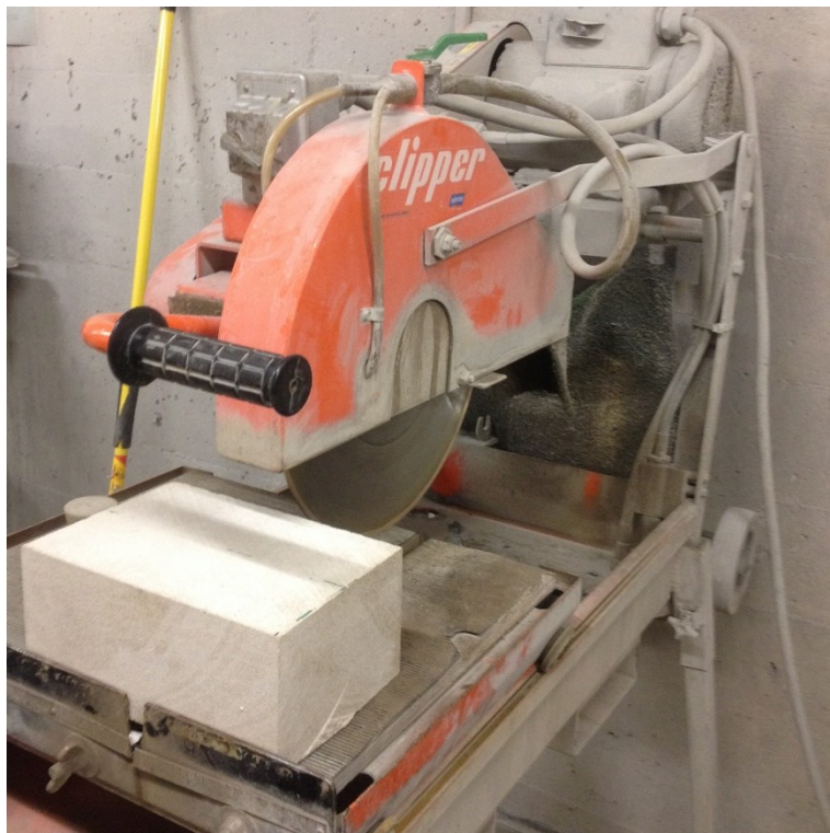
Figure 4.2 Image of the diamond rock saw used to cut Indiana limestone blocks. The blocks are fed into the saw by a manually movable platform. Water is pumped onto the blade to wash away cuttings and cool the blade and rock.
