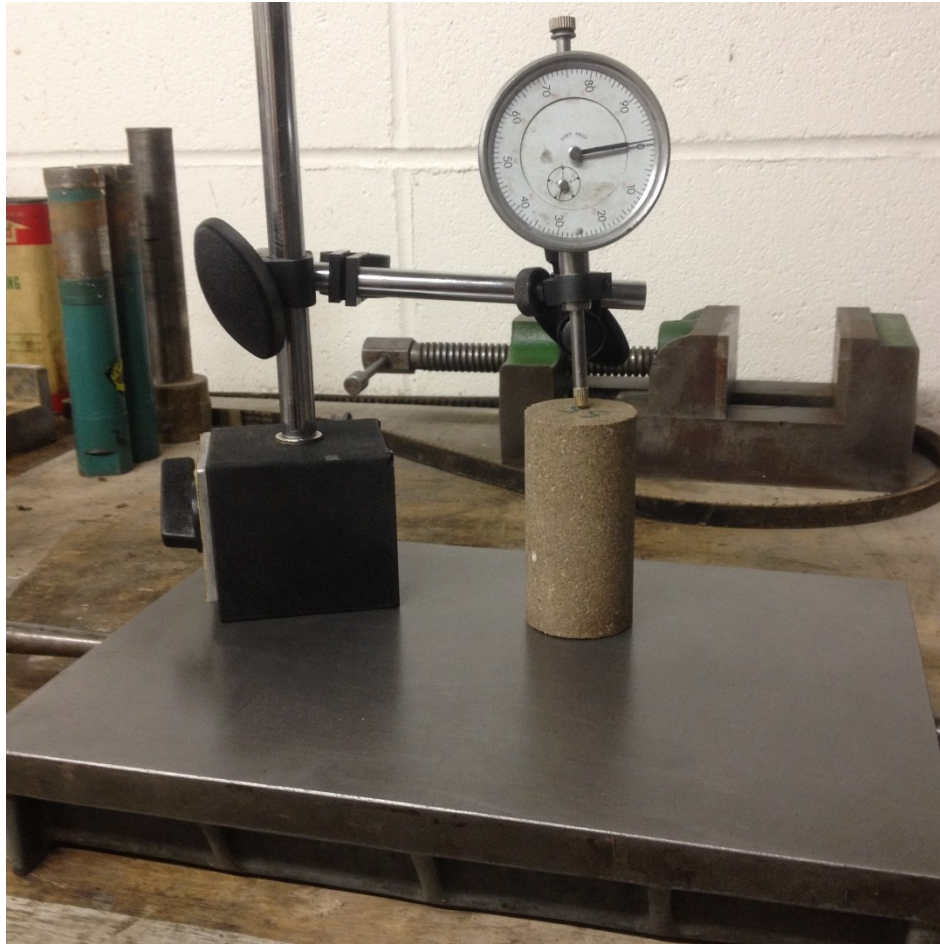
Figure 4.5 Photo of the apparatus used for determining the flatness of the cylindrical end surfaces. The displacement gauge is mounted on an adjustable stand with magnetic base. The base sits on top of the flat steel support surface.
