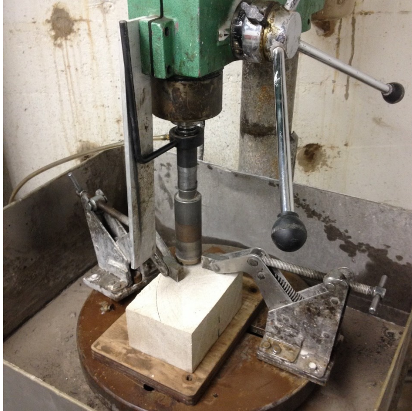
Figure 4.3 Photo of the drill press and example of a thin walled drill bit used to cut core samples. Water is pumped through a water swivel adapter, to cool the diamond core barrel and wash cuttings away from the rock surface. The rock blocks are clamped securely to a ½" thick piece of plywood on the drill table to prevent unwanted motion.
