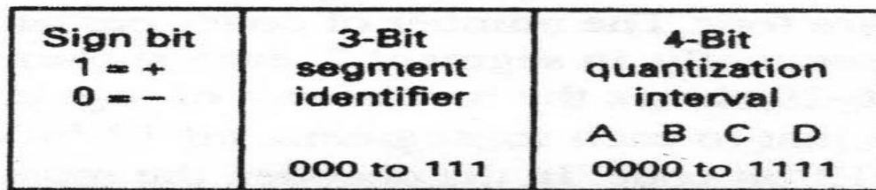
Fig 7.2: 8-bit compressed \mu 255 code format
