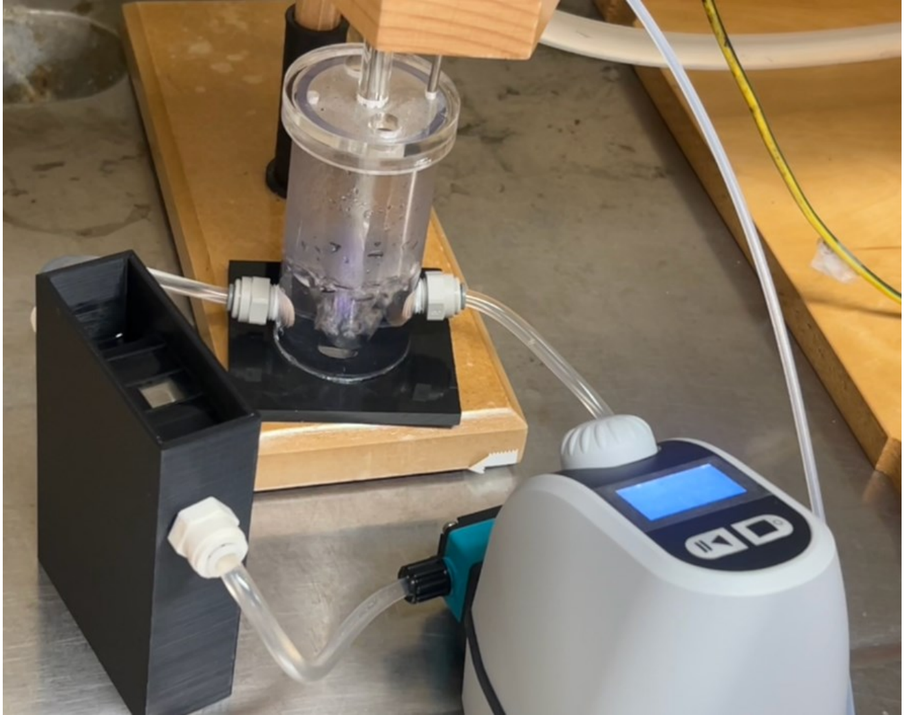
Figure A3: Setup depicting the continuous generation and circulation of PAWB on the inoculated stainless steel coupons.
