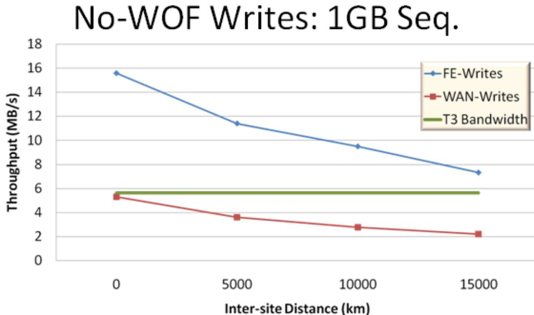
In the above graph, the RTT latency is varying among 0, 50, 100 and 150 ms which correspond to the following distance between sites respectively 0, 5000, 10000 and 15000 km. The green line represents to bandwidth of the T3 link used (around 45 Mbps which is equivalent to 5.625 MB/s) and FE-Writes means front-end writes.
