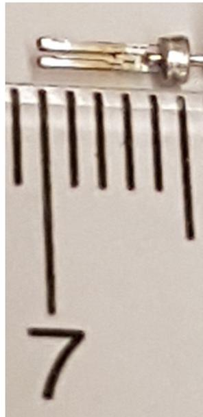
Figure 3.1. Typical 40 kHz QTF as used in this study.
