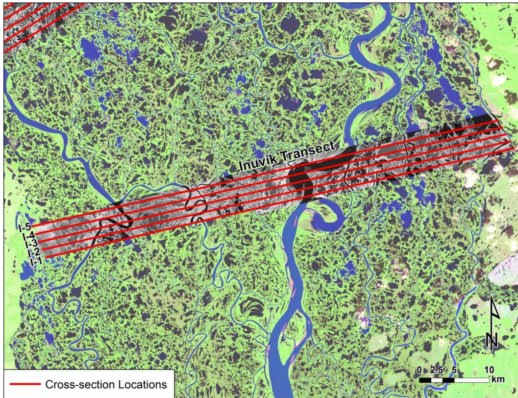
Figure 4.6 The cross-sections used to analyse the LiDAR data in the Inuvik Transect.
