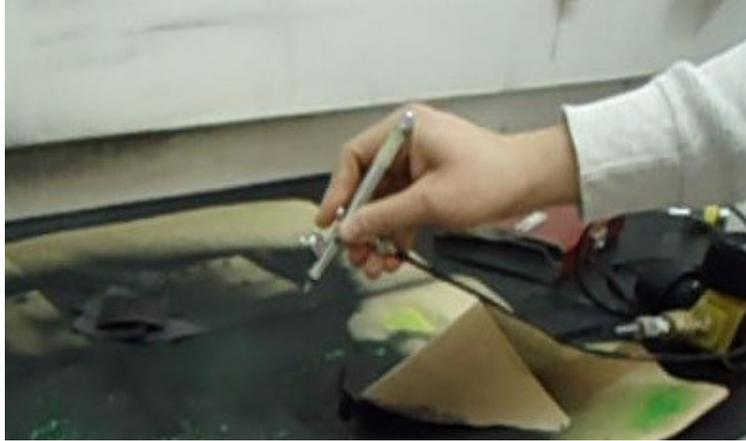
**Figure 6-4 : Using air brush technique to seed the rubber sample surface**
