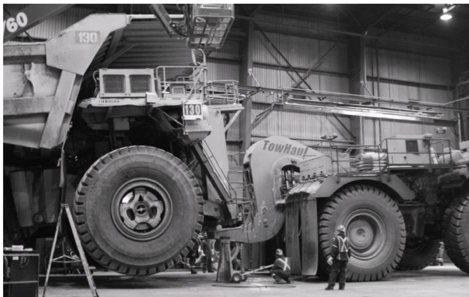
**Figure 1-1: Photograph of inspection of a haul-truck tire in a shop
