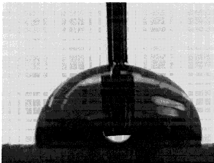
Figure A-1: Contact Angle of Water on Fluorinated Polyurethane & Silicone PC100 Coating
