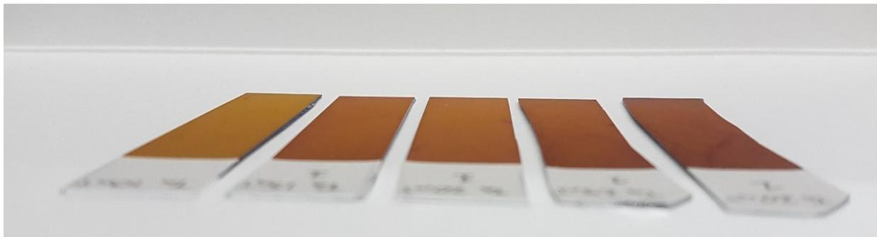
*Figure 2-9. Anodized aluminum-tantalum thin films, viewed at approximately  $75^\circ$  from normal through a polarizing lens (S-polarized light). From left-to-right tantalum sputtered at 10 mTorr, 15 mTorr, 20 mTorr, 25 mTorr and 30 mTorr.*
