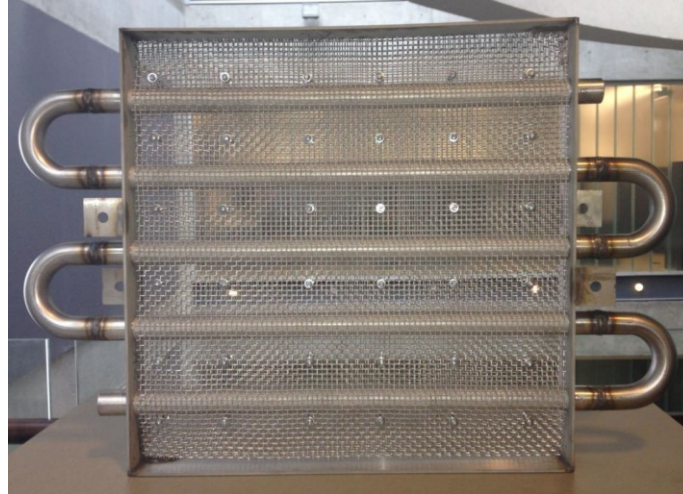
Figure 33: Wire mesh mounting prior to wire-arc coating and bonding
