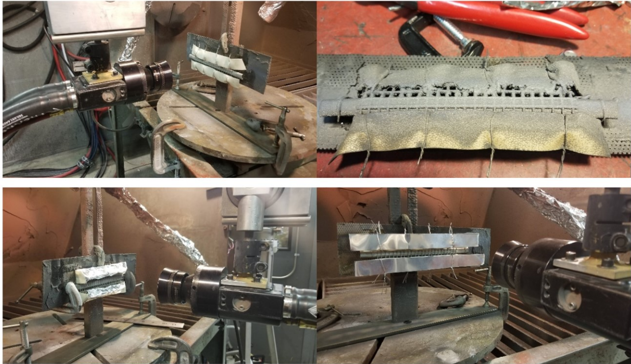
Figure 9: Various sample masking tests, heat resistant tape (Top Left), tape melted onto mesh after spraying (Top Right), Aluminum foil over tap (Bottom Left), and Aluminum sheet secured with wire (Bottom Right)
