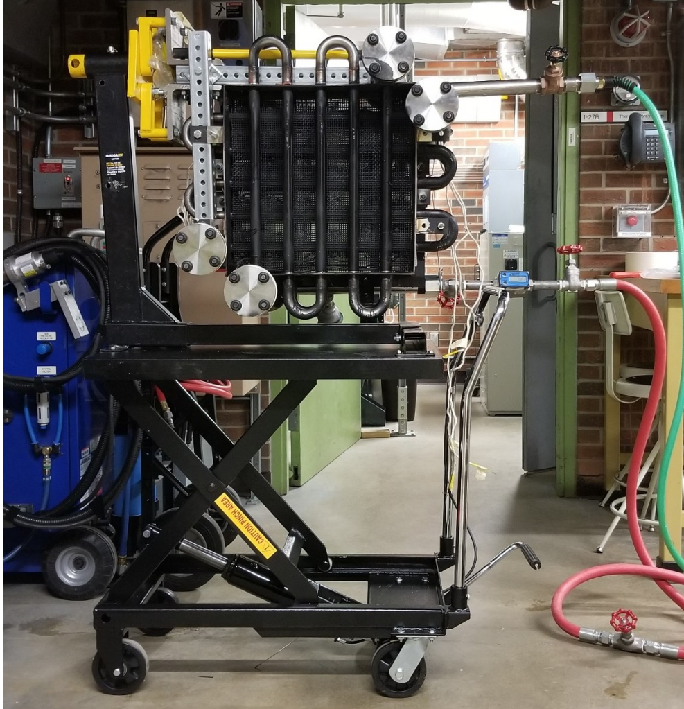
Figure 35: Final portable test cart for prototype heat exchanger
