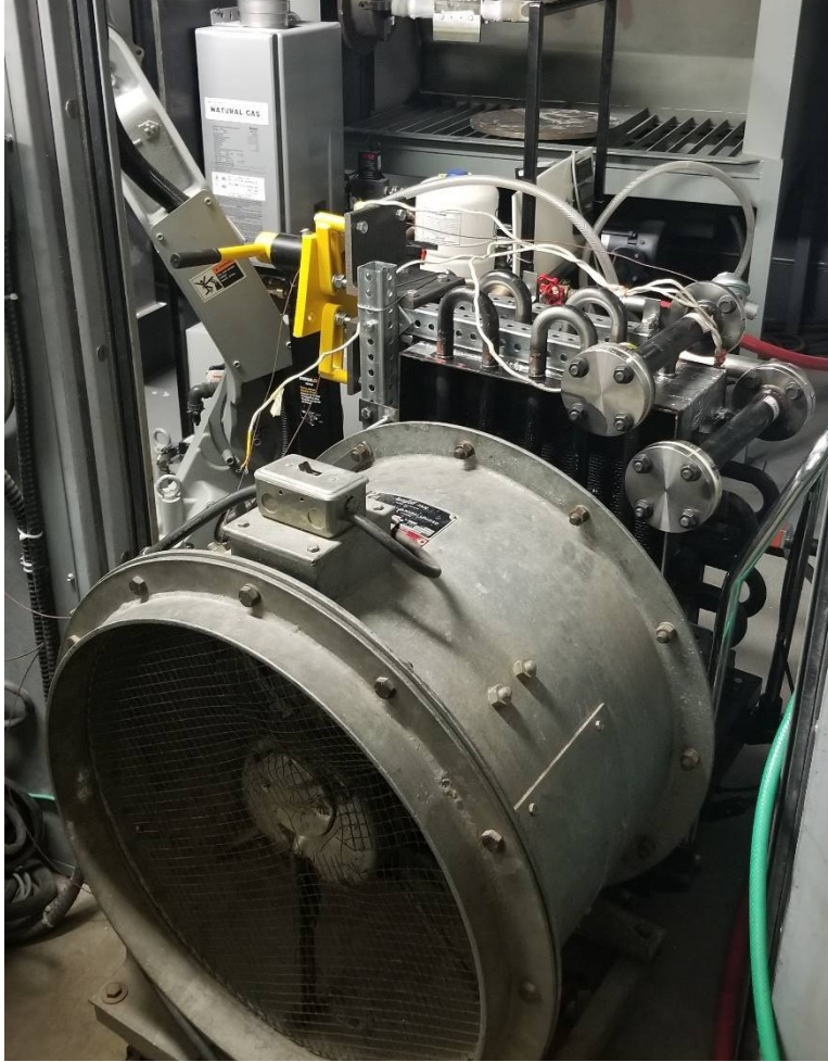
Figure 43: Large vane axial fan for air cooling tests
