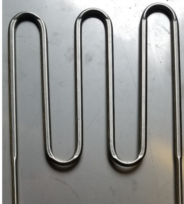
Figure 5: Bent and flattened bare tube heat exchanger
