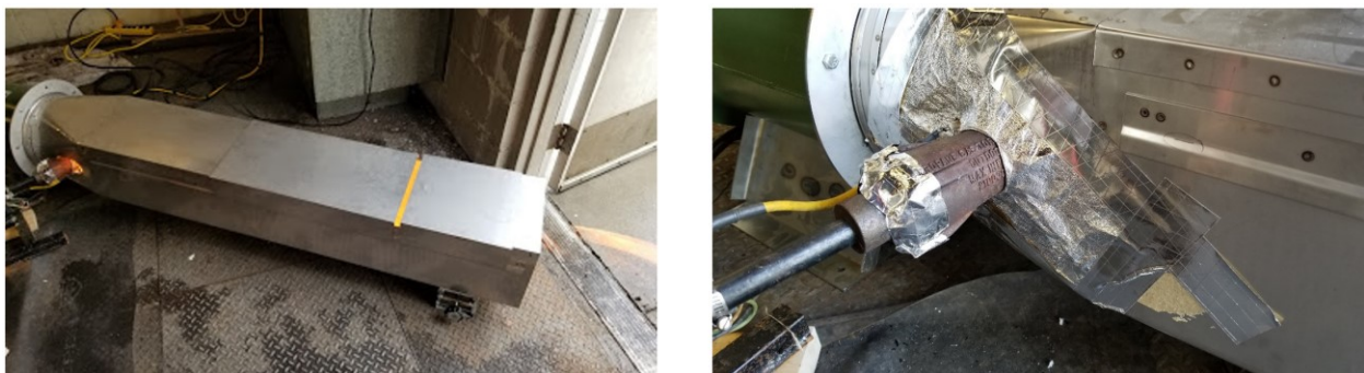
Figure 18: Propane torch flames reaching the outlet of the duct (Left), Propane torch head sealed into duct port with heat resistant foil tape (Right)
