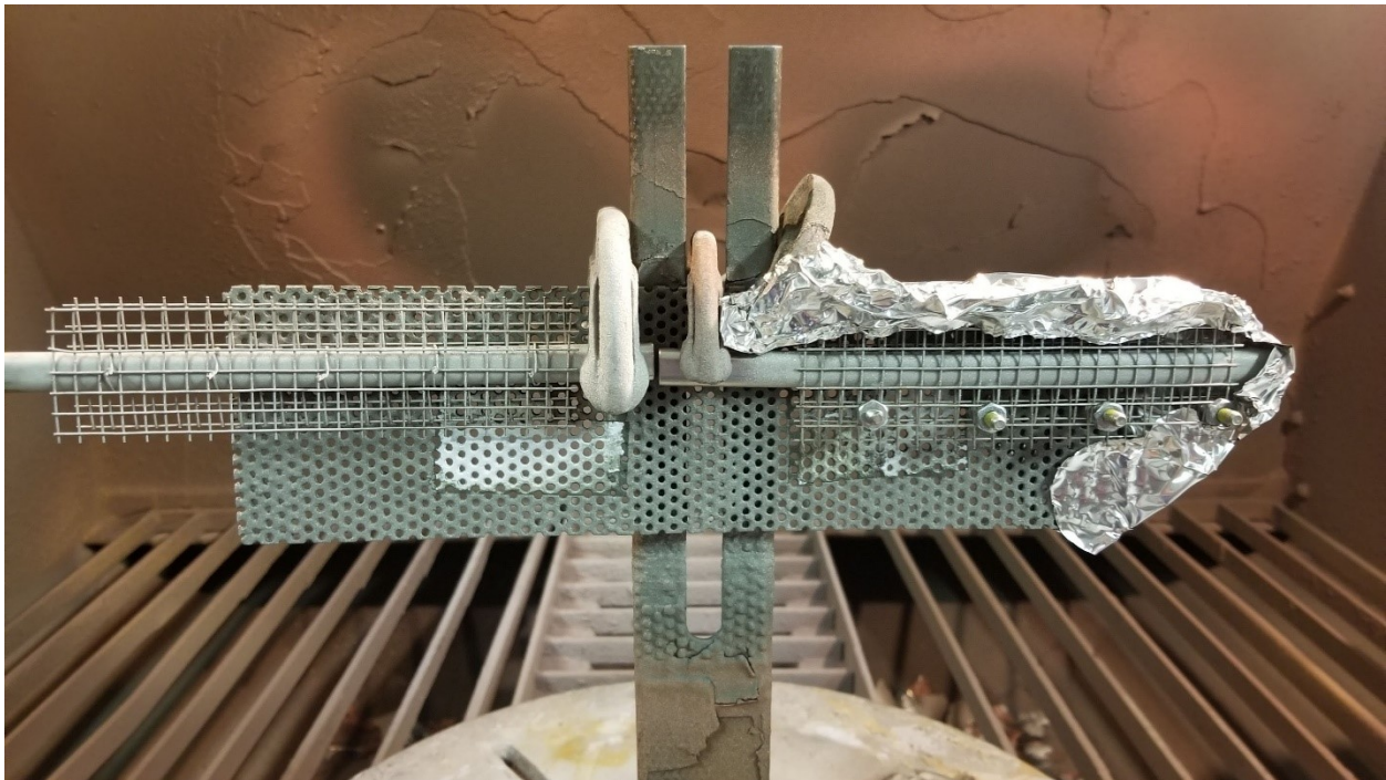
Figure 8: Two wire mesh clamping methods, wire tie method (L) compared with screw and nut method (R) with partial masking by aluminum foil to protect screw threads from coating deposition
