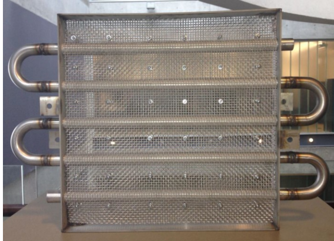
Figure 33: Wire mesh mounting prior to wire-arc coating and bonding
