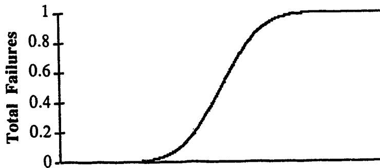
Figure 6.3 Cumulative density function, F(t) of a normal f(t) function
