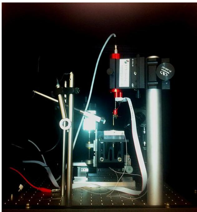
**Figure 2-3 Photo of Kelvin Probe used for SPV measurement.**
