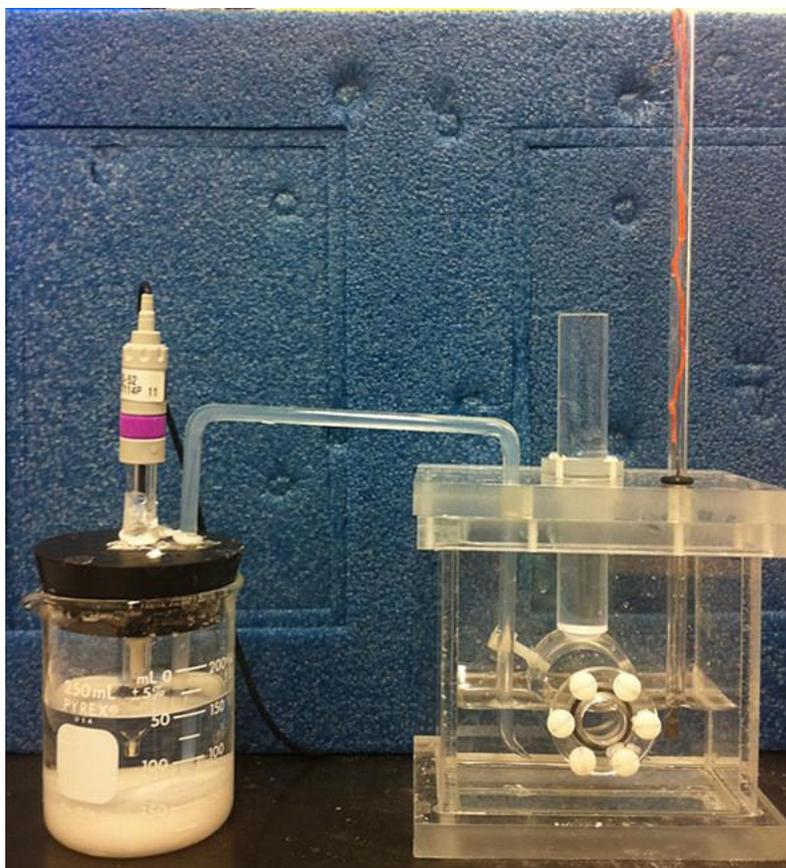
**Figure 2-2 Photo of the experimental set-up for photocurrent measurement.**
