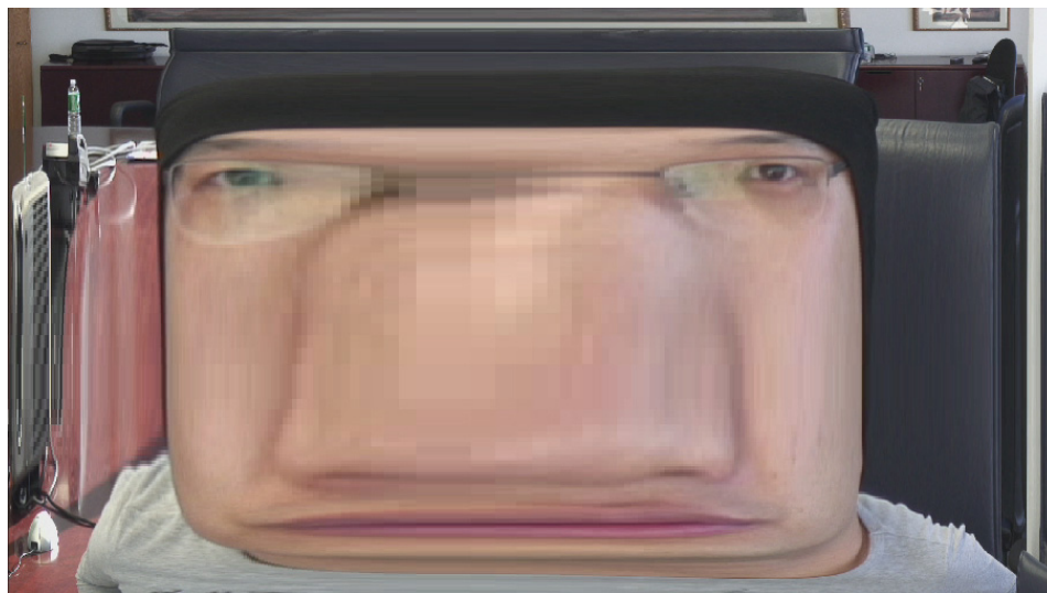
(a) Foveated 904 \times 508 image resulting from 1280 \times 720 original image, using the CVR method.
