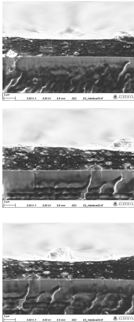
Figure 4.8: SEM images at 5000x magnification before testing of a) E2, \text{Ir}_8\text{NiO}_x 0.99 \text{ mg/cm}^2 , b) ML19, \text{IrO}_x TTK 0.993 \text{ mg/cm}^2 where the vertical direction displays the 3 cross sections used to estimate the thickness of each catalyst layer.
