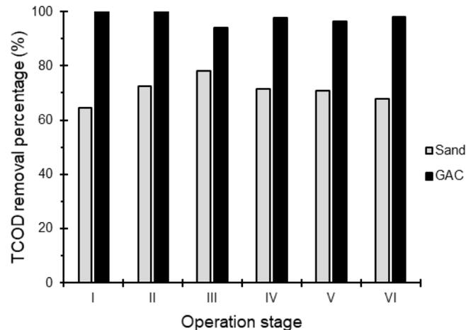
Figure 4.3. Overall TCOD removal percentage of the GAC and sand biofilters during the six operation stages.
