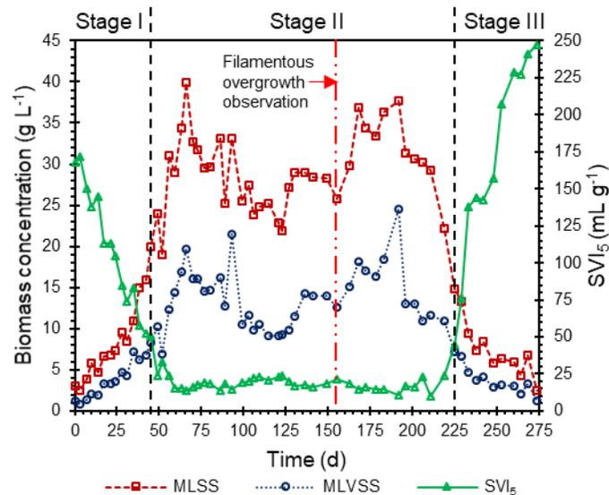
Figure 5.2. AGS settling ability and gravimetric evolution.
