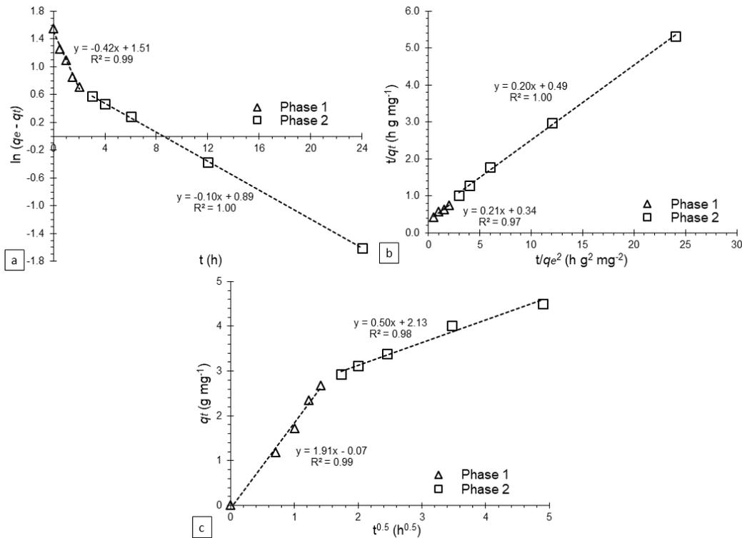
Figure 3.8. Isotherms of the adsorption kinetics of TCOD ( $\text{mg L}^{-1}$ ) on IgBGAC media in greywater constructed using linearized forms of the (a) pseudo-first
