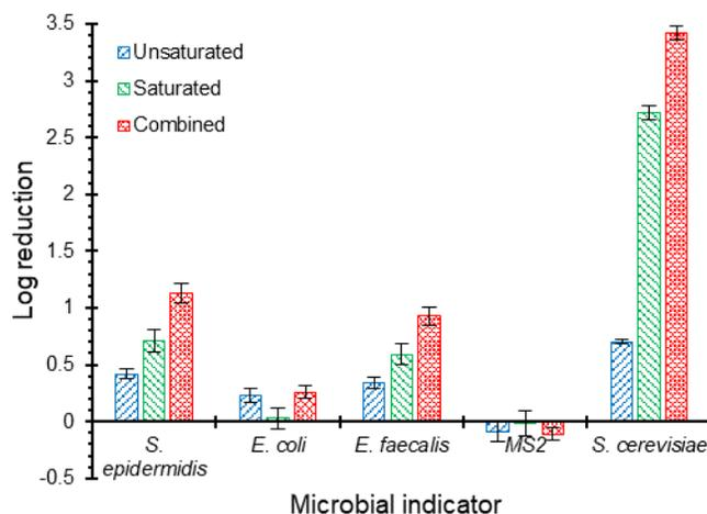
Figure 2.6. Log reductions of five pathogen surrogates: *S. epidermidis*, *E. coli*, *E. faecalis*, MS2 bacteriophage, and *S. cerevisiae* within each of the unsaturated and saturated zones individually and the entire biofilter. The columns and error bars represent the average and standard deviation values, respectively, for triplicate measurements.
