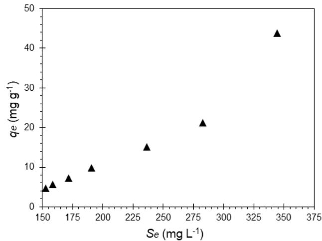
Figure 3.4. Equilibrium adsorption capacity ( $q_e$ ;  $\text{mg g}^{-1}$ ) of IgBGAC (0.1-5.0  $\text{g L}^{-1}$ ) for TCOD in greywater as a function of TCOD equilibrium concentrations ( $S_e$ ;  $\text{mg L}^{-1}$ )
