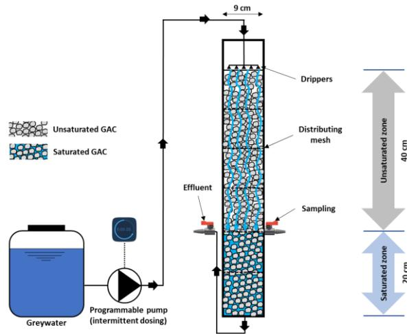
Figure 2.1. Schematic of the laboratory-scale single-stage unsaturated-saturated GAC biofilter for greywater treatment.
