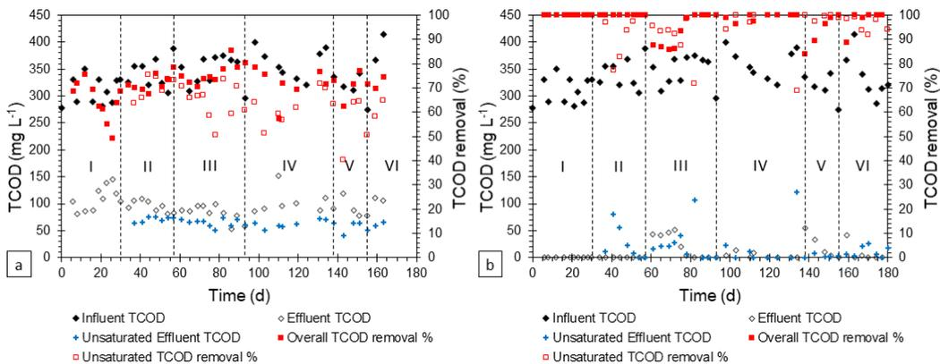
Figure 4.2. Concentration of TCOD ( $\text{mg L}^{-1}$ ) in the influent, unsaturated effluent, and overall effluent as well as the removal percentage in the two effluents as a function of the (a) sand and (b) GAC biofilters' operational time (d). The Latin numerals represent the operation stages.
