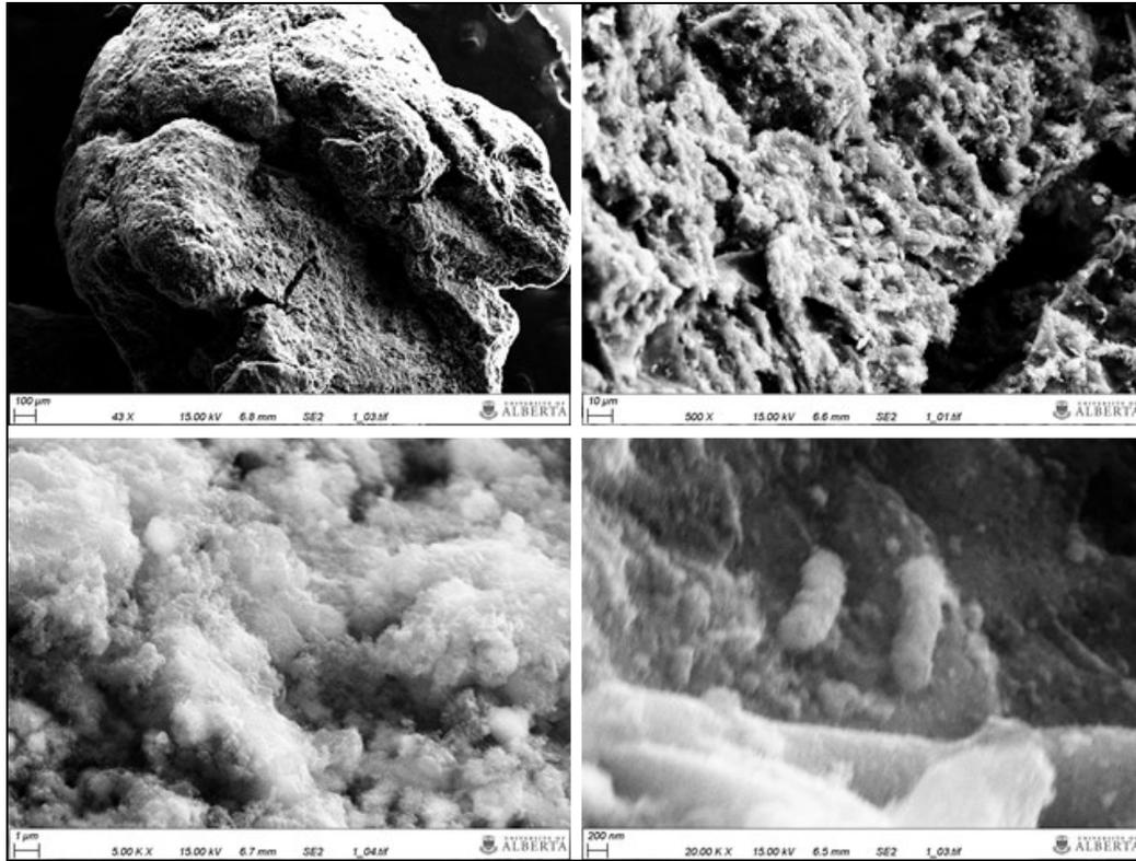
Figure 2.3. Scanning electron microscopy images of the GAC media collected from the GAC biofilter treating greywater.
