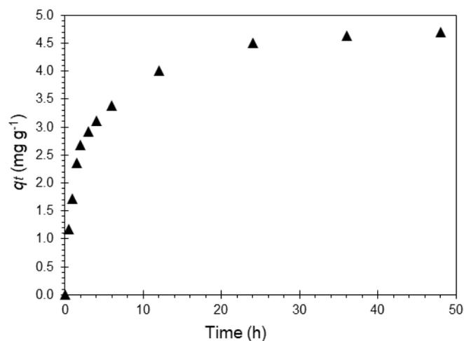
Figure 3.6. Adsorption kinetics of TCOD onto IgBGAC represented as the adsorption capacity ( $\text{mg g}^{-1}$ ) as a function of time (h).
