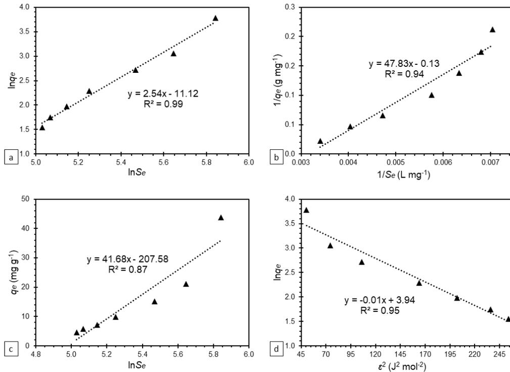
Figure 3.5. Adsorption equilibrium isotherms for TCOD ( $\text{mg L}^{-1}$ ) on IgBGAC media in greywater, described using the linearized forms of the (a) Freundlich, (b) Langmuir, (c) Temkin, and (d) D-R models. The dotted lines represent the linear trendlines of the data sets. The trendlines' formulae and their  $R^2$  values are shown.
