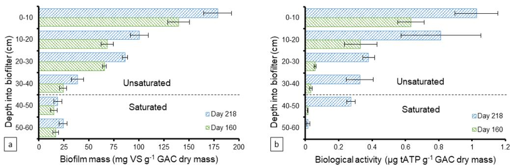
Figure 2.4. Development profile of the (a) attached biofilm mass ( $\text{mg VS g}^{-1}$  GAC) and (b) biological activity ( $\mu\text{g tATP g}^{-1}$  GAC) along the GAB biofilter depth (cm) at 10-centimeter intervals at days 160 and 218. The columns and error bars represent the average and standard deviation values, respectively, for triplicate measurements.
