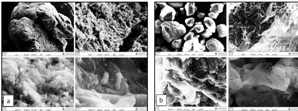
Figure 4.4. Scanning electron microscopy images of the (a) GAC and (b) sand media collected from the GAC and sand biofilters, respectively, on day 218.
