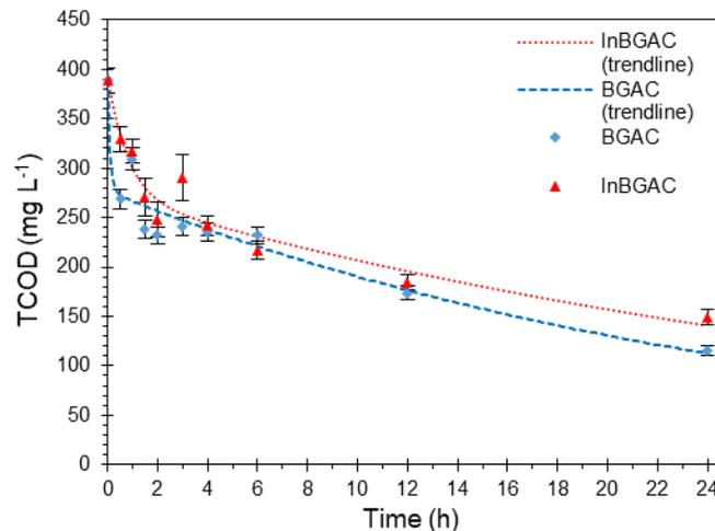
Figure 3.1. TCOD concentration ( $\text{mg L}^{-1}$ ) as a function of time (h) for BGAC and InBGAC treatment groups treating greywater. The error bars represent the standard deviation values for triplicate measurements.
