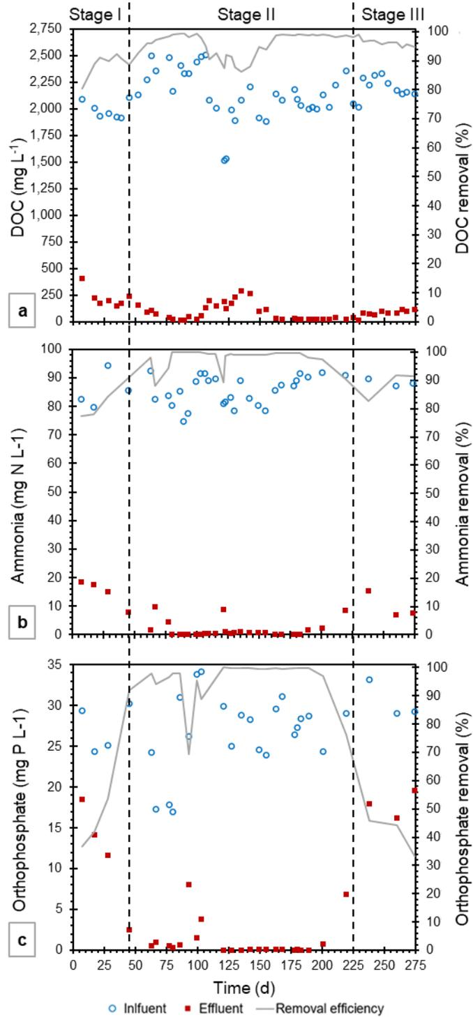
Figure 5.3. AGS reactor removal performance of (a) DOC, (b) ammonia, and (c) orthophosphate.
