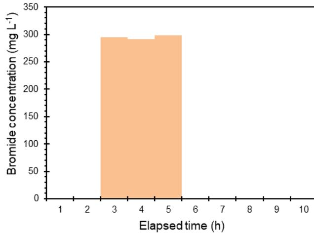
Figure 2.5. Bromide tracer test breakthrough curve.
