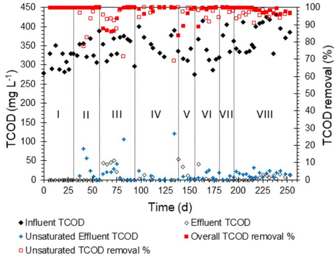
Figure 2.2. Concentration of TCOD ( $\text{mg L}^{-1}$ ) in the influent, unsaturated effluent, and overall effluent as well as the removal percentage in the two effluents as a function of the GAC biofilter's operational time (d). The Latin numerals represent the operation stages.
