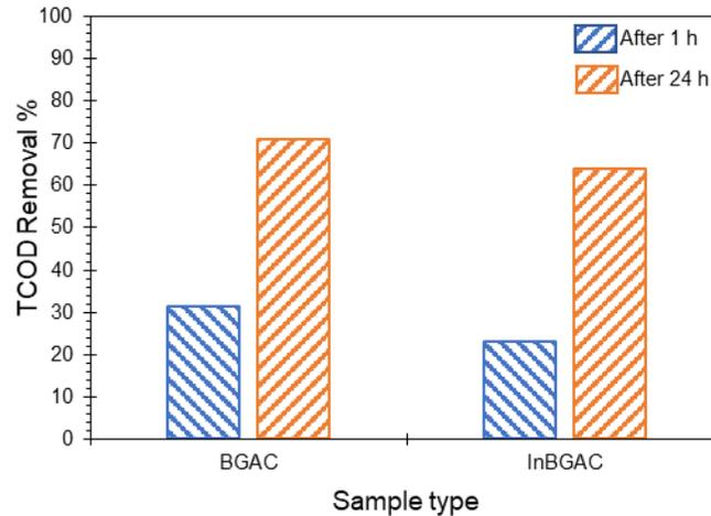
Figure 3.2. TCOD removal efficiency (%) of BGAC and InBGAC treatment groups after 1 h and after 24 h. The columns represent the average values of triplicate measurements
