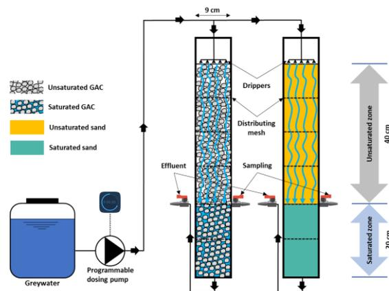
Figure 4.1. Schematic of the experimental setup of the laboratory-scale single-stage unsaturated-saturated GAC and sand biofilters treating greywater.
