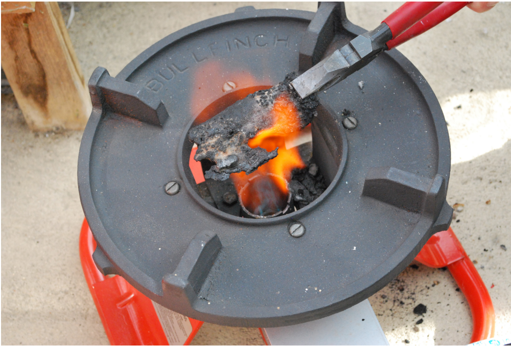
Figure 2. Bringing the iron strip to a glow.
