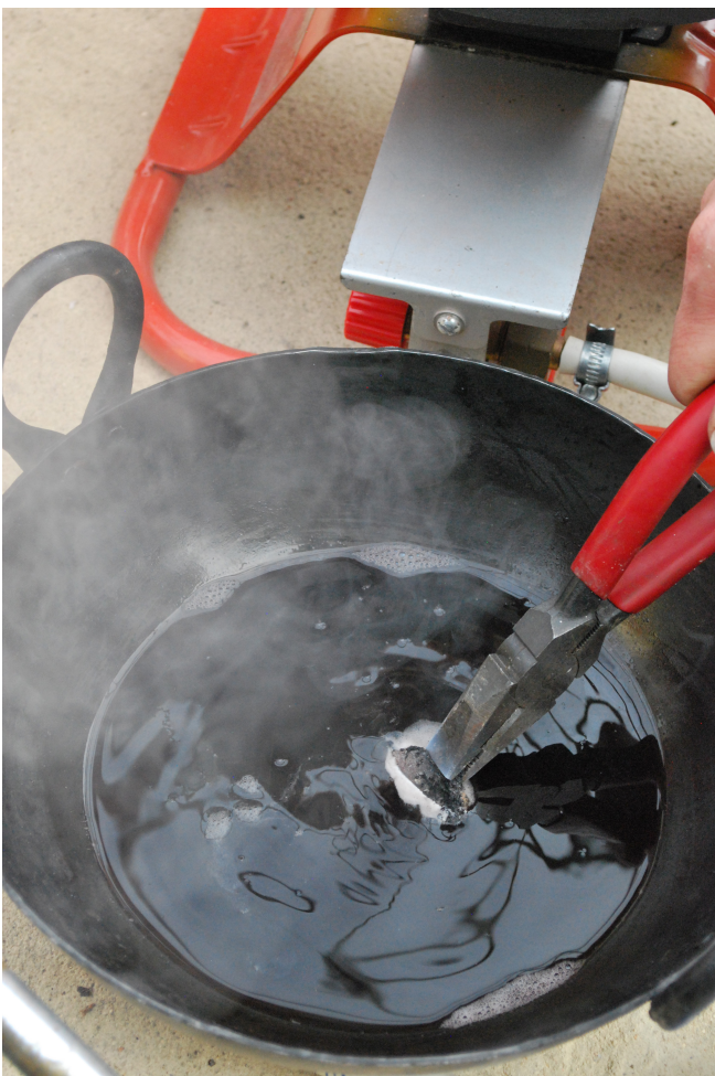
Figure 3. Quenching the iron in cow's urine and triphalā decoction.
