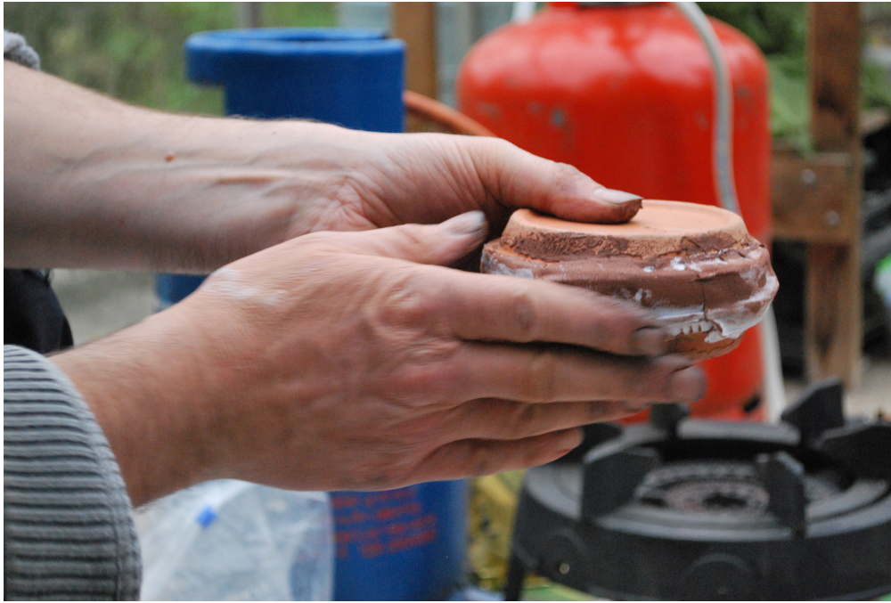
Figure 5. Sealing the clay plates. (Ayuryog, 2015)
