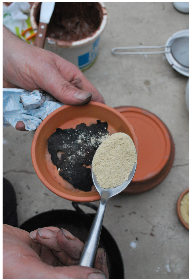
Figure 4. Placing iron and sulfur on a clay plate.
