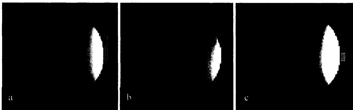
Figure 2.11 Cylindrical phantom test of the four coil phased array with the 4.7 T magnet. A pair of coils (#1 and #2) was placed on the right side of the phantom and set to receive, with the second pair of coils (#3 and #4) turned off and placed on the other side in order to demonstrate the effect of coupling interactions. (a) Coil #1 is set to receive alone. The grey rectangle represents the coil. (b) Surface coil #2 is set to receive alone. Coils #3 and #4, located on the left side, transmit some signal and noise to coil #2 through a mutual coupling interaction. This does not happen with the commercial coils 20 that were used for the images in later chapters. (c) Coils #1 and #2 are tested in combination, with the light gray area indicating coil overlap. Notice the SNR improvement due to the combination.
