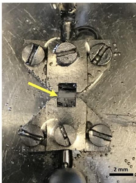
**Figure 3.1** A third-order mesenteric artery mounted in a Mulvany-Halpern wire myograph. The yellow arrow denotes an artery threaded with gold-plated tungsten wire; one foot is connected to an isometric force transducer.
