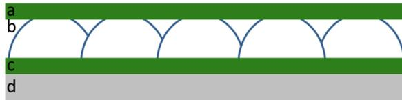
**Figure 4.1** The structure of a pNIPAm microgel based etalon, which consists of two 15-nm Au mirrors (a,c), with a 2-nm Cr adhesion layer. The mirrors sandwich a jammed layer of microgels (b) (dielectric) built on a rigid glass substrate (d).
