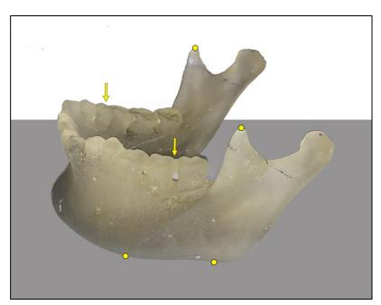
Figure 3.1: 3D-printed mandible with six radiopaque markers denoted by yellower circles and arrows
