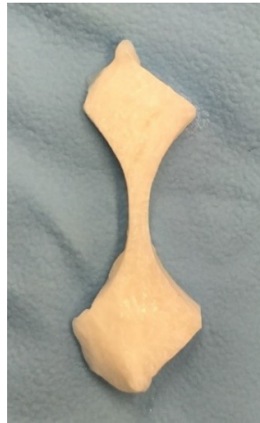
Figure 3-4: A Dumbbell-Shaped Tensile Specimen Harvested from Central Region of Each Lateral Meniscus along 4 Different Orientations
