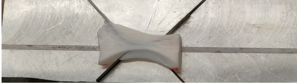
Figure 3-6: A Specimen Placed on a Specially Constructed Cutting Die
