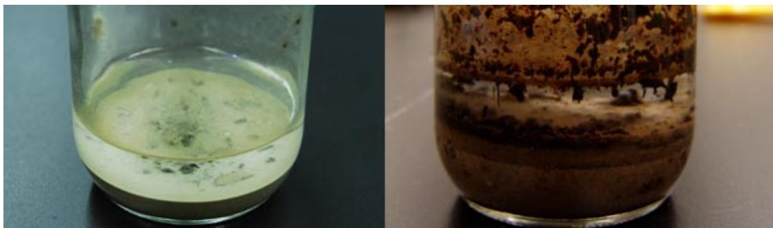
Figure 4.6: The photos of treated oil Syncrude oil slurry (left) and fresh ARC oil sand slurry (right)
