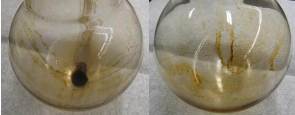
Figure 4.11: Photos of residue left in kettles (left – kettle after Dean-Stark extraction of sample treated at abc condition; right – kettle after Dean-Stark extraction of sample treated at another set of conditions)
